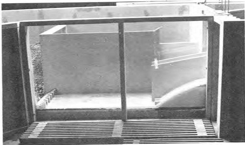
Figure 5.—Side view of hydraulic model. Yellowtail Afterbay Dam. P801-D-79762
