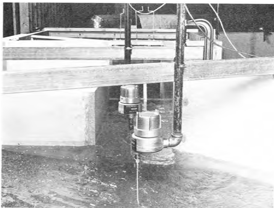
Figure 23.—Capacitance-type wave probes. P801-D-79778
