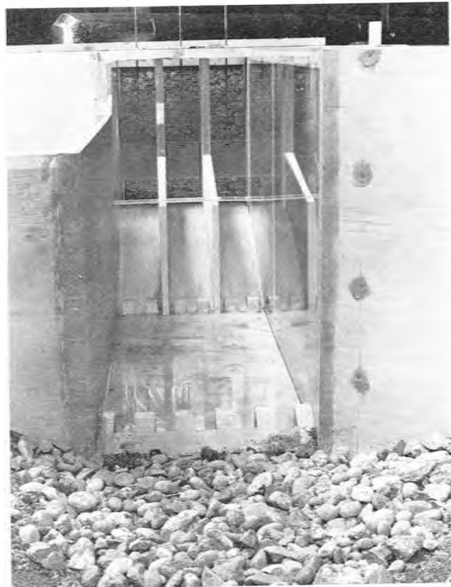
Figure 6.—Hydraulic model looking upstream into sluiceway stilling basin Yellowtail Afterbay Dam. P801-D-79763
