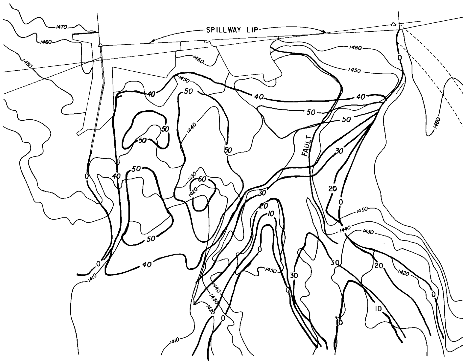
Figure A-4. Velocity contours for a discharge of 30,000 ft 3 /s (initial model topography).
