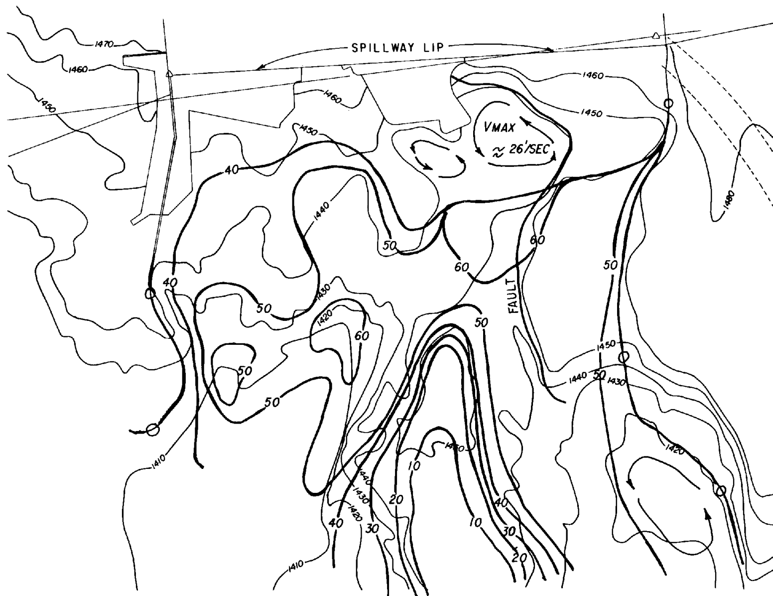
Figure A-6. Velocity contours for a discharge of 60,000 ft 3 /s (initial model topography).
