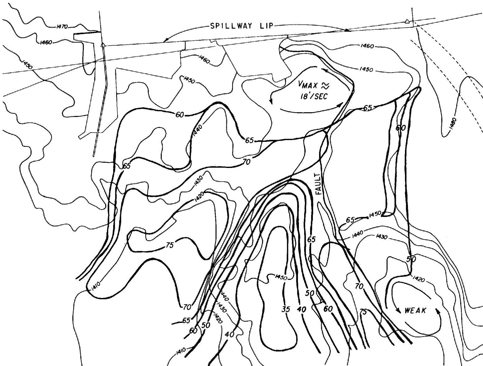
Figure A-8. Velocity contours for a discharge of 140,000 ft 3 /s (initial model topography).
