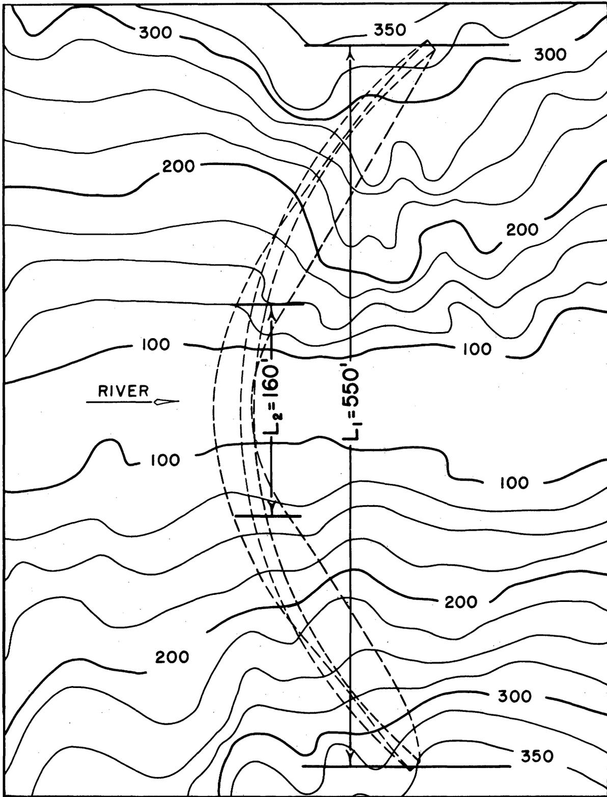
FIGURE 1.—Damsite topography and required dimensions for nomographs and layout of dam. For example 1:  $H$  = estimated structural height (290 feet);  $L_1$  = chord length, crest elevation (550 feet);  $L_2$  = chord length, 0.15 $H$  above base (160 feet); and crest assumed at elevation 325.
