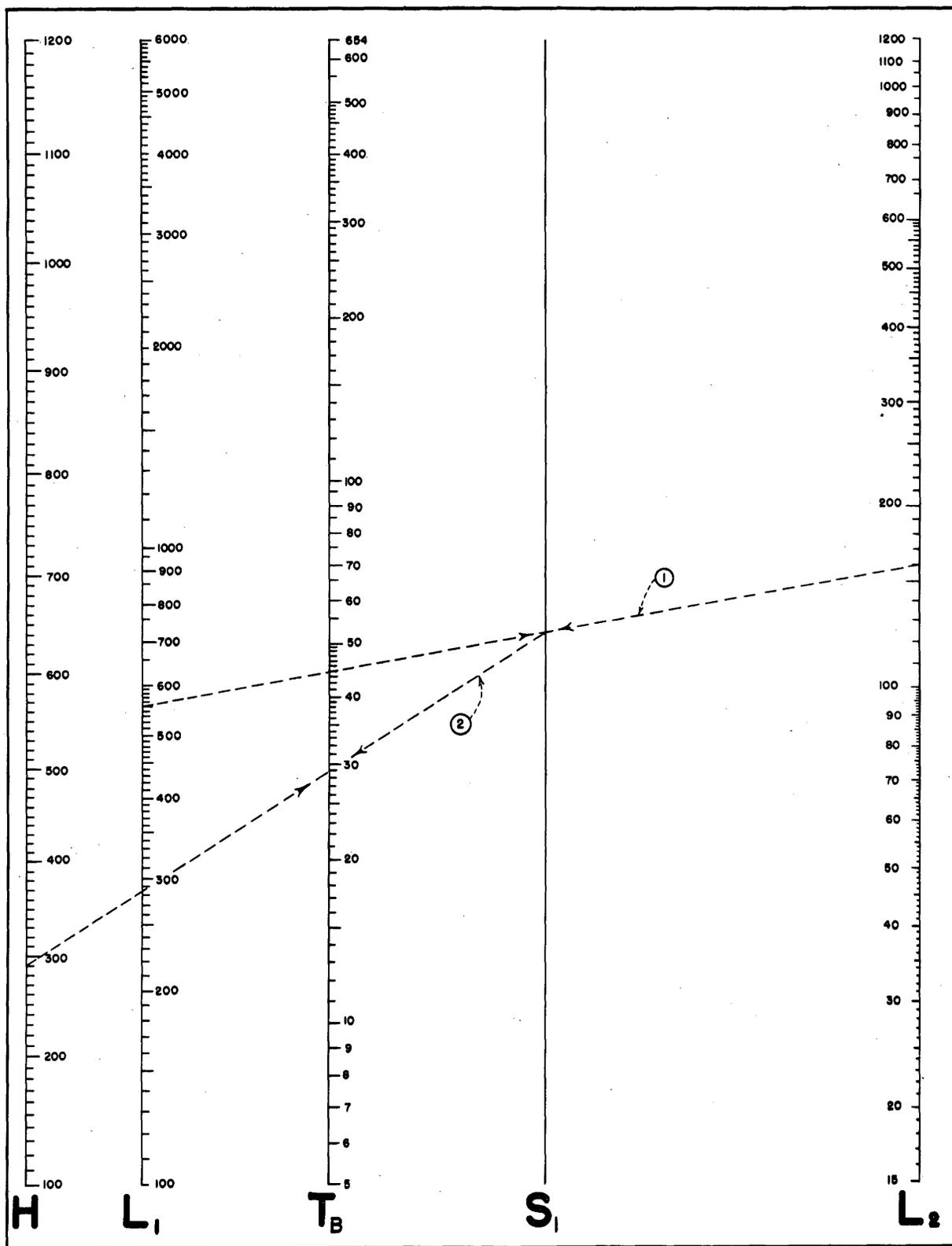
FIGURE 3.—Nomograph for obtaining base thickness and projections on crown cantilever. See notes and drawing on figure 2.
