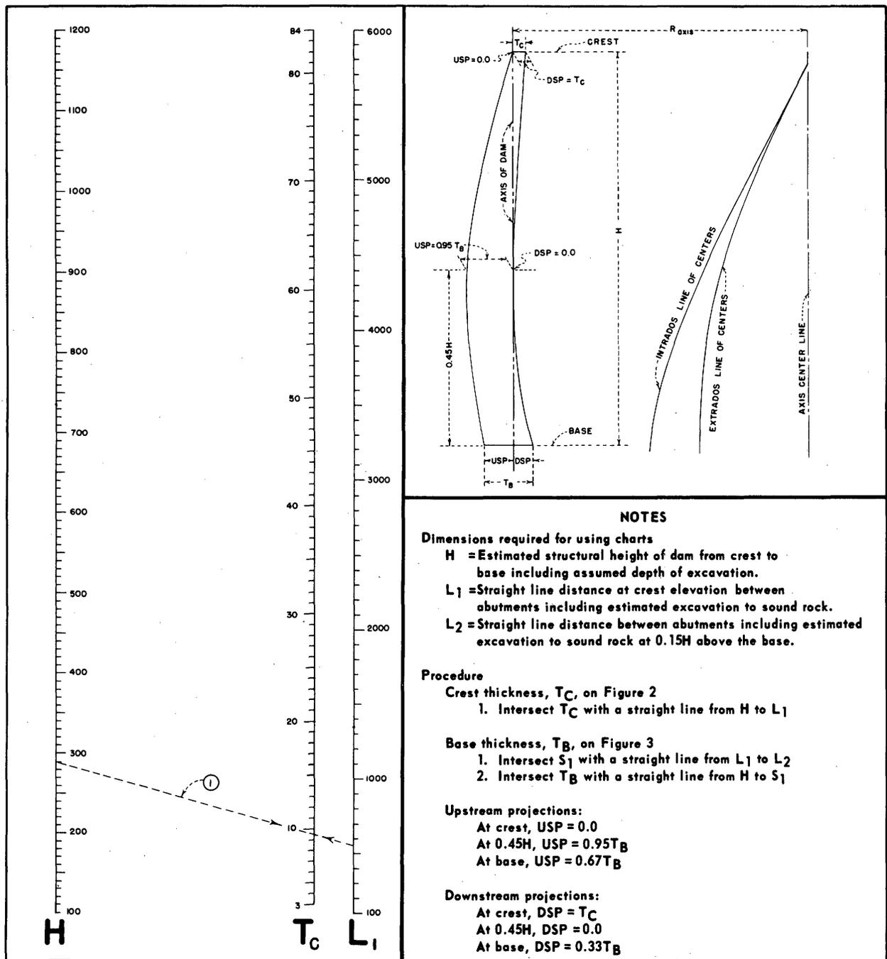
FIGURE 2.—Nomograph for obtaining crest thickness and projections on crown cantilever.
