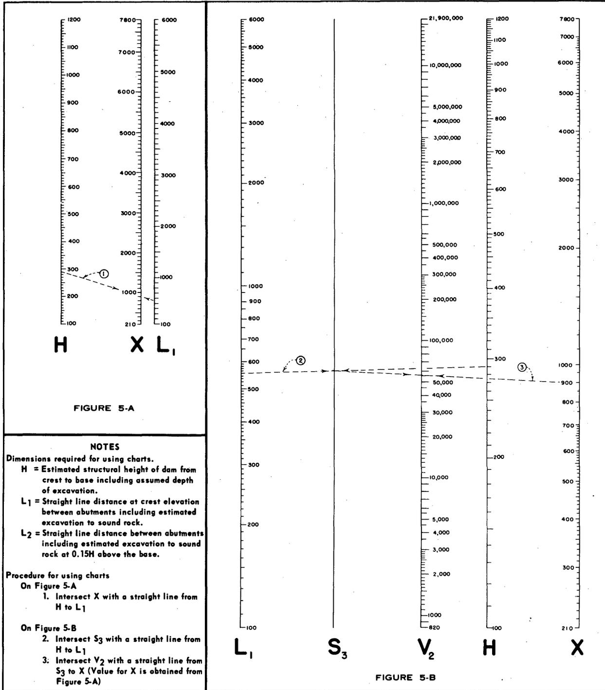
FIGURE 5.—Nomograph for obtaining  $V_2$ . ( $V = V_1 + V_2$ ).
