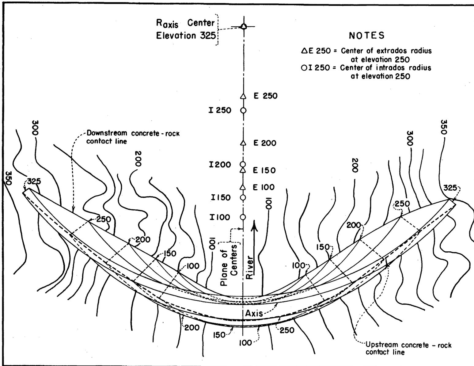
FIGURE 6.—Plan for a preliminary design.
