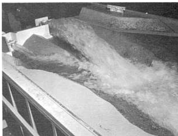
FIGURE 156.—Tube elbow bucket produces clear-cut stable jet with little spray. Discharge 28,650 c.f.s. maximum.
