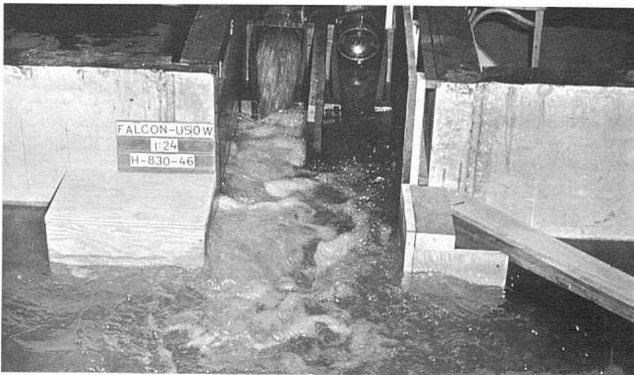
72-inch right valve fully open, discharging 1,600 c.f.s. Reservoir elevation 310, approx. Tail water elevation 180.5. FIGURE 98.—Falcon Dam: United States outlet works—model scale: 1:24.
