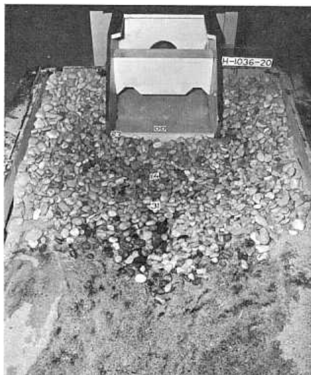
FIGURE 173.—Hydraulic model tests using 9- to 18-inch diameter (equivalent) stones show some movement of riprap.
