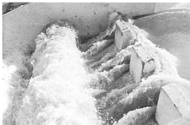
The second row of baffles is completely covered because of acceleration of flow between the first and second rows with a flow of 75 c.f.s. at top of baffled chute.
