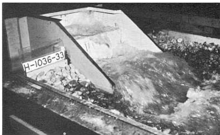
FIGURE 43.—Typical performance of impact-type energy dissipator at maximum discharges—no tail water (Basin VI).
