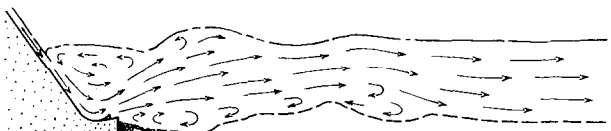
D—Tail water same as in C. Diving jet is lifted by ground roller. Scour hole backfills similar to B. Cycle repeats. (Bed level 0.3 inch below apron lip at start of test.)
