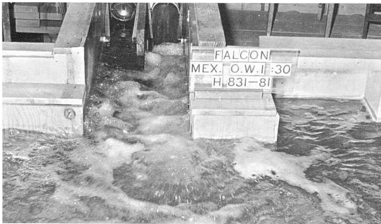
90-inch left valve fully open, discharging 2,400 c.f.s. Reservoir elevation 300, approx. Tail water elevation 181.2. FIGURE 96.—Falcon Dam: Mexican outlet works—model scale: 1:30.
