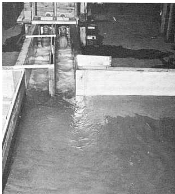
FIGURE 90.—Boysen Dam: outlet works discharging 1,320 c.f.s.—model scale: 1:16.
