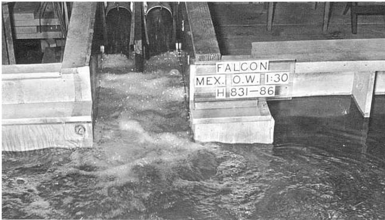
90-inch valves fully open, discharging 4,570 c.f.s. Reservoir elevation 300, approx. Tail water elevation 181.2. FIGURE 95.—Falcon Dam: Mexican outlet works—model scale: 1:30.
