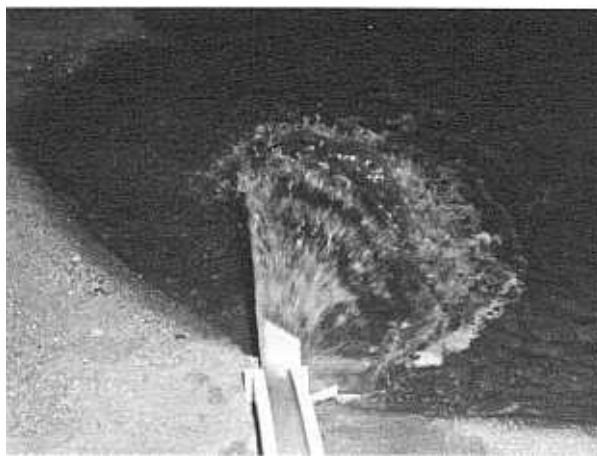
FIGURE 143. Dispersion-type flip bucket— Q=24,000 c.f.s.
