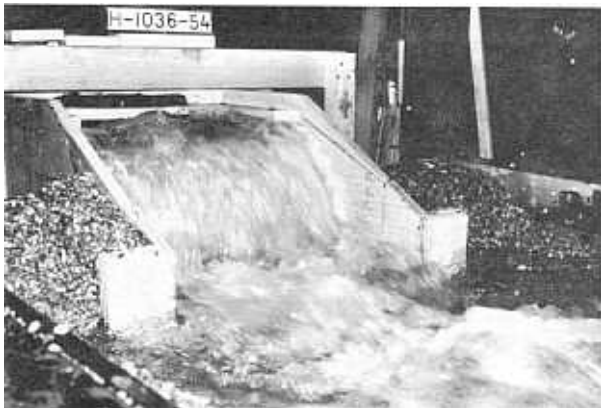
FIGURE 45. Channel erosion and emergency operation for maximum tabular discharge—impact type energy dissipator—no tail water (Basin VI).
