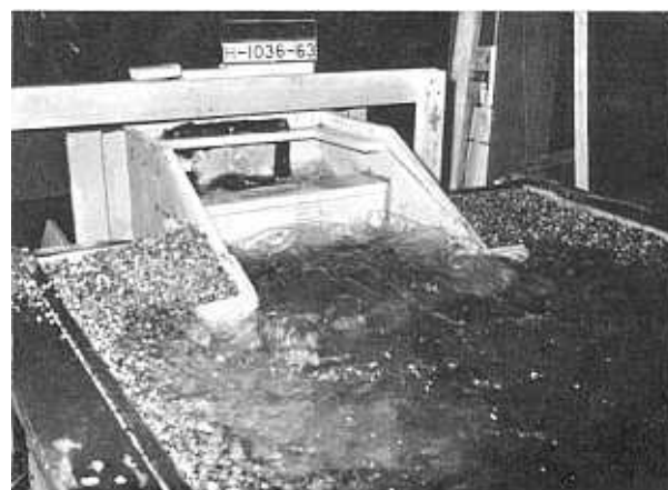
Flow appearance in model for the same conditions. Note similarity both upstream and downstream from vertical baffle.
