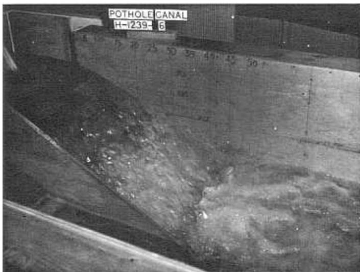
Baffle piers 4'6" high, row spacing 9'0".
