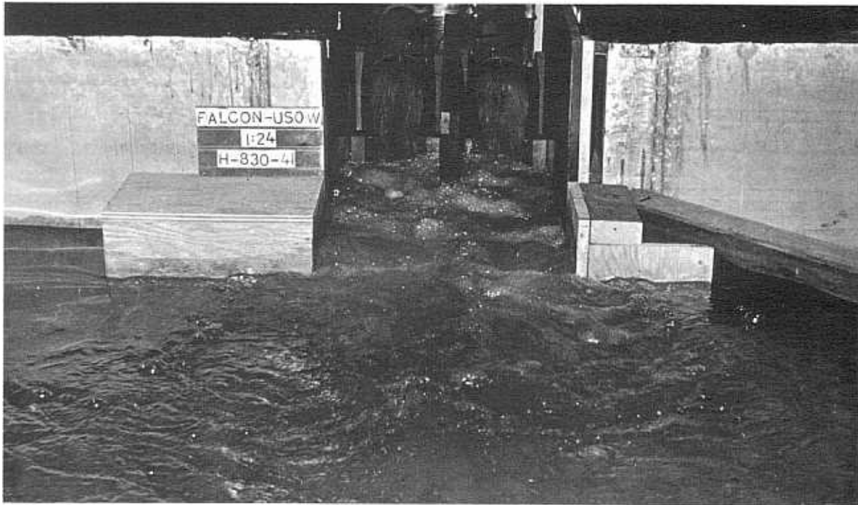
72-inch valves fully open, discharging 2,920 c.f.s. Reservoir elevation 310, approx. Tail water elevation 180.8. FIGURE 97.—Falcon Dam: United States outlet works—model scale: 1:24.
