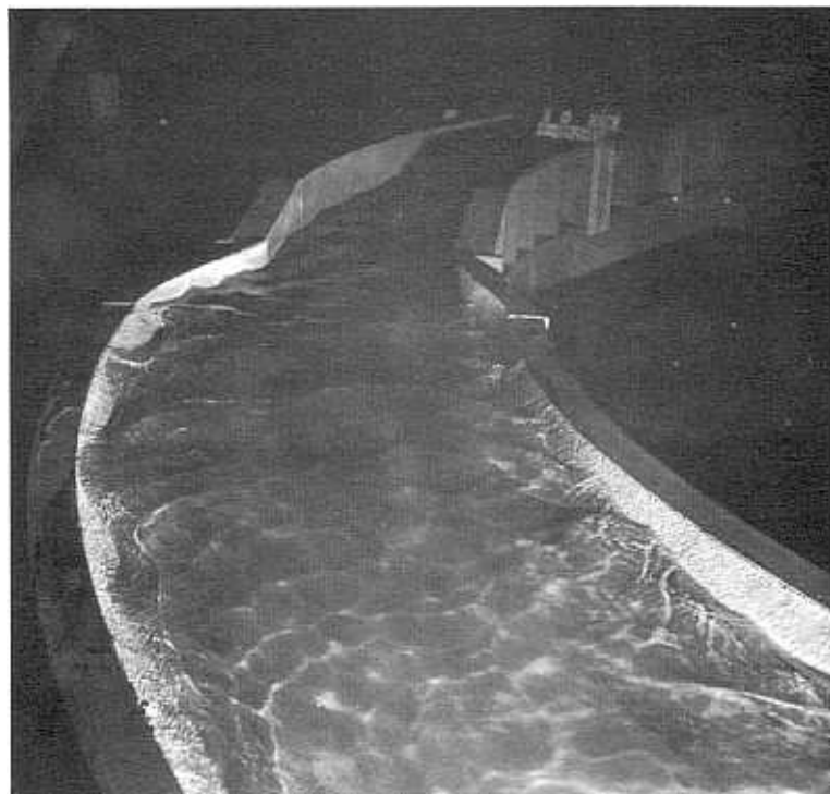
Without suppressor—waves overtop canal.
