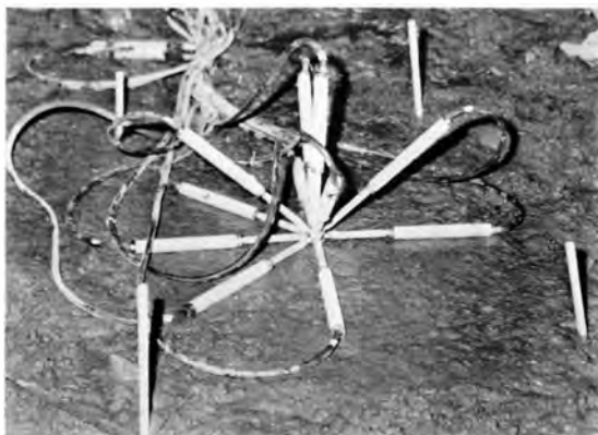
FIGURE 7 - Strain meter group showing instruments assembled to holding spider.
