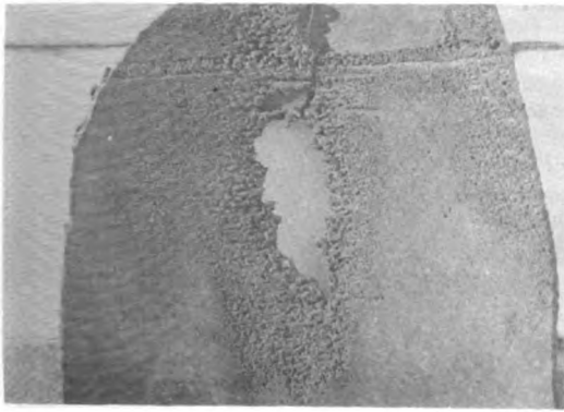
A. Pitting which has penetrated through a 5/8-inch penstock plate.
