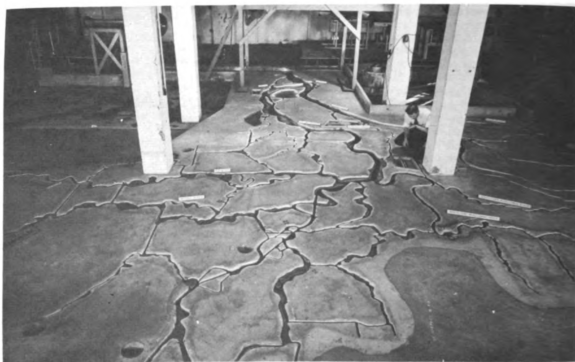
Figure 39. Distorted fixed-bed model of Sacramento and San Joaquin Rivers: horizontal scale 1:4800 and vertical scale 1:100
