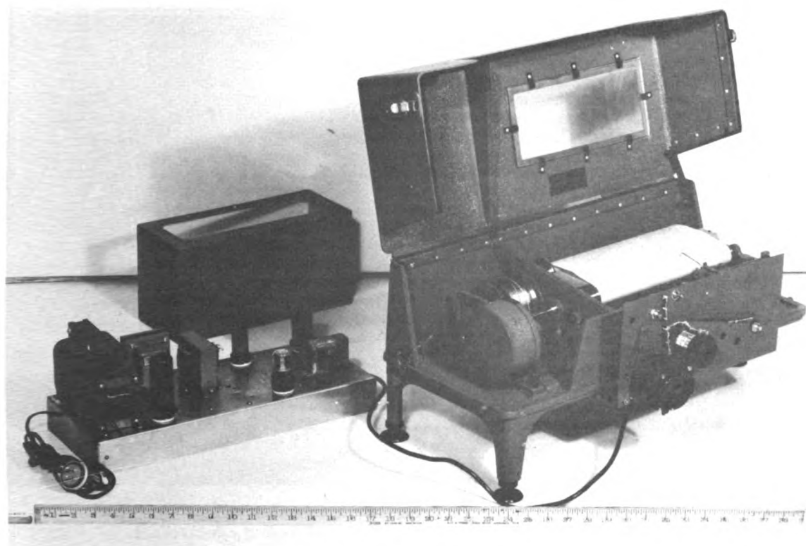
Figure 22. Instrument for continuous recording of salinity in Sacramento-San Joaquin Delta, Central Valley, California
