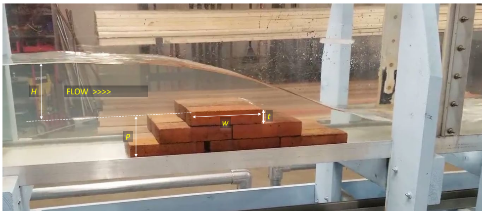
Figure 4: Initial flume testing, with illustration of key variables.
