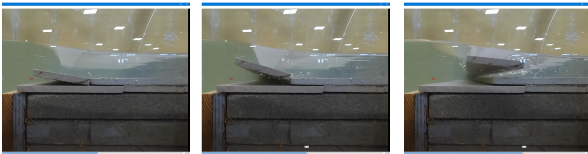
Figure 9: Failure sequence for uplift of crest cap upstream from a longitudinal crack. Flow is left to right. Elapsed time is less than 1 second. Sliding failure of the downstream piece occurred after the completion of this photo sequence (a few seconds later).
