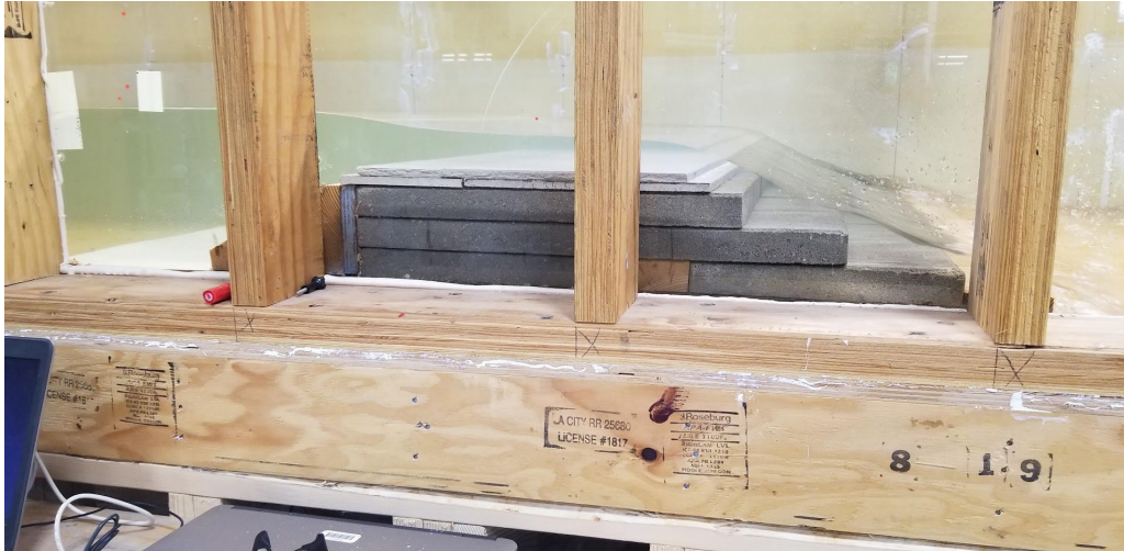
Figure 6: Overtopping testing conducted in wide flume with minimal tailwater.
