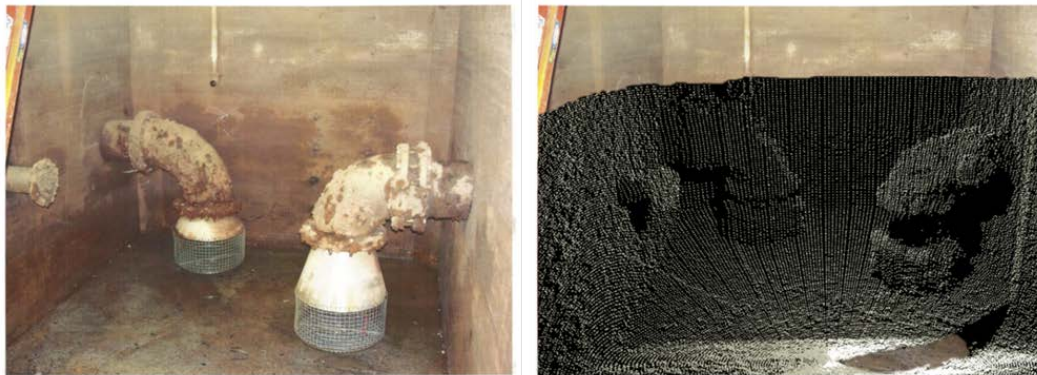
Figure 3.—Left – Photograph of a pump sump in Reclamation's hydraulics lab in Denver, Colorado. Right – 3-D point cloud of the water-filled sump (over 100,000 profile points) overlaid on the photograph.
