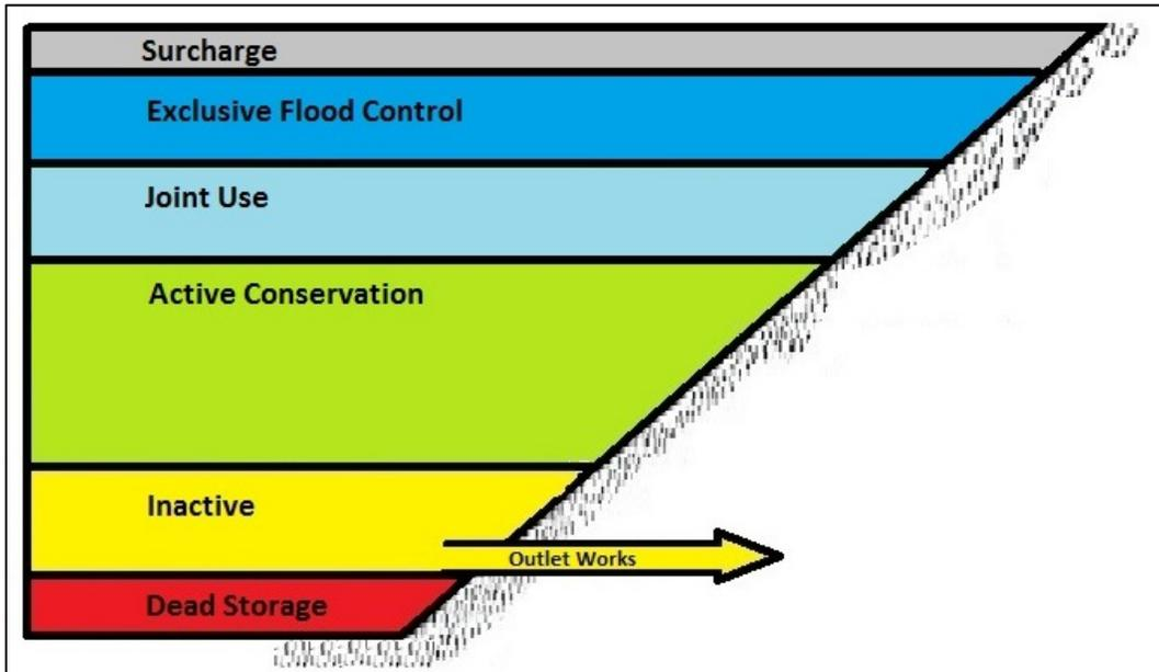
Figure 7.2.2-3. Typical reservoir storage allocation within Reclamation’s reservoirs.
