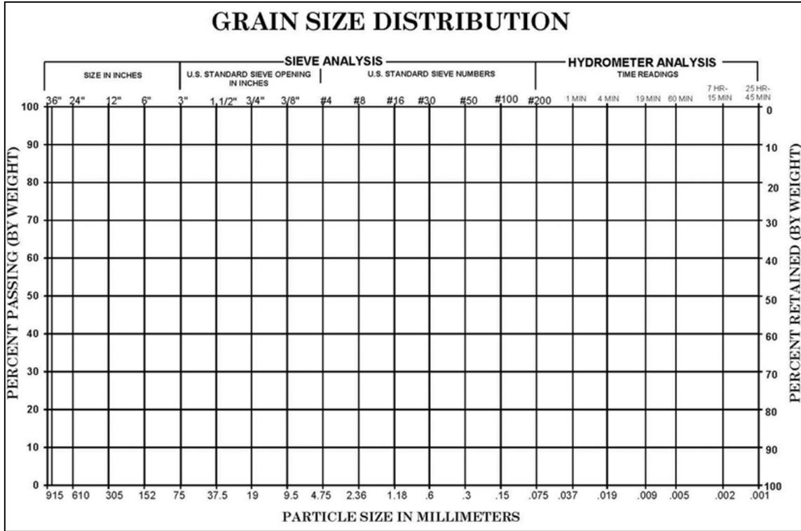
Figure 7.3.7-1. Blank gradation chart (by particle diameter) for riprap and bedding material design.
