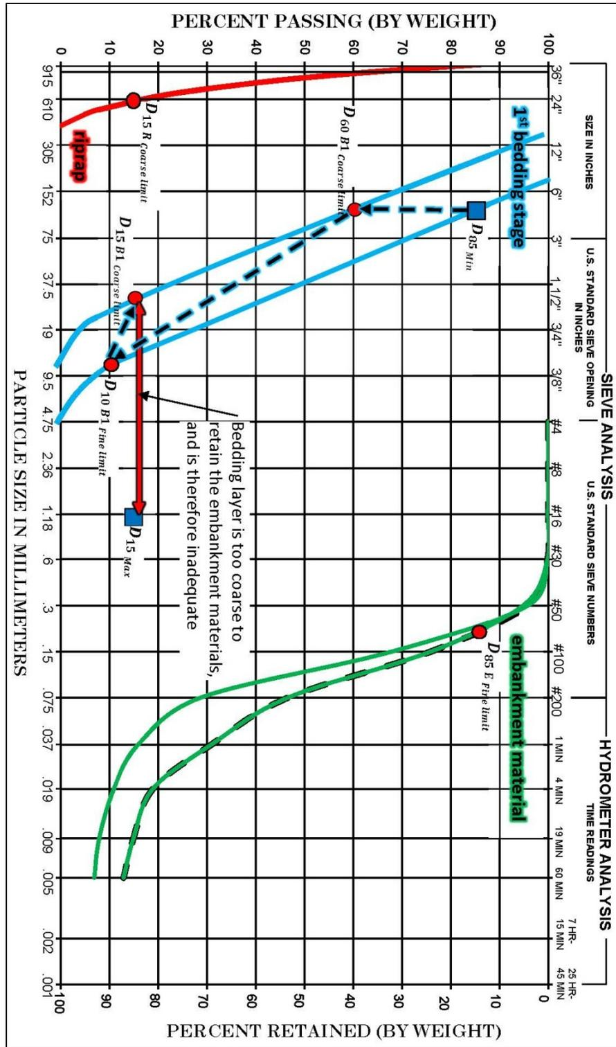
Figure 7.3.7.5-3. First bedding layer is inadequate because  $D_{15 B1 Coarse-limit}$  is greater than  $D_{15 Max}$ . The blue dashed arrows indicate the order in which the points are calculated when constructing the bedding gradation band (section 7.3.7.4).
