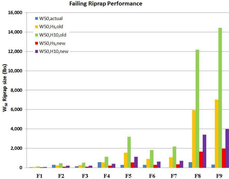
Figure D.1.  $W_{50}$  sizes of riprap “failures” due to erosion.
