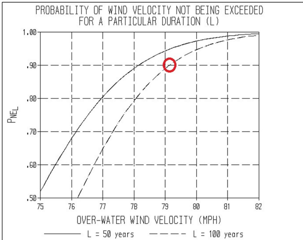
**Figure C.3. Design wind velocity versus probability of nonexceedence chart for Dam A.**
