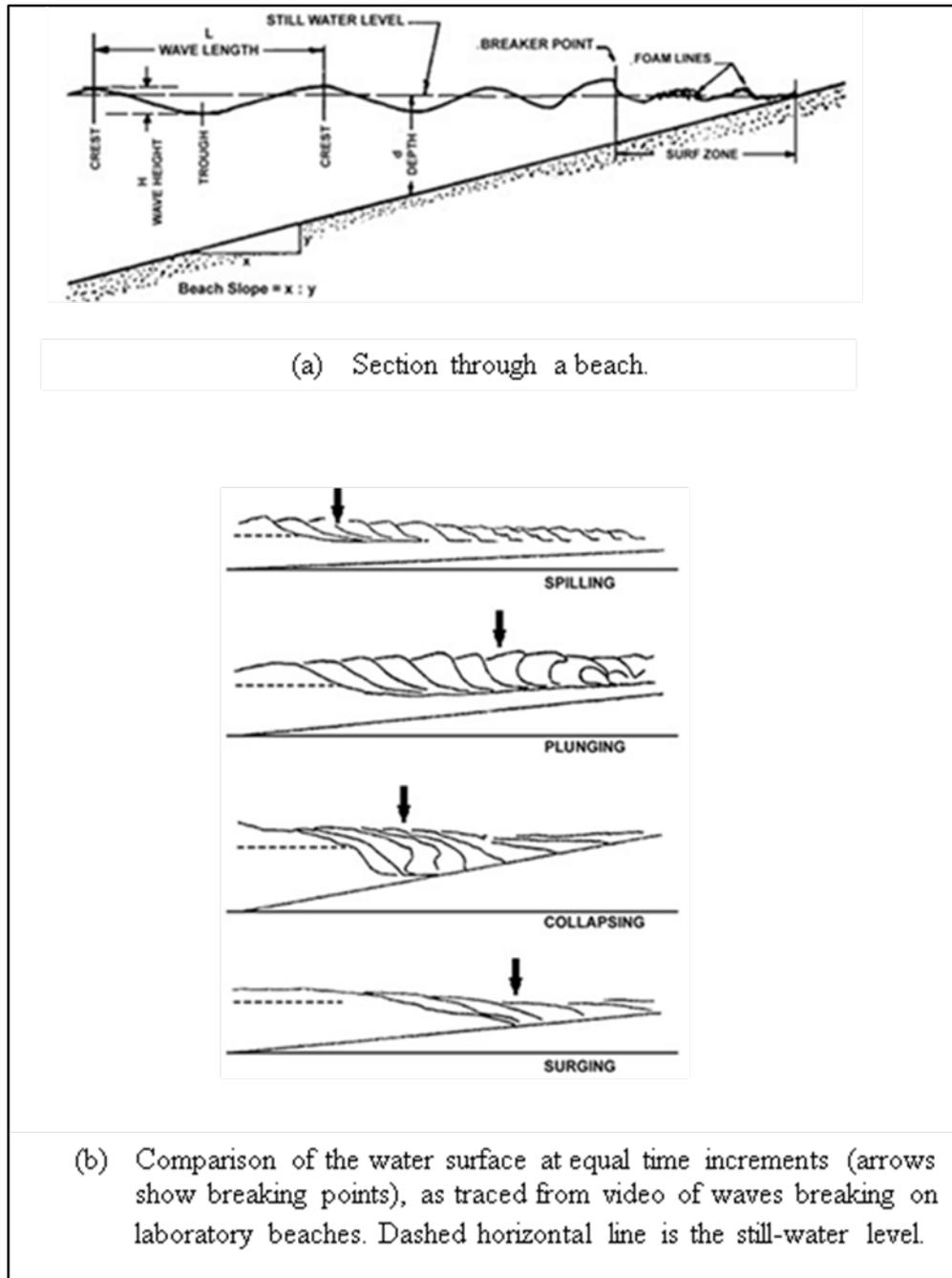
Figure 7.2.2-1. Wave breaker types.
