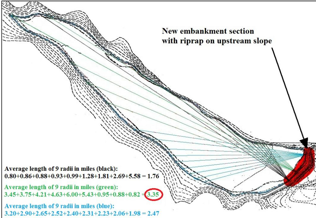
Figure C.1. Fetch calculation at Dam A using the method described in section 7.3.2.
