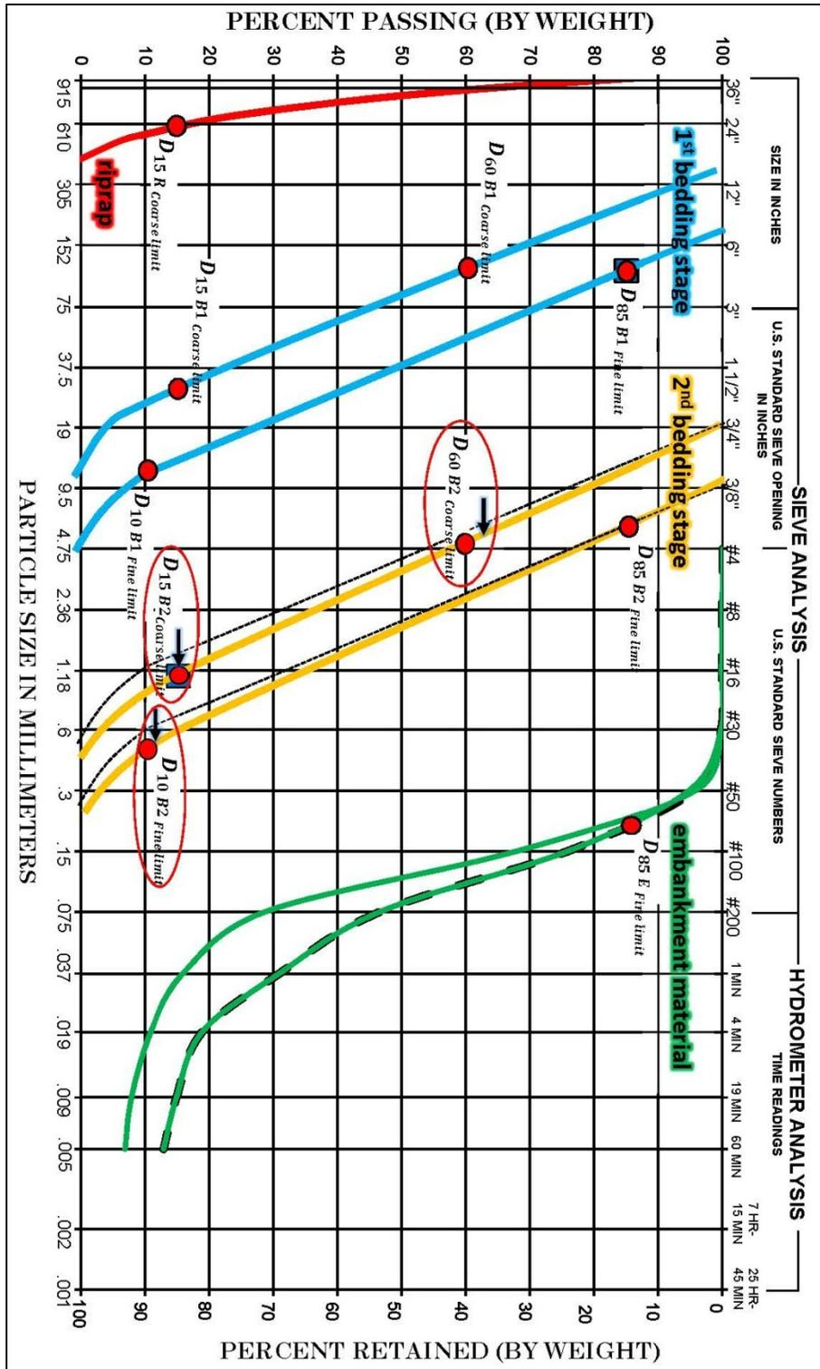
Figure 7.3.7.5-5. Modified second bedding layer. Circled points were translated right to meet  $D_{15max}$  criteria, resulting in a more broadly graded (flatter) gradation. Coarse- and fine-limit curves were moved closer together to meet stability criteria ( $C_u > 10$ ).
