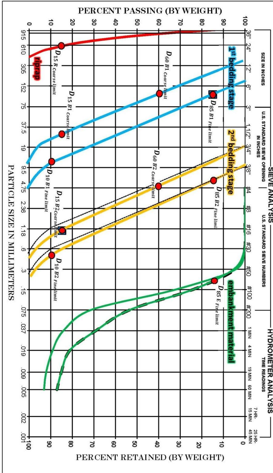
Figure C.7. Final gradation curves for first (blue) and second (orange) bedding stages.
