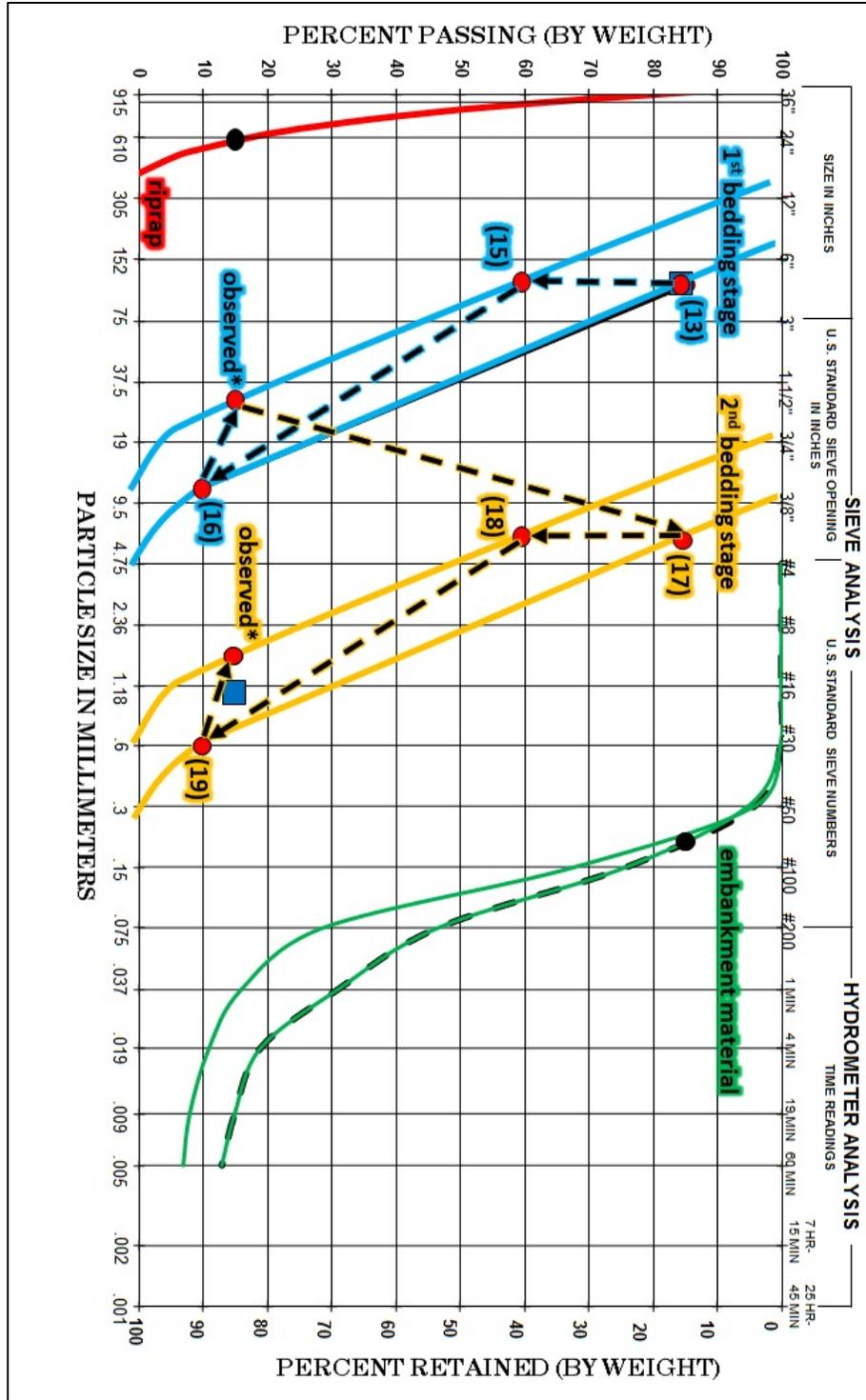
Figure 7.3.7.5-4. Steps used to define gradation bands for two layers of bedding. Blue arrows indicate steps used to define the first layer. Orange arrows indicate steps used to define the second layer. Numbers highlighted in blue indicate the equation used to determine the location of the point. The size of points with the “observed\*” label are estimated from the gradation band after it is constructed.
