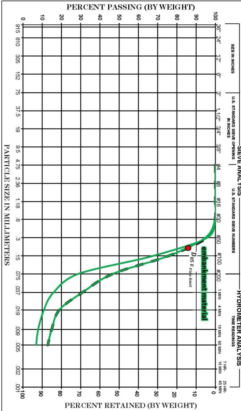
Figure C.5. Gradations of embankment material samples at Dam A.
