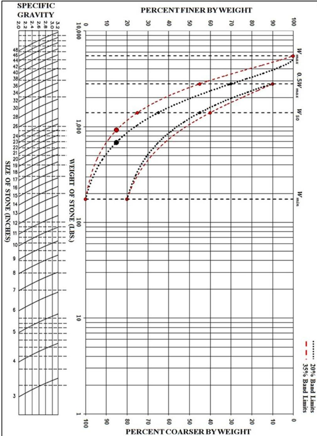
Figure C.4. Design riprap gradation band.  $D_{15 R Coarse limit}$  was estimated from coarse-limit curve of 35-percent band to have a value of 900 lbs.
