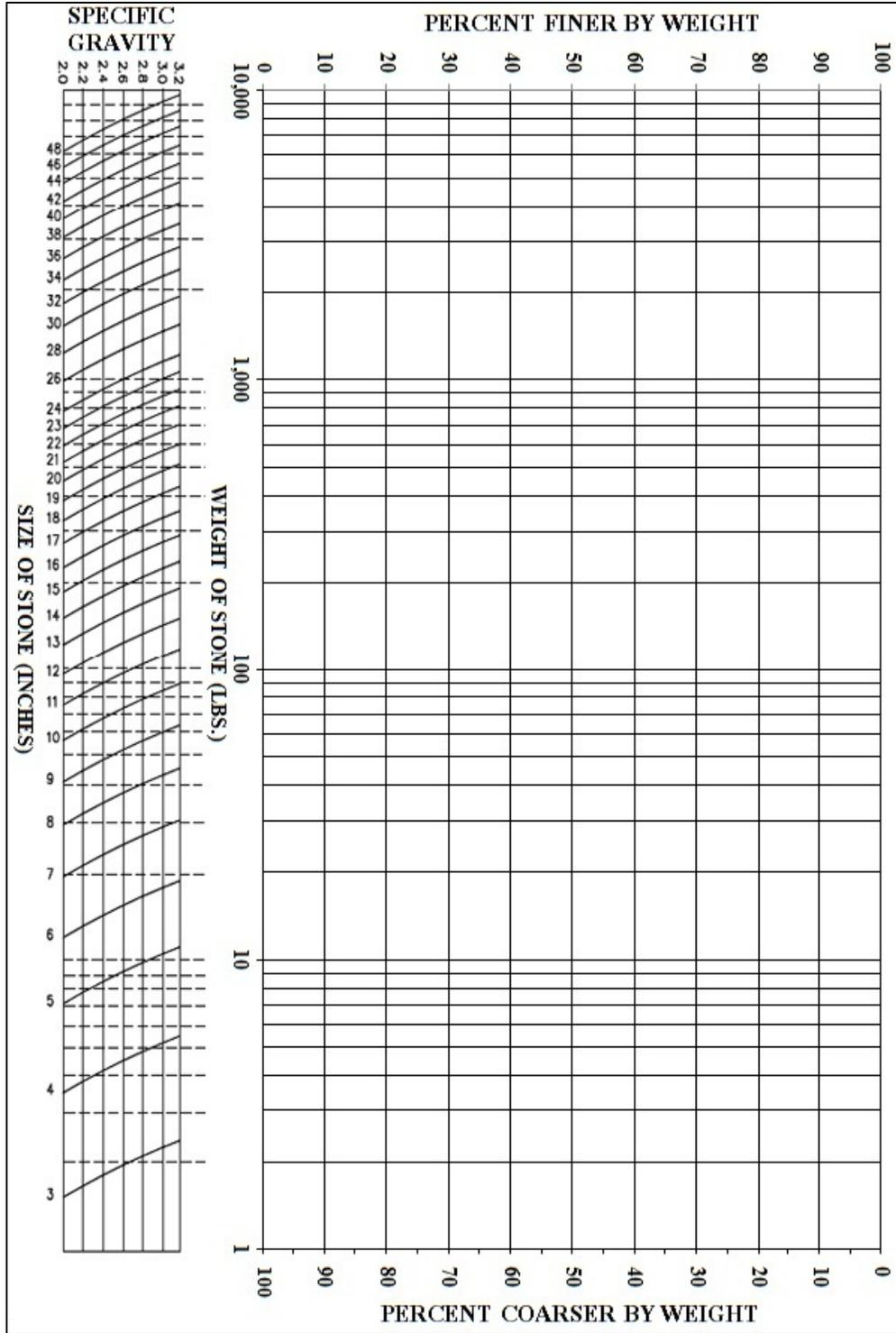
Figure 7.3.6-2. Blank riprap gradation, by weight (pounds). Equant shape assumed.
