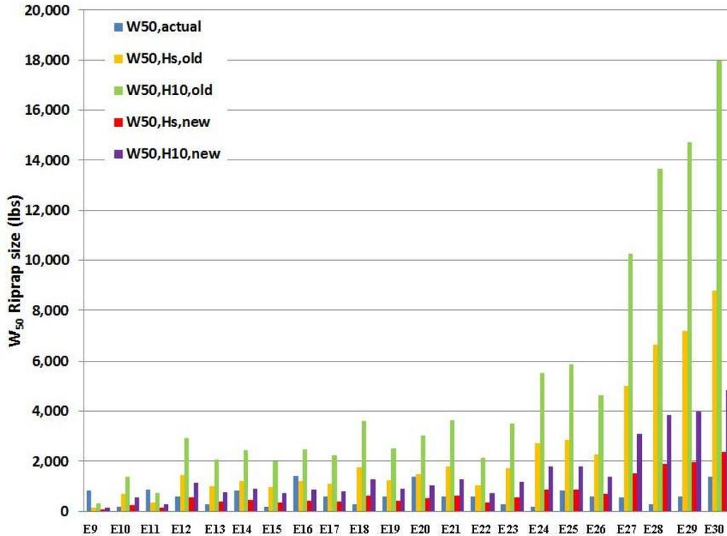
Figure D.3. Comparison of  $W_{50}$  sizes for riprap on dams where  $F > 1.2$
