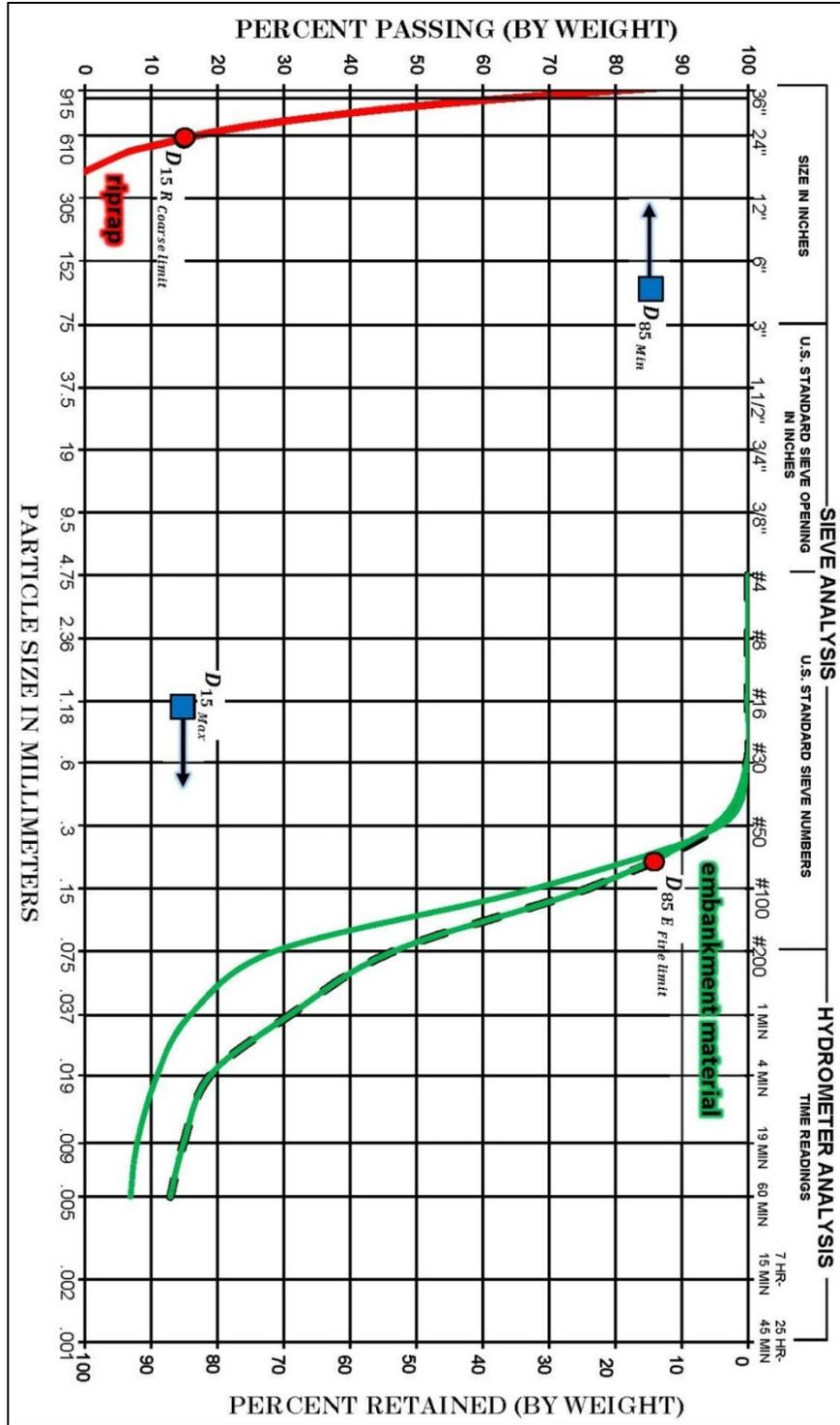
Figure 7.3.7.3-1. Bedding sizes required for particle retention  $D_{15 Max}$  and  $D_{85 E Fine limit}$  depicted by blue squares.
