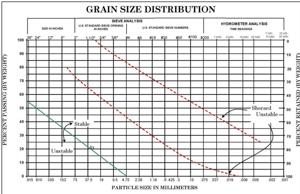
Figure 7.3.7.1-1. Bedding material instability chart; material may be internally unstable if it lies within Sherard's unstable bands or is flatter than the 4X line [15].
