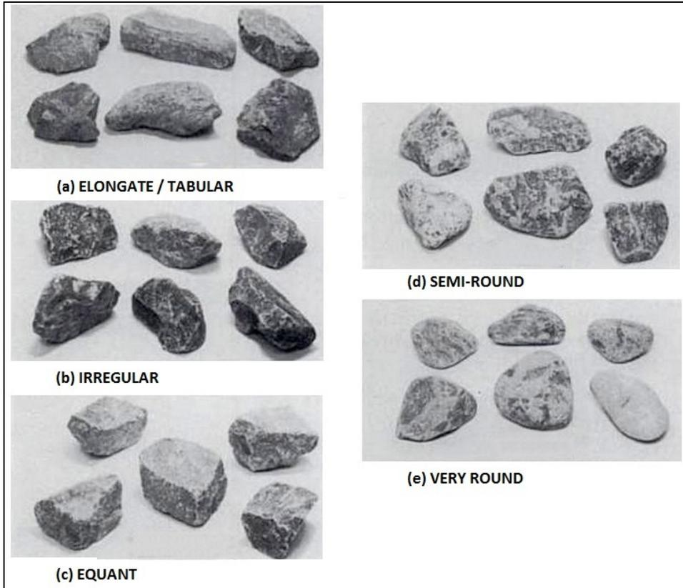
Figure 7.2.5-1. Visual comparison of block shapes (photo by H.R. Wallingford) [4].
