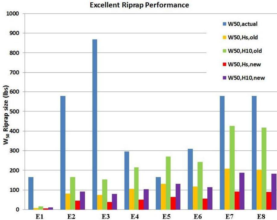
Figure D.2. Comparison of  $W_{50}$  sizes for riprap on dams where  $F < 1.2$ .
