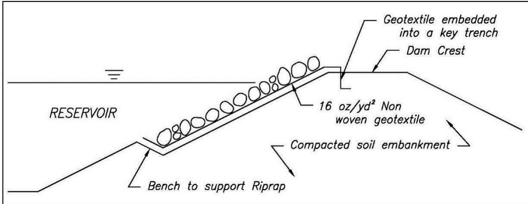
**Figure 19.4.3.2-3. Illustration showing the use of a bench to support the placement of riprap on a geotextile bedding to improve slope stability performance. In addition to the frictional resistance along the riprap/geotextile interface, the bench adds physical support, which is transmitted up the slope from one piece of riprap to the next one above it to resist sliding.**
