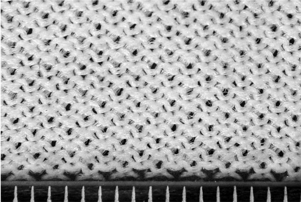
**Figure 19.2.2.3-1. Knitted multifilament geotextile, magnified view (1-mm scale). This geotextile is used as a filter placed around perforated pipe.**
