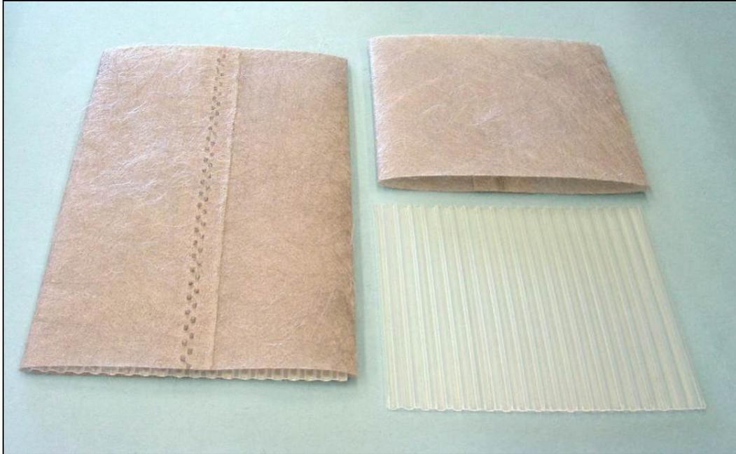
Figure 19.3.2.-2. Photograph of a wick drain composed of a polymeric corrugated core and outer heat set nonwoven geotextile. The assembled drain is on the left, and the components are shown on the right.
