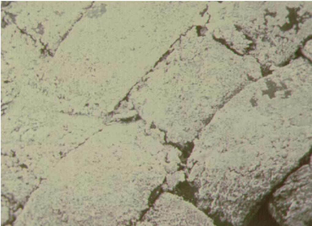
**Figure 19.4.1-3. Photograph (magnified view) of soil filter cake built up on the geotextile and bridging across the openings between the fibers. Photograph courtesy of Dr. George Koerner.**
