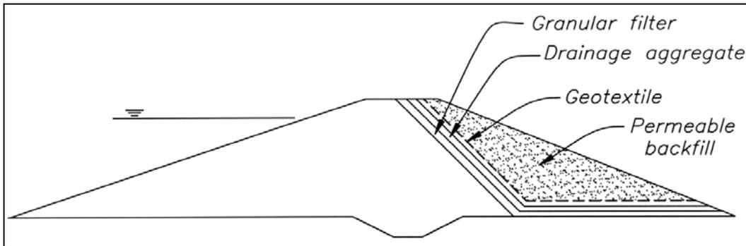
Figure 19.4.3.3-1. Illustration showing a geotextile being used to separate a downstream aggregate drain from the overlying backfill (shell material).
