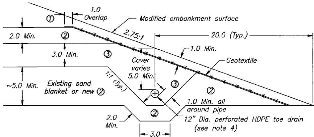
Figure RW9. Cross section showing toe drain detail with geotextile separating zone 1 from the zone 2 sand and the zone 3 gravel.
