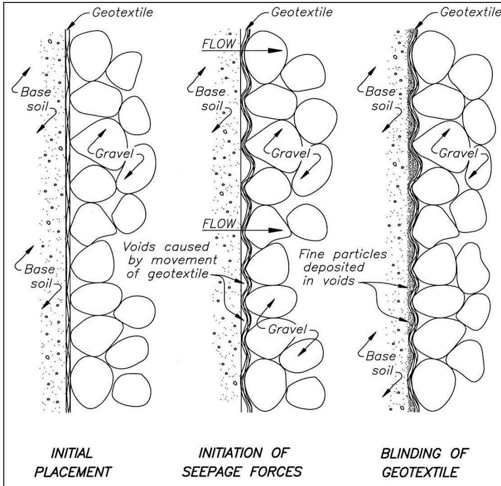
Figure 19.4.1-4. Illustration showing the progressive steps leading to blinding of a geotextile, which is a type of excessive clogging that deposits a layer of fine soil particles on the geotextile. It can be caused by using drainage aggregate that is too large in size.
