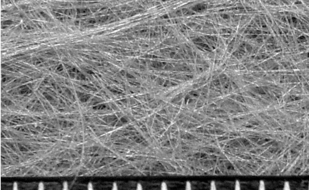
**Figure 19.2.2.2-3.** Photograph of a nonwoven continuous-filament needle-punched spun-bond geotextile, magnified view (1-mm scale). This geotextile is only lightly “heat set” (lightly fused together).
