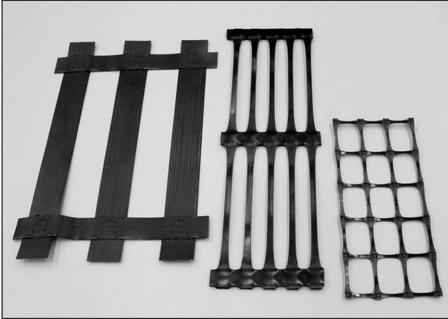
**Figure 19.3.4-1. Photograph showing examples of geogrids. Geogrids have supplanted geotextiles in many reinforcement applications where high-strength reinforcement of granular soils is required.**
