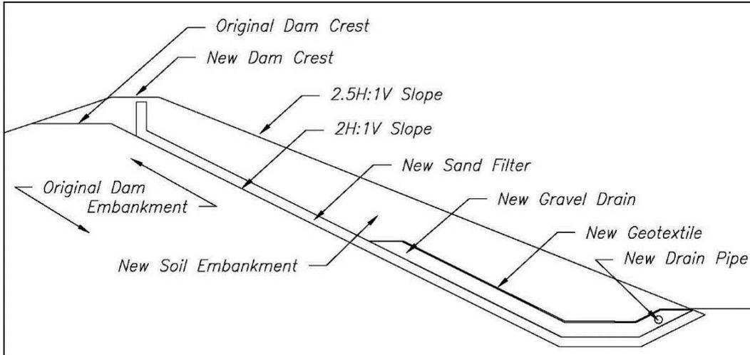
**Figure A1. Cross section showing geotextile separator to prevent migration of fine soil from new embankment fill into gravel drain.**
