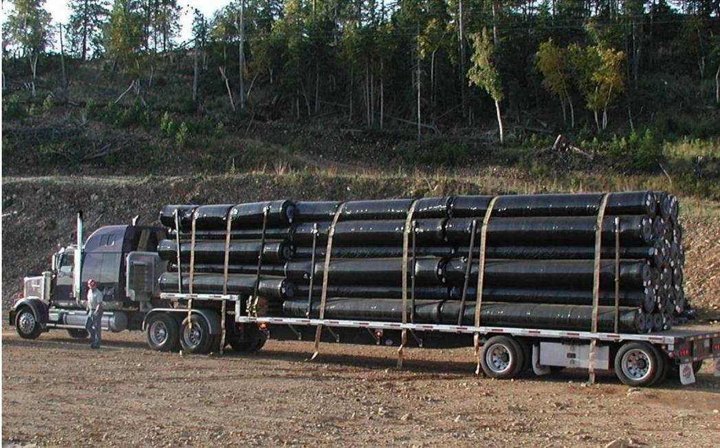
**Figure 19.5-1. Photograph showing delivery of geosynthetic rolls to a construction site. The tiedown straps at the front of the truck are intruding into and have distorted the shape of the top roll, which must be examined to verify that it has not been damaged.**
