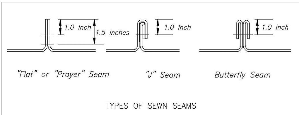
**Figure 19.6.3-1. Illustration showing types of sewn seams used to join geotextile panels.**
