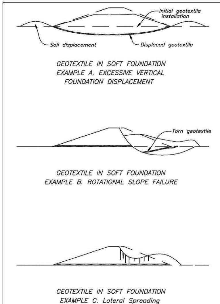
**Figure 19.4.4.2-1. Illustration showing types of foundation failures.**
