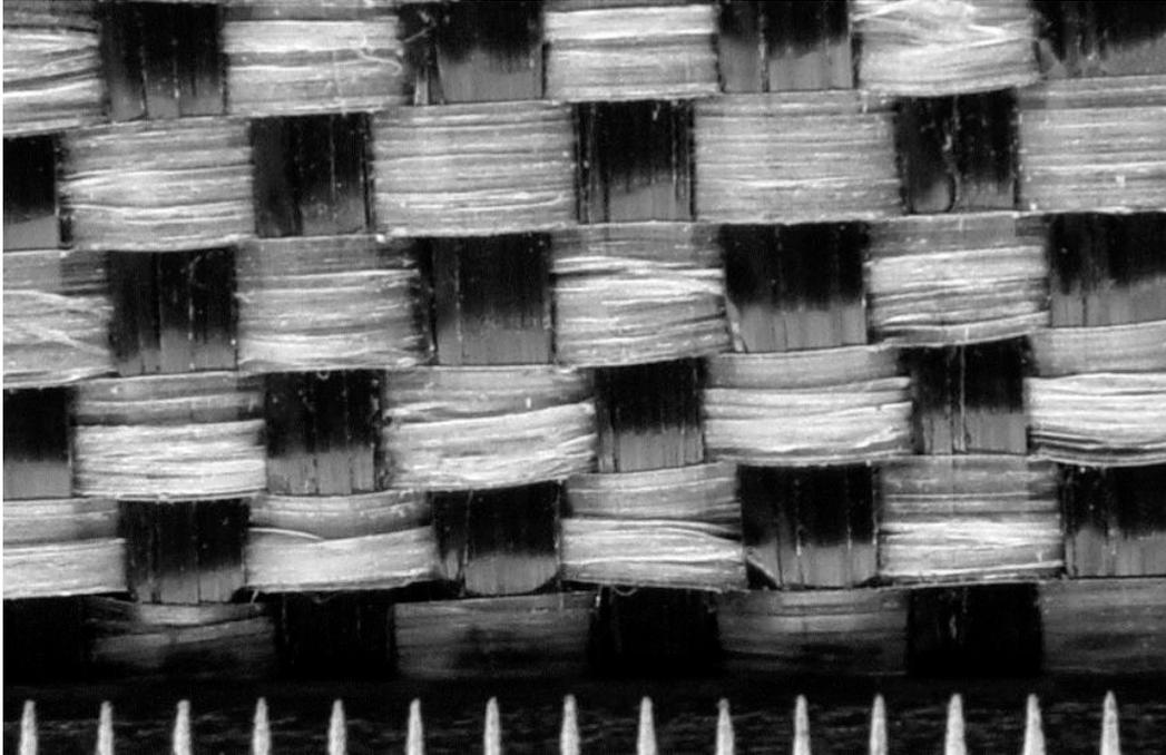
**Figure 19.1.2.1-2. Woven fibrillated slit film geotextile, magnified view (1-mm scale). This geotextile has a greater porosity and is therefore more permeable than that shown on figure 19.2.2.1-1.**
