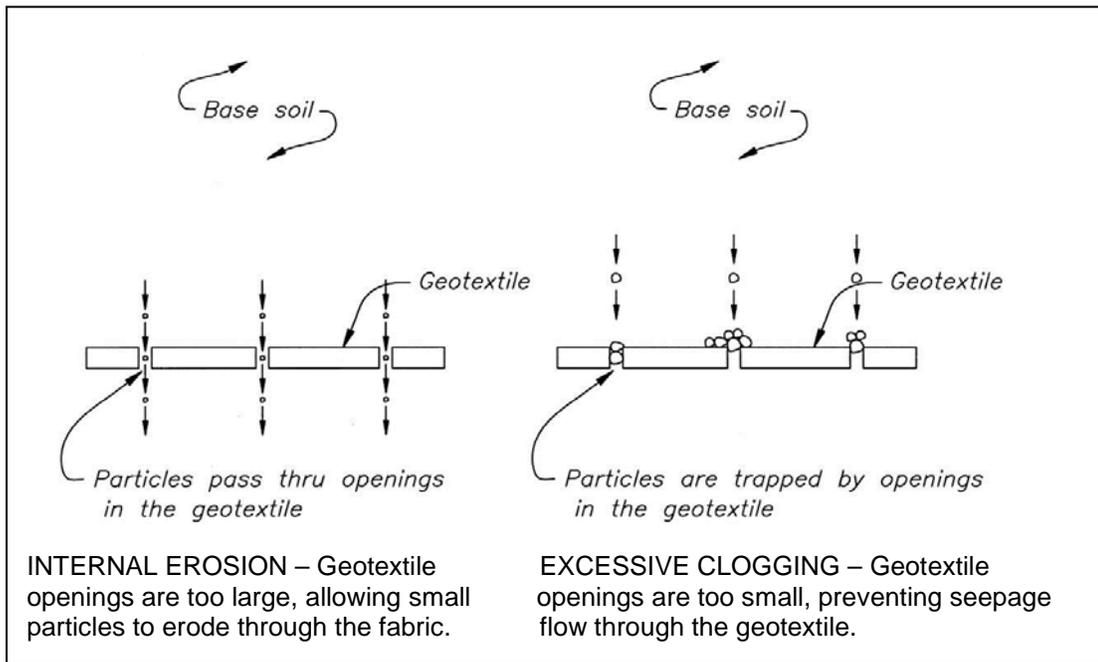
**Figure 19.4.1-1. Illustration of a geotextile filter showing the concepts of soil internal erosion and excessive clogging. In each case, a permeable “filter cake” fails to form; thus, the geotextile is not suitable as a filter.**
