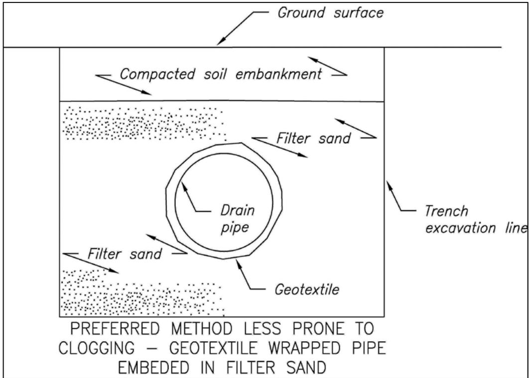
Figure 19.4.3.5-5. Toe drain formed by placing a geotextile filter around a perforated drainpipe, which is embedded in filter sand.
