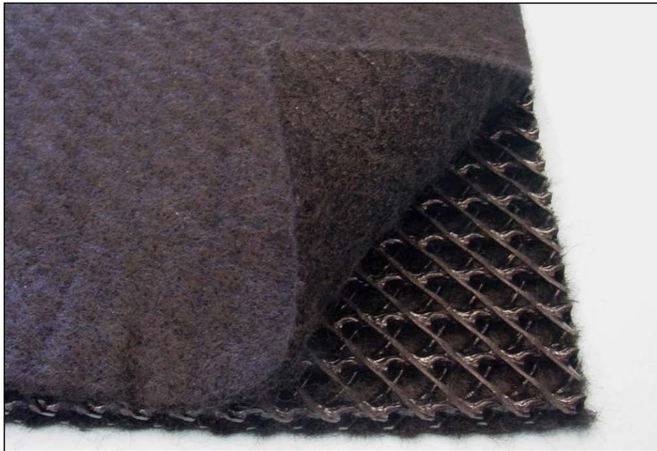
**Figure 19.3.2-1. Photograph of a geonet composite drain made by bonding nonwoven geotextiles to each side of a tri-planar geonet. One corner of the upper geotextile layer has been peeled back to show the underlying geonet core.**
