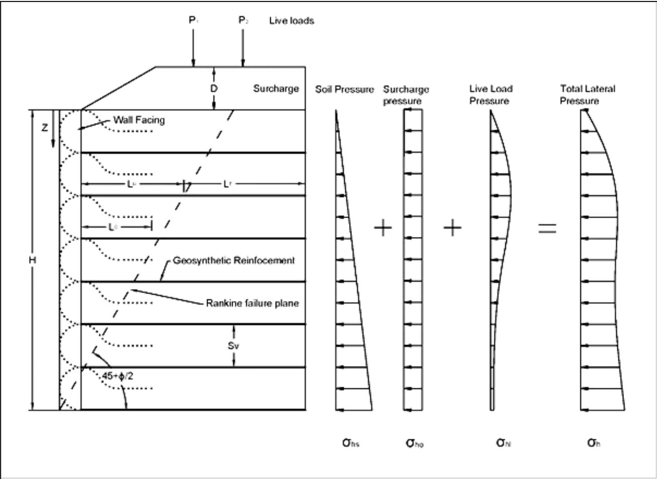
Figure 19.4.4.4-1. Rankine earth pressure concepts for geosynthetic reinforced soil wall design (after Koerner, 2012).
