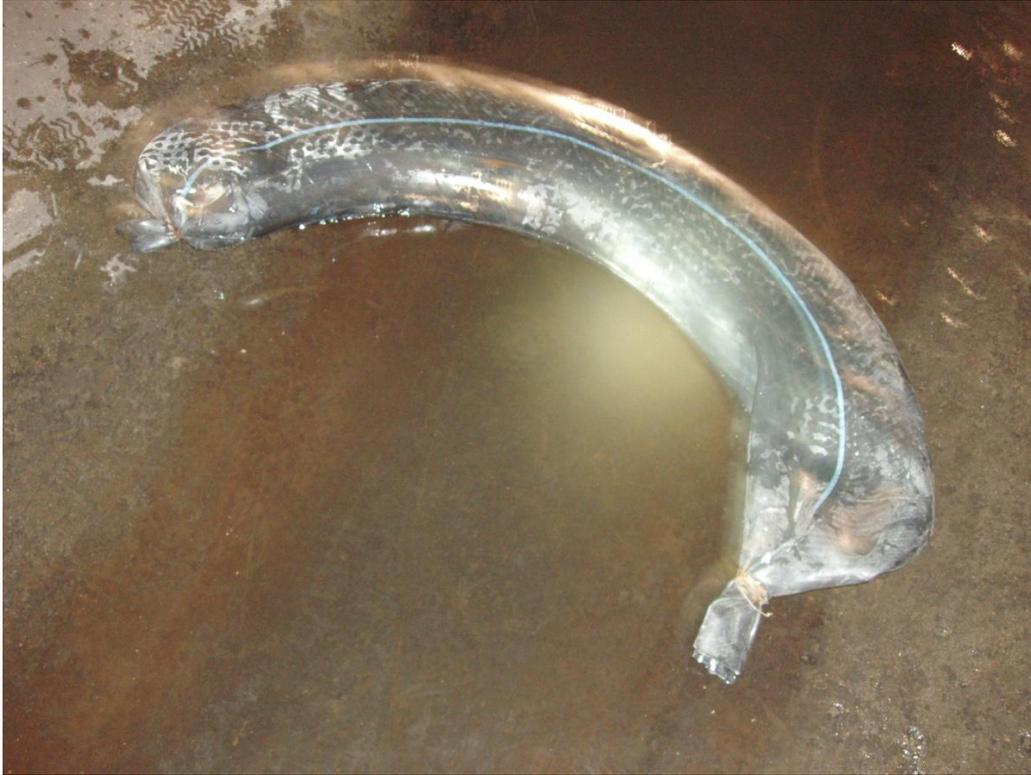
**Figure HB6. Photograph showing a sand-filled inner tube that was used to form a temporary sediment trap within the conduit about 10 feet downstream from the geotextile filter installation.**
