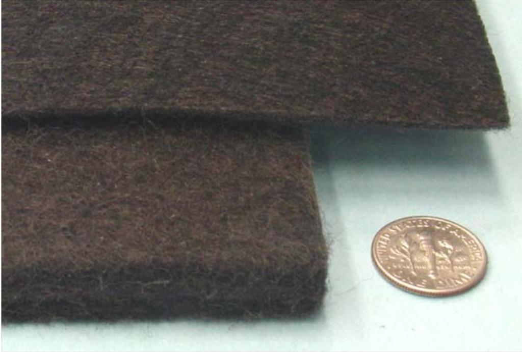
**Figure 19.2.2.2-1. Examples of nonwoven needle-punched geotextiles showing variation in thickness with mass. At top, a 4 oz/yd<sup>2</sup> geotextile, and at lower left, a 32 oz/yd<sup>2</sup> geotextile.**
