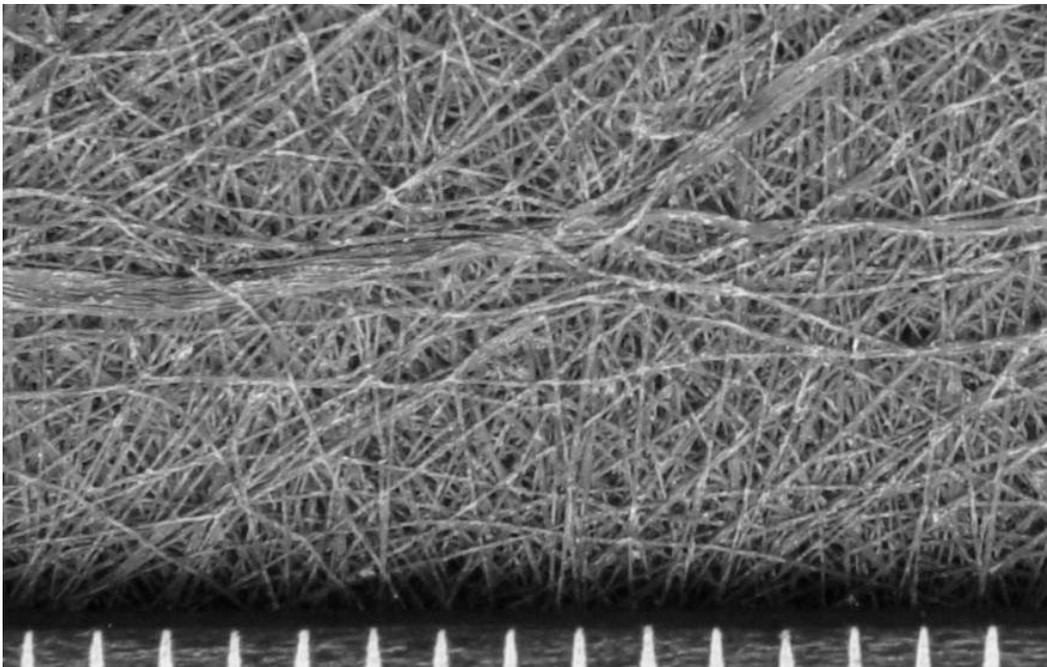
**Figure 19.2.2.2-4.** Photograph of a nonwoven continuous-filament spun-bond and heat-bonded geotextile, magnified view (1-mm scale). The fibers in this geotextile have a heavy “heat set.” The fibers are more thoroughly melted to fuse them together than the example on figure 19.2.2.2-3. This geotextile is used as a filter wrapping for wick drains.
