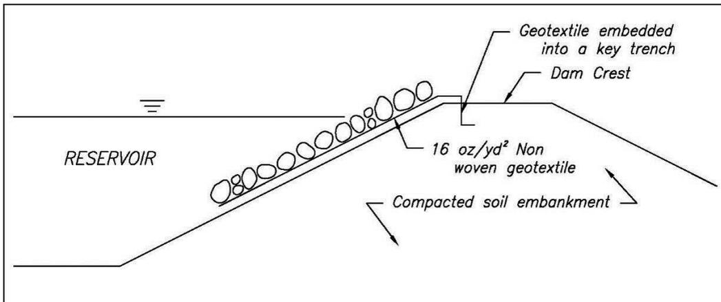
**Figure 19.4.3.2-1. Illustration of riprap on geotextile bedding at a small dam in Arizona. This installation experienced a slope failure. The riprap slid along the interface between the riprap and the underlying geotextile.**
