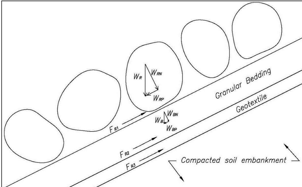
**Figure 19.4.3.2-4. Illustration of static forces showing three frictional interfaces to be evaluated:  $F_{R1}$  riprap on a granular bedding,  $F_{R2}$  granular bedding on geotextile, and  $F_{R3}$  geotextile on compacted soil embankment.**
