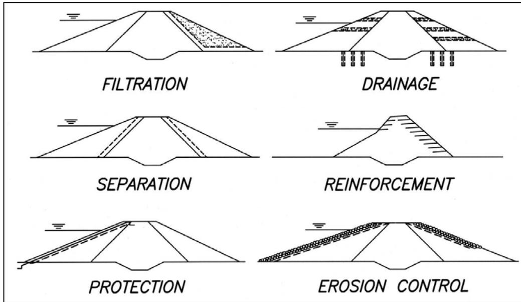
Figure 19.3-1. A graphical representation of various geotextile functions in earthen dams.
