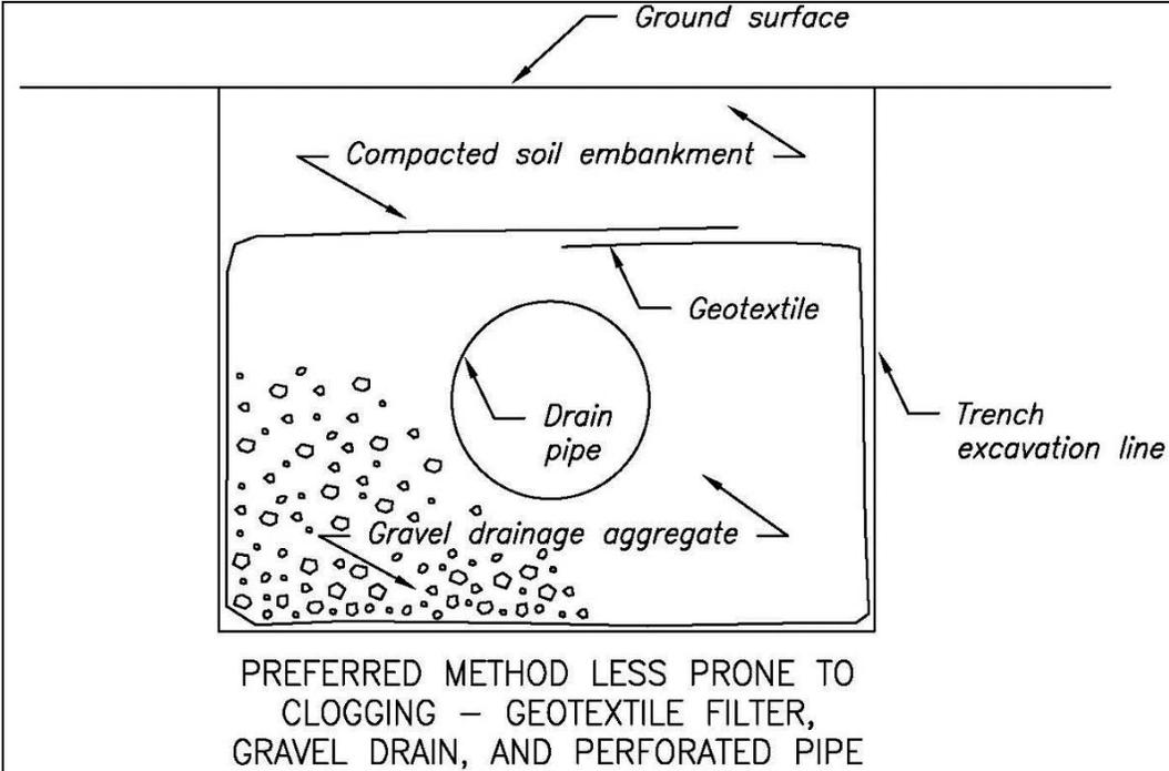
Figure 19.4.3.5-4. Toe drain formed by placing a geotextile filter around a gravel aggregate drain.
