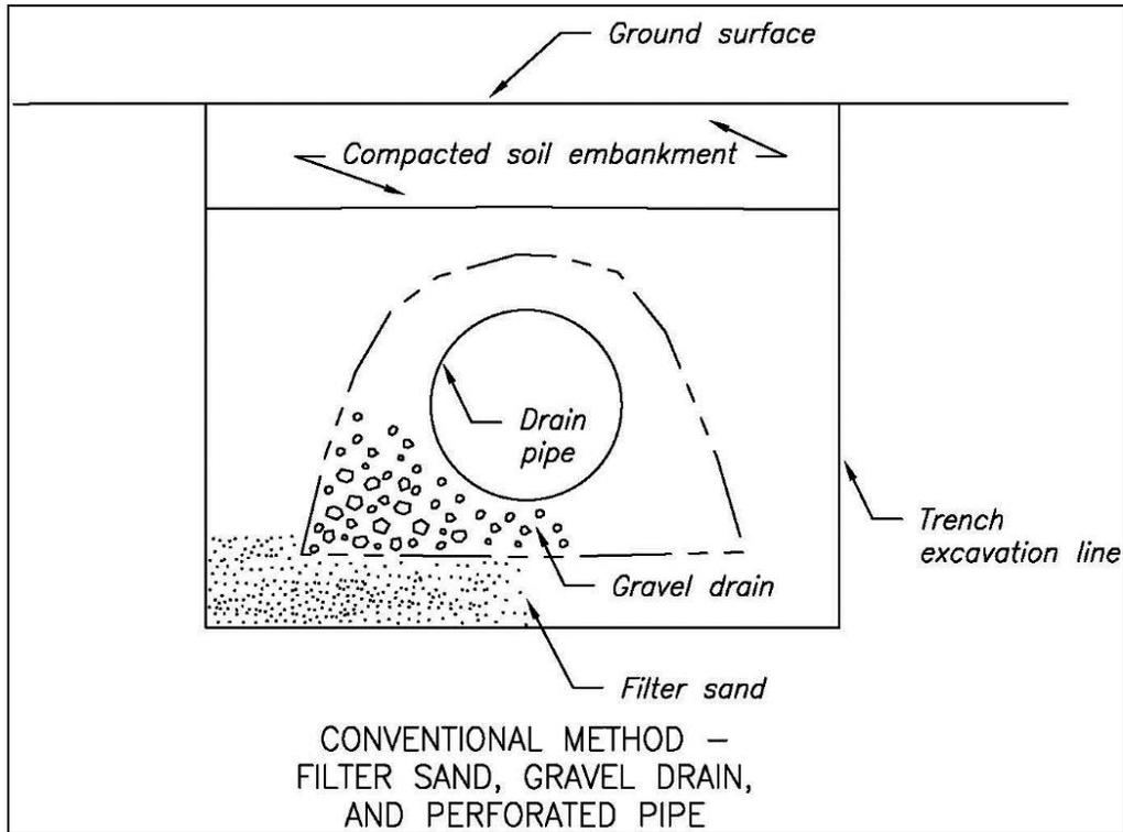
**Figure 19.4.3.5-1. Conventional toe drain construction without a geotextile is formed by placing a sand filter around a gravel aggregate drain containing a perforated drainpipe.**
