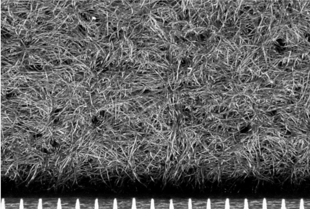
**Figure 19.2.2.2-2. Photograph of a nonwoven needle-punched staple-fiber geotextile, magnified view (1-mm scale). The needle holes are visible in the photograph. The entanglement of the fibers holds the fabric together.**
