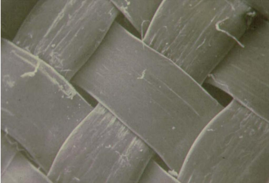
**Figure 19.4.1-2. Photograph (magnified view) of a woven geotextile showing openings between the woven fibers. Photograph courtesy of Dr. George Koerner.**
