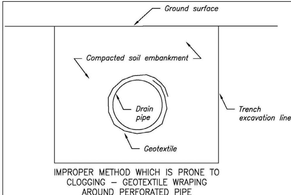
**Figure 19.4.3.5-2. Toe drain formed by placing a geotextile filter around a perforated drainpipe. Although this method eliminates the need for sand and gravel, there are many cases of excessive clogging of the geotextile.**
