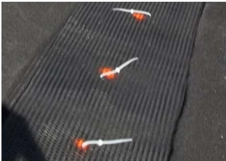
**Figure RW6. Photograph showing a closeup view of nylon ties joining the geonet layer of the geonet composite.**
