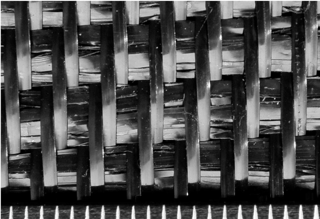
**Figure 19.2.2.1-1. Woven monofilament (vertical fibers) and fibrillated slit film (horizontal fibers) geotextile; magnified view, a scale with 1-mm gradations is shown along the bottom of the photograph. There are pore spaces at the junctions between the vertical and the horizontal fibers. The horizontal fibers also have a secondary porosity due to the secondary cuts (fibrillation) in the horizontal fibers, which can be seen in the photograph.**
