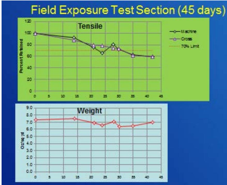
Figure RW7. Field exposure test section results for the Red Willow Dam geotextile. The horizontal axis is exposure time in days. The vertical axis for the upper graph is percent tensile strength retained. The vertical axis for the lower graph is fabric weight in oz/yd<sup>2</sup>.
