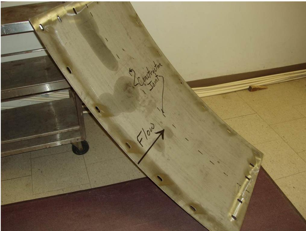
**Figure HB2.** Photograph showing the fabricated stainless steel plate that will be used to attach a geotextile to the outlet works conduit. Note the slots down the middle to allow seepage through the plate. Slots around the perimeter are for the anchor bolts.
