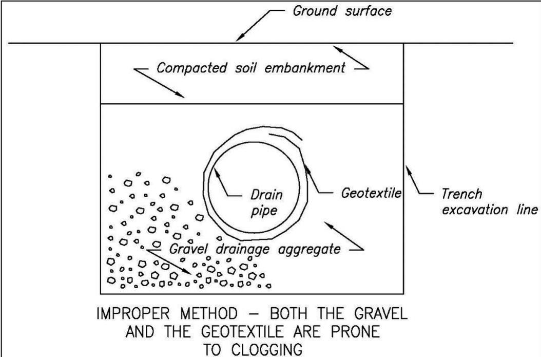
Figure 19.4.3.5-3. Toe drain formed by placing a geotextile filter around a perforated drainpipe surrounded by a gravel aggregate drain. This method is prone to clogging if the gravel does not filter the surrounding soil embankment.
