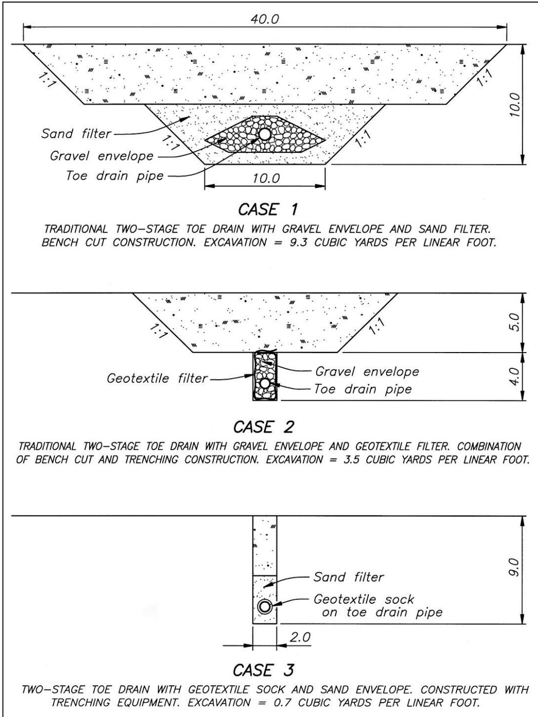
Figure MF2. Illustration showing the required amounts of excavation for three different toe drain configurations.
