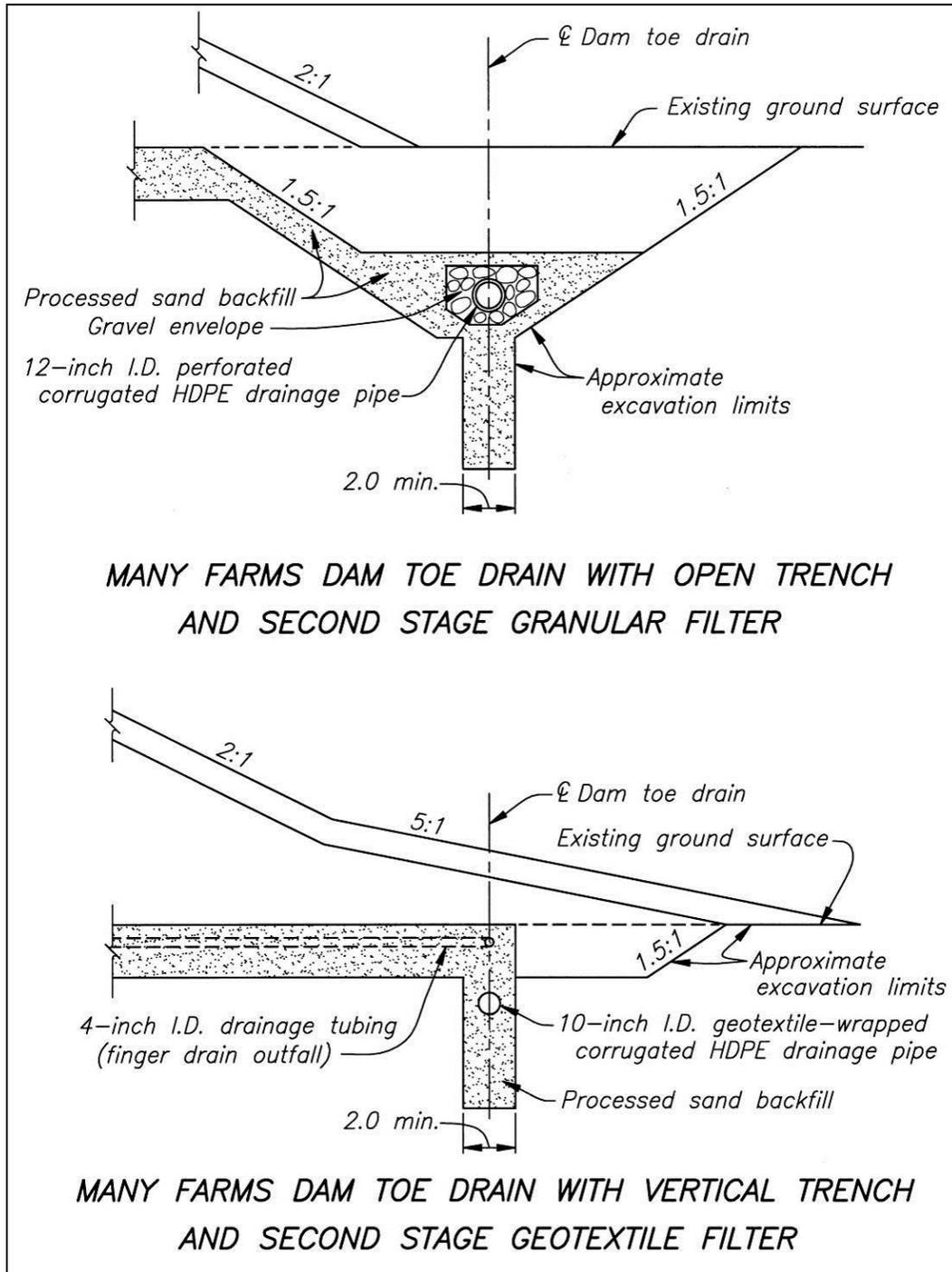
Figure MF1. Illustration showing the original Many Farms Dam toe drain design with a two-stage granular filter (at top) and the re-designed toe drain with a single granular filter containing a geotextile-wrapped pipe.
