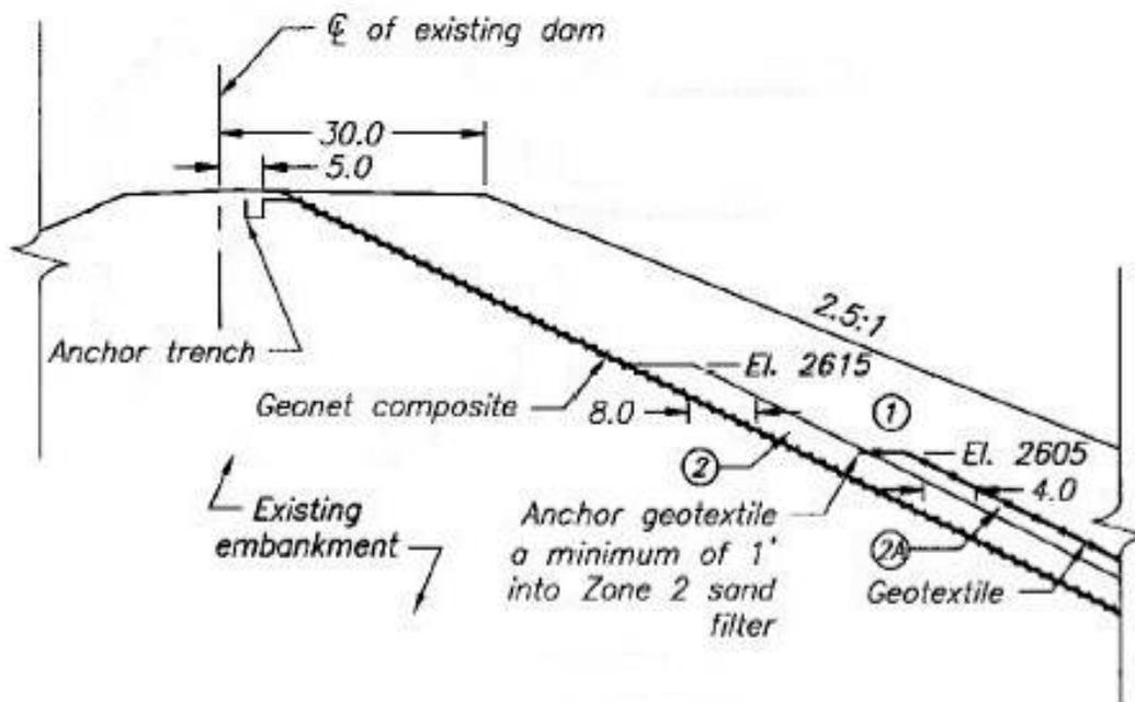
**Figure RW1. Cross-section view of Red Willow chimney filter and drain incorporating a geonet composite.**
