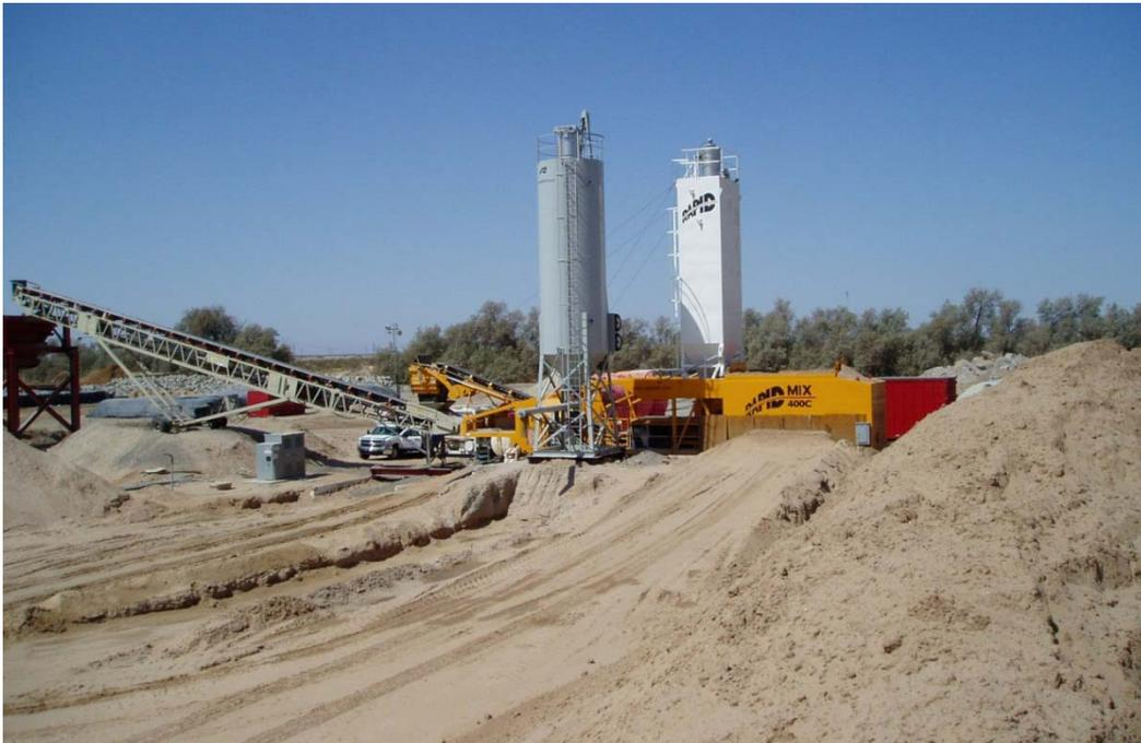
**Figure 17.6.2-1. Pugmill used to make soil-cement at Warren H. Brock Reservoir, California.**
