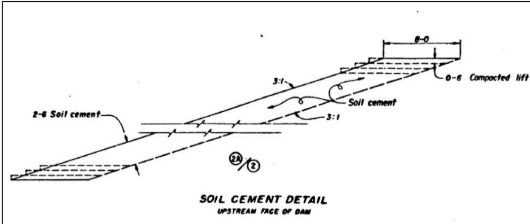
Figure 17.5.3-1. Typical stairstep soil-cement configuration.
