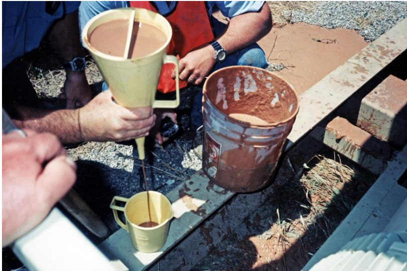
Figure 16.4.1.1-1. Marsh funnel viscosity test being performed on fresh bentonite slurry.
