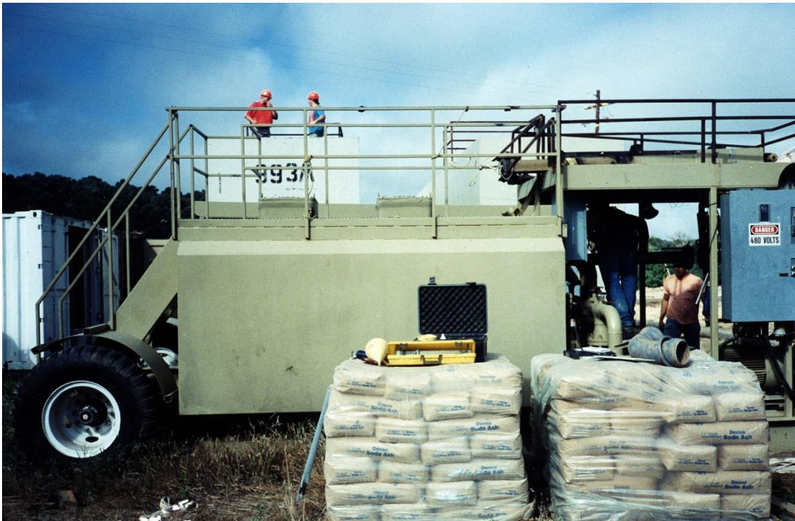
Figure 16.4-2. SB equipment for mixing slurry (high-speed colloidal mixer shown) (Bradbury Dam, California).
