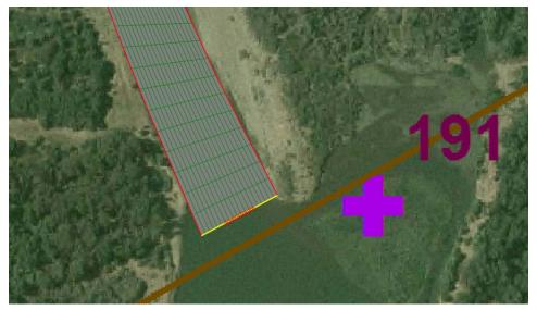
Figure 5-15. Downstream boundary condition line.
