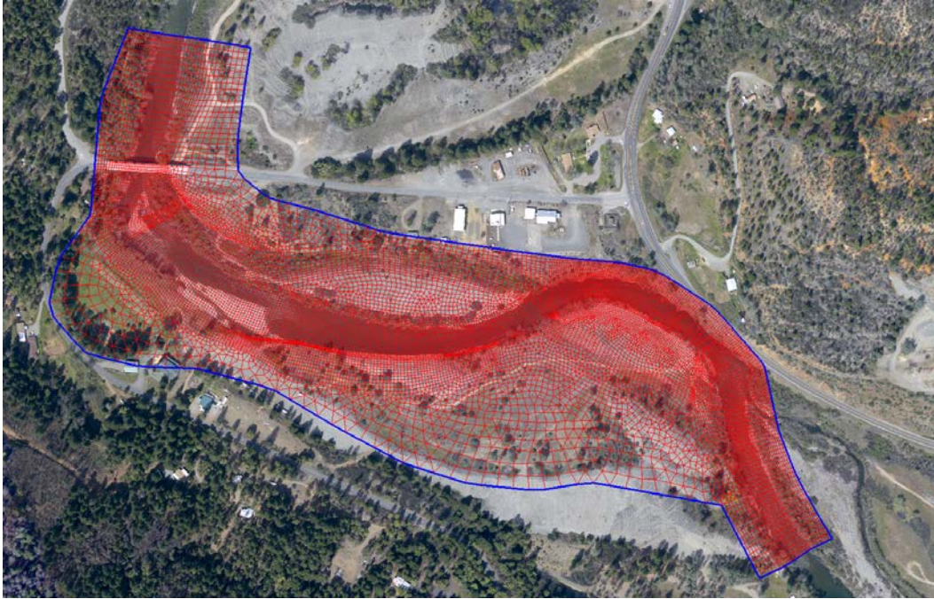
Figure 7. Solution domain (blue) and the mesh (red) for the PB (pre-erosion baseline) condition modeling (aerial photo was in April 2009).
