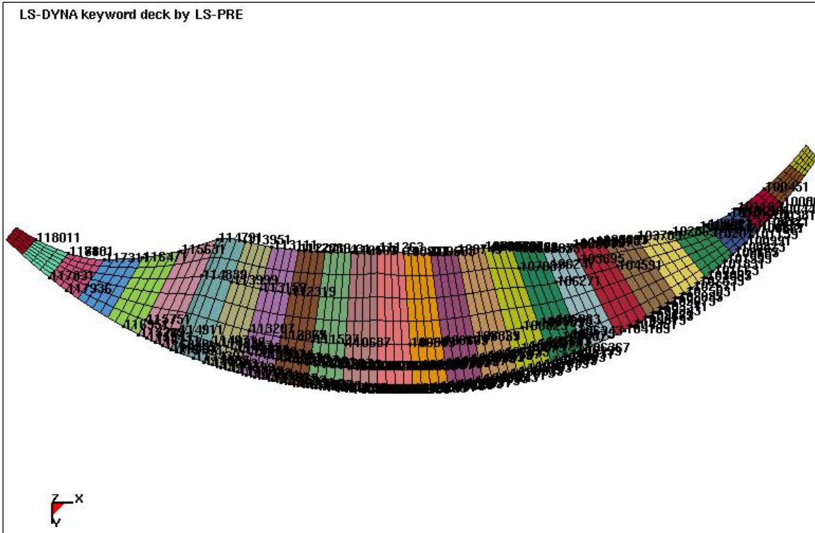
Figure E-4-8.—Nodes that separated for 50k earthquake ground motions at 5% damping.
