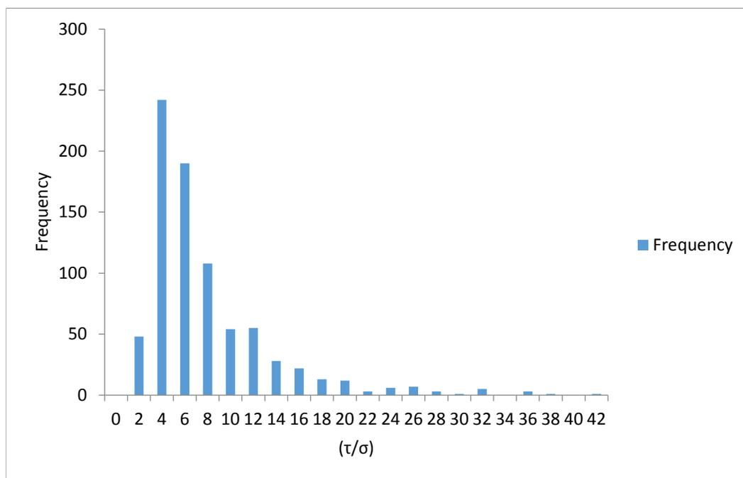
**Figure 15 - Histogram of the stress ratio at failure.**
