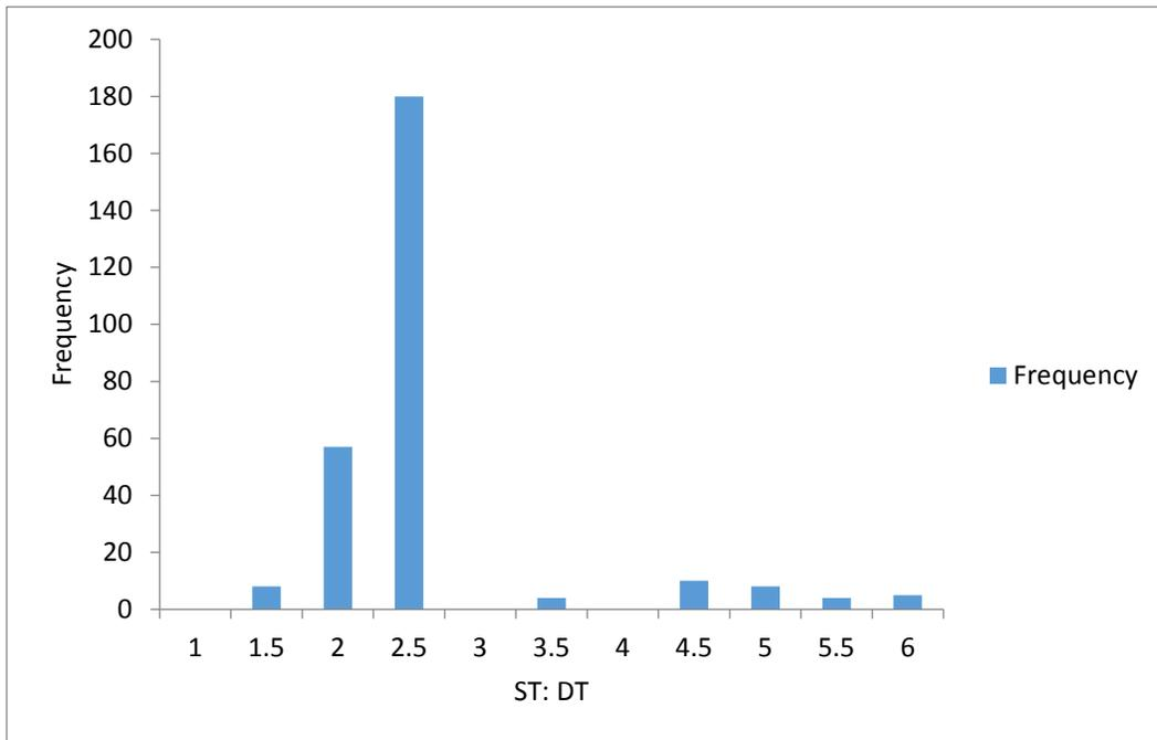
**Figure 6 - Histogram of the ratio between splitting tensile and direct tensile strengths (ST/DT).**
