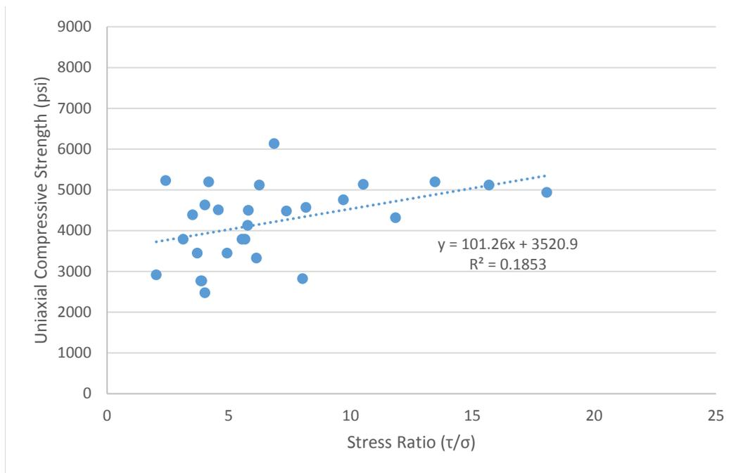
**Figure 56 - Concrete lift lines with AAR issues break-bond. Uniaxial compressive strength versus stress ratio.**
