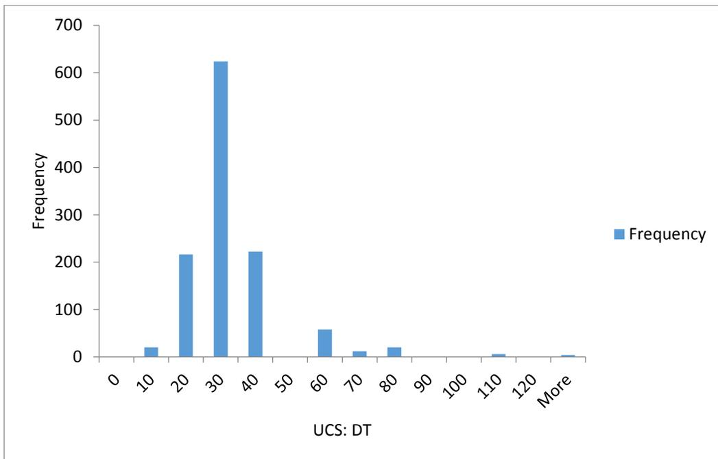
**Figure 8 - Histogram of the ratio between uniaxial compressive and direct tensile strengths (UCS/DT).**
