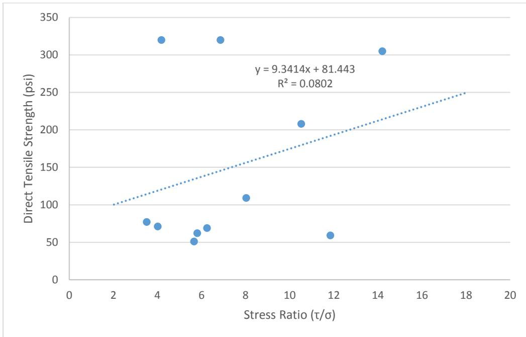
**Figure 55 - Concrete lift lines with AAR issues break-bond. Direct tensile versus stress ratio.**
