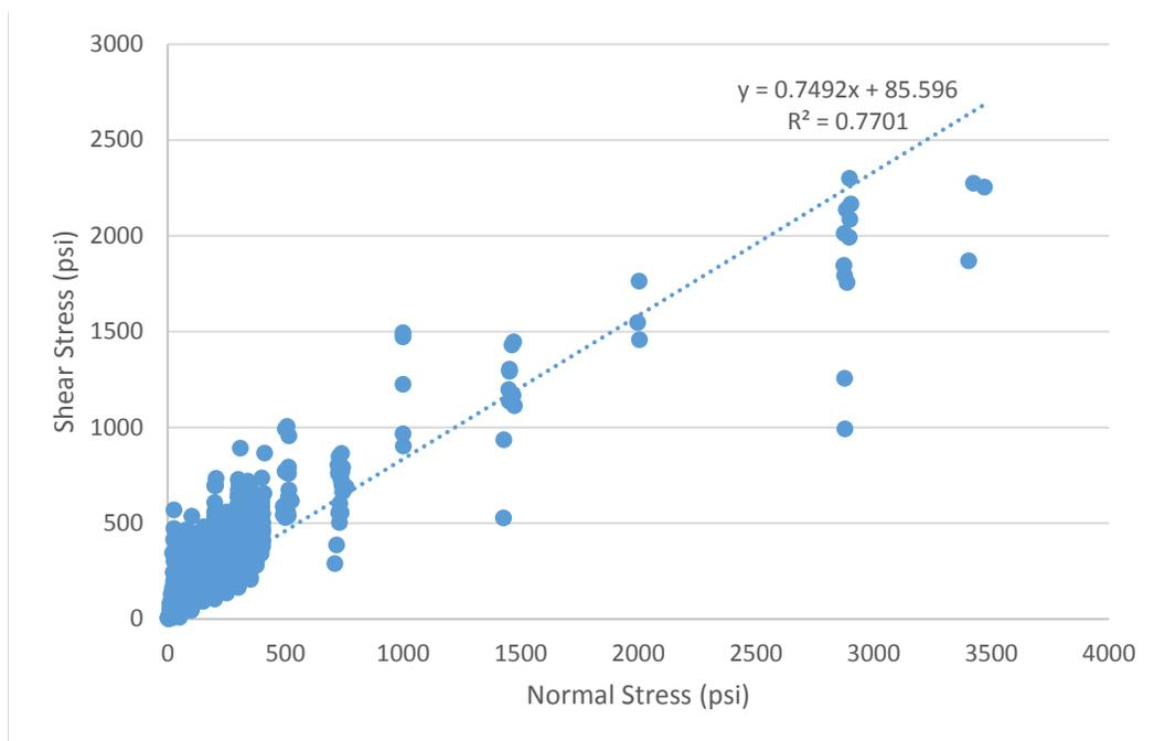
**Figure 24 – All data sliding shear strength test data.**
