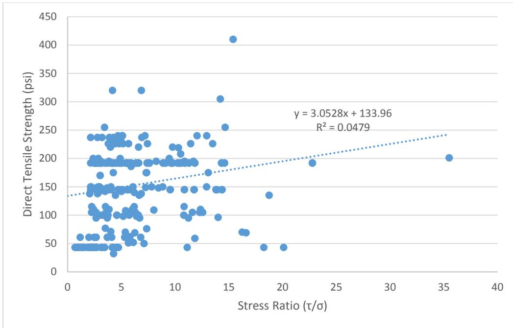
**Figure 13 – All data break-bond direct tensile versus stress ratio. The average direct tensile strength is 154 psi.**
