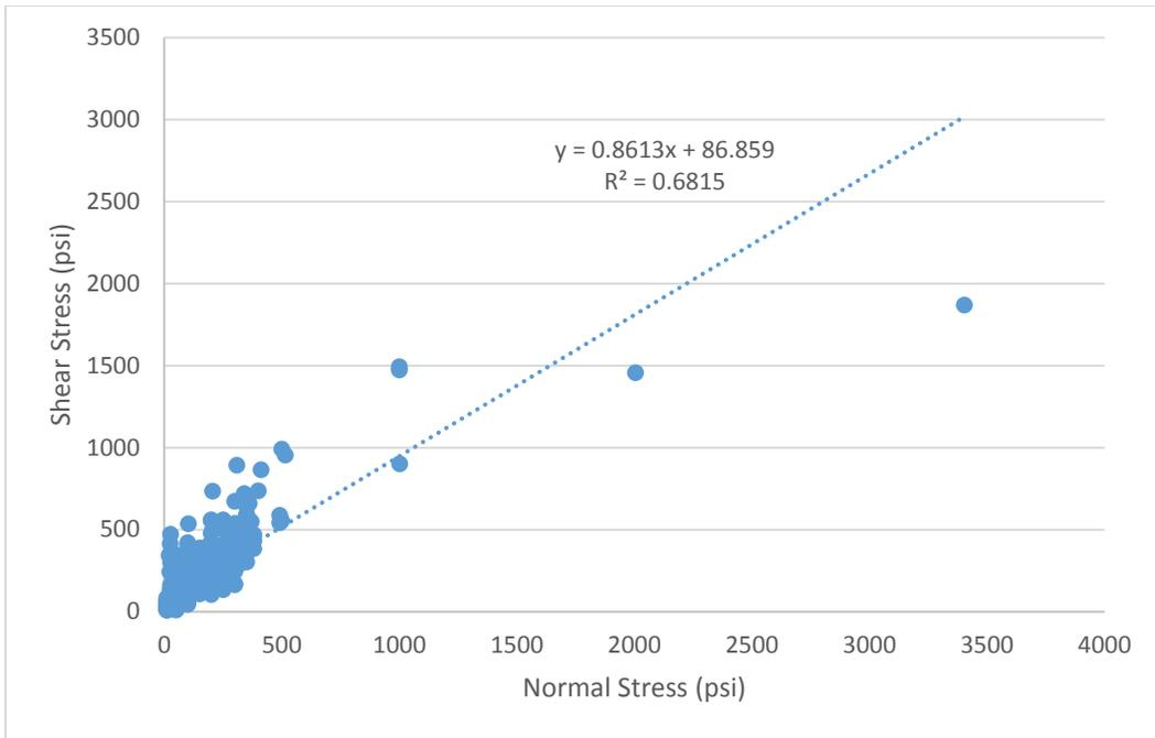
**Figure 45 - Conventional concrete lift line sliding shear strength.**
