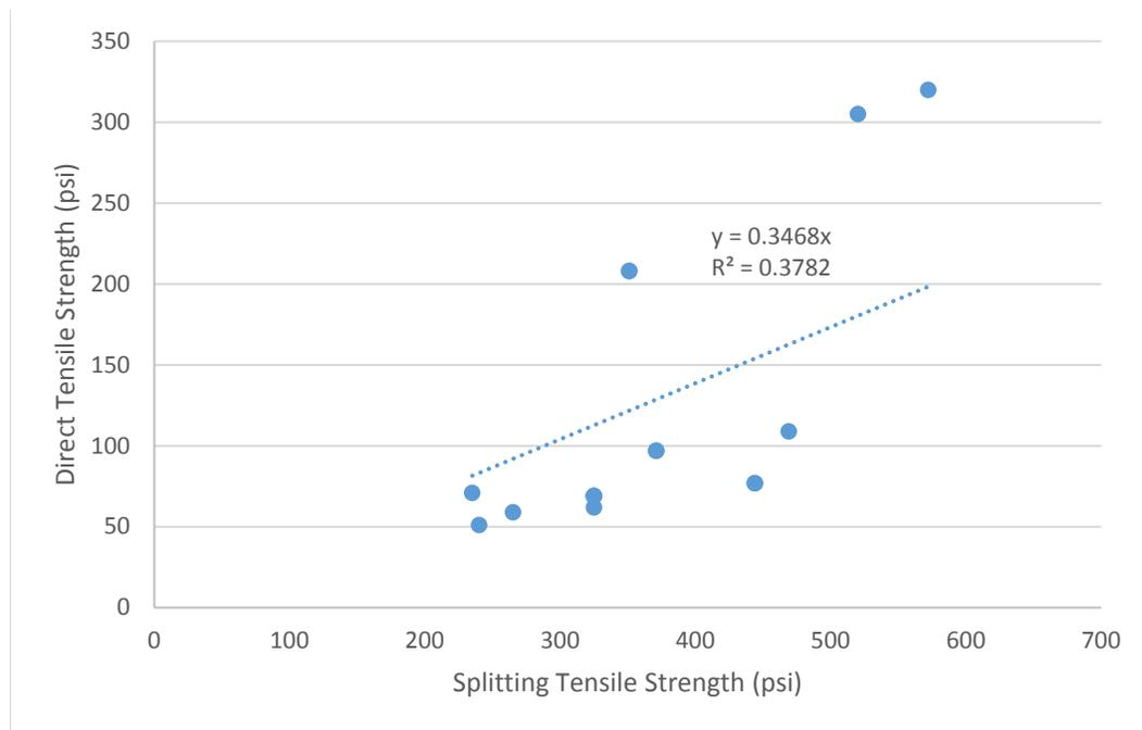
**Figure 52 - Concrete lift lines with AAR issues. Direct tensile versus splitting tensile strength.**
