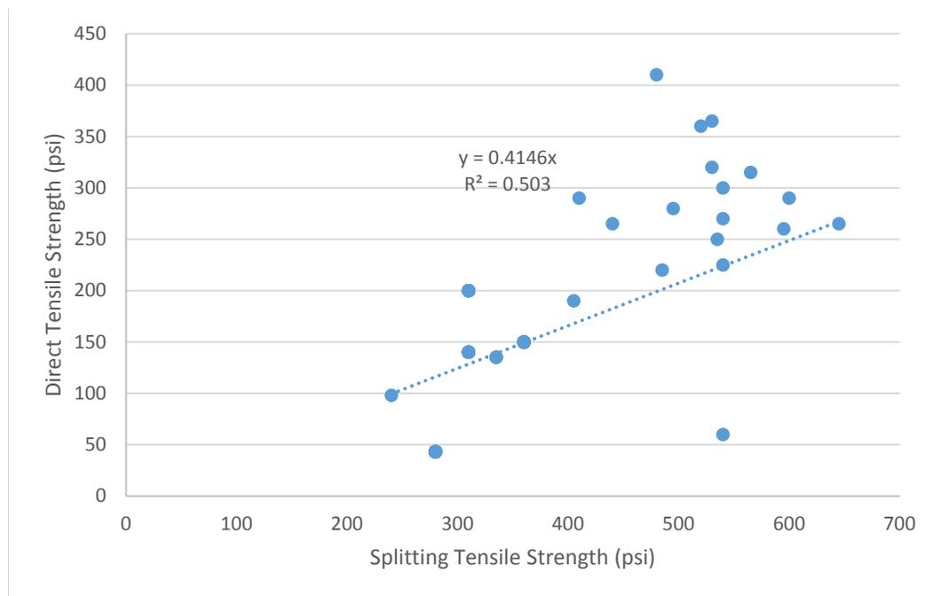
**Figure 40 - Conventional concrete lift line, direct tensile versus splitting tensile strength.**
