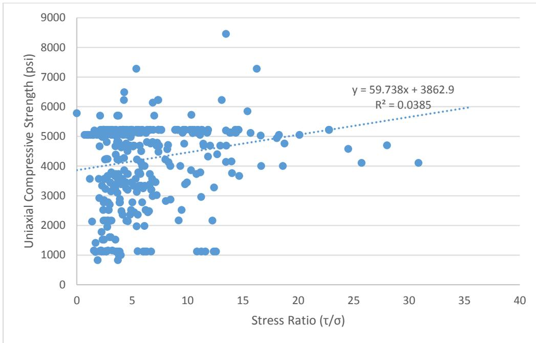
**Figure 14 – All data break-bond uniaxial compressive strength versus the stress ratio. The average uniaxial compressive strength is 4,239 psi.**
