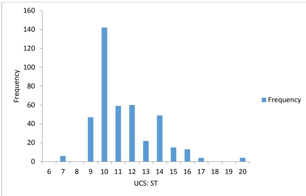
**Figure 7 - Histogram of the ratio between uniaxial compressive and splitting tensile strengths (UCS/ST).**
