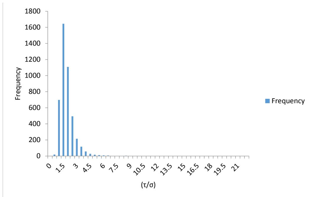
**Figure 32 - Histogram of stress ratio at failure for all data sliding shear strength tests.**
