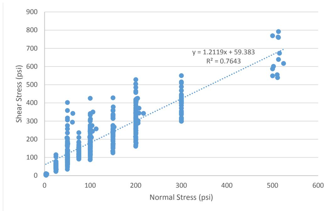
**Figure 57 - Concrete lift lines with AAR issues, sliding shear strength data.**
