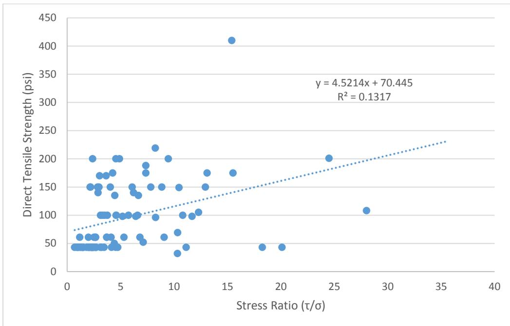
Figure 43 - Conventional concrete lift line break-bond data showing direct tensile strength versus stress ratio.
