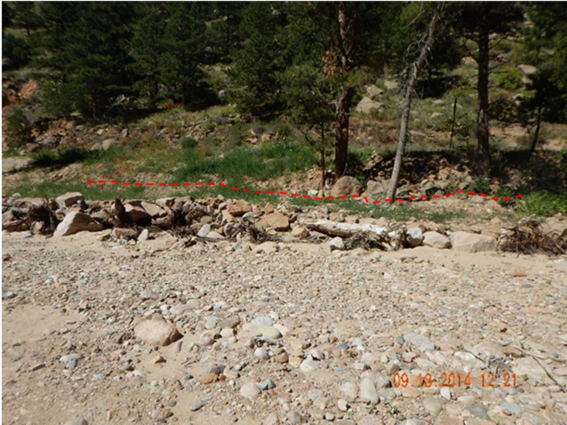
FIGURE 3.4: SITE SSV1 ON THE SOUTH SAINT VRAIN RIVER NEAR LYONS. LOOKING UPSTREAM, EVIDENCE OF HWMS ON THE LEFT BANK
