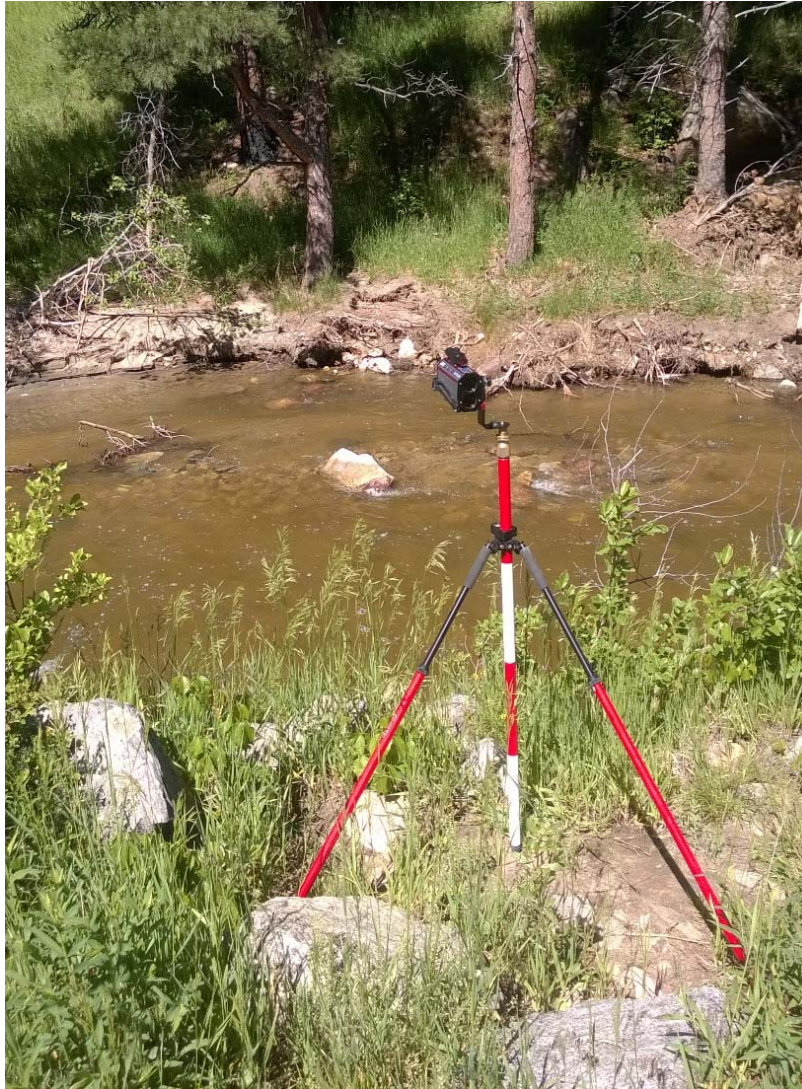
FIGURE 3.1: LIGHT WEIGHT HAND-HELD LASER RANGING INSTRUMENT USED TO COLLECT SURVEY DATA FOR THE DETERMINATION OF A CHANNEL SINGLE CROSS SECTION AT EACH SITE.
