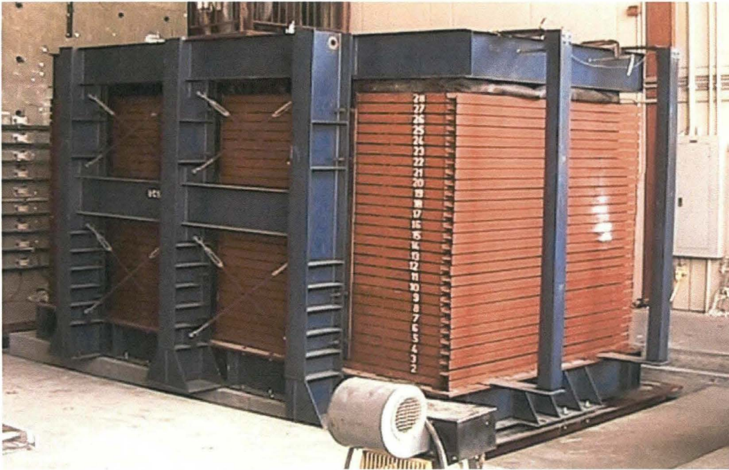
Figure 6. – UCSD on-campus shake table container to accommodate 6.7 ft (2 m) high walls.
