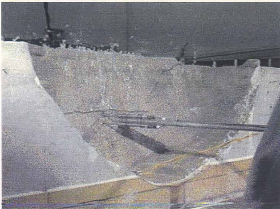
Model M10 – 8/2/00, South view camera initial cracking
