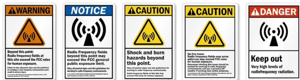
FIGURE 30-1. Examples of warning and danger signs that may be required at a tower site.
