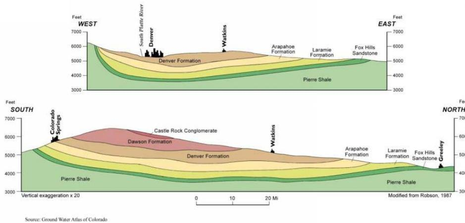
**Figure 2. Geologic cross sections of the Denver Basin**
