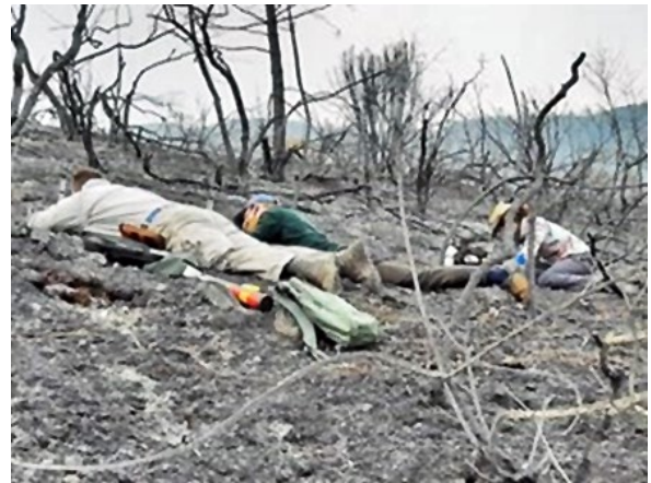
USGS scientists measuring infiltration rate.
