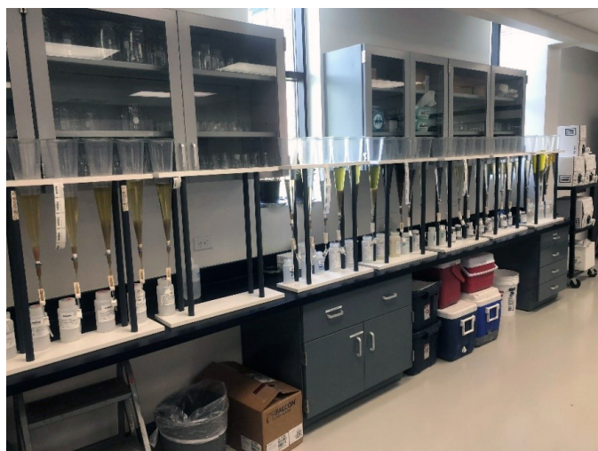
Imhoff settling cones containing invasive mussel early detection samples at the Reclamation Ecological Research Lab.
