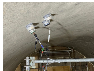
Electrochemical impedance spectroscopy test cell set-up for coating evaluation near pipe crown in a large diameter pipe.
