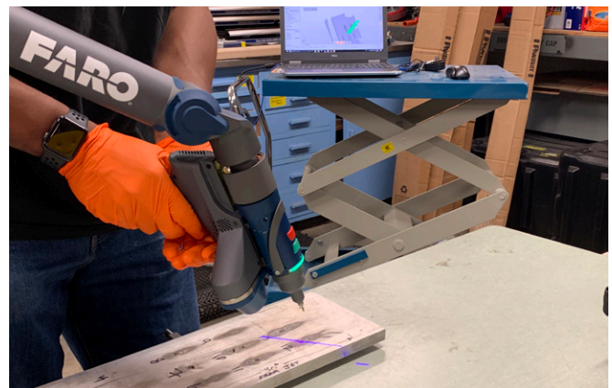
FARO LLP Scanning Cavitation Damage.
