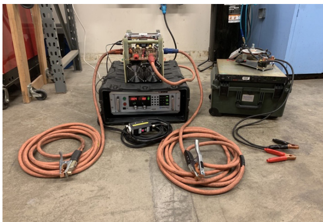
Electromagnetic rotor turner prototype consisting of two modified commercial power supplies and a lab-built current reversing module and handheld control box.
