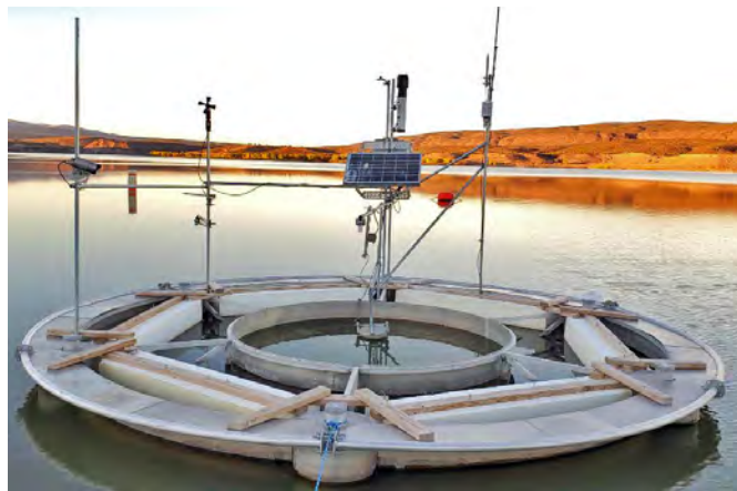
Final Version of the Collison Floating Evaporation Pan on Cochiti Lake, New Mexico.
