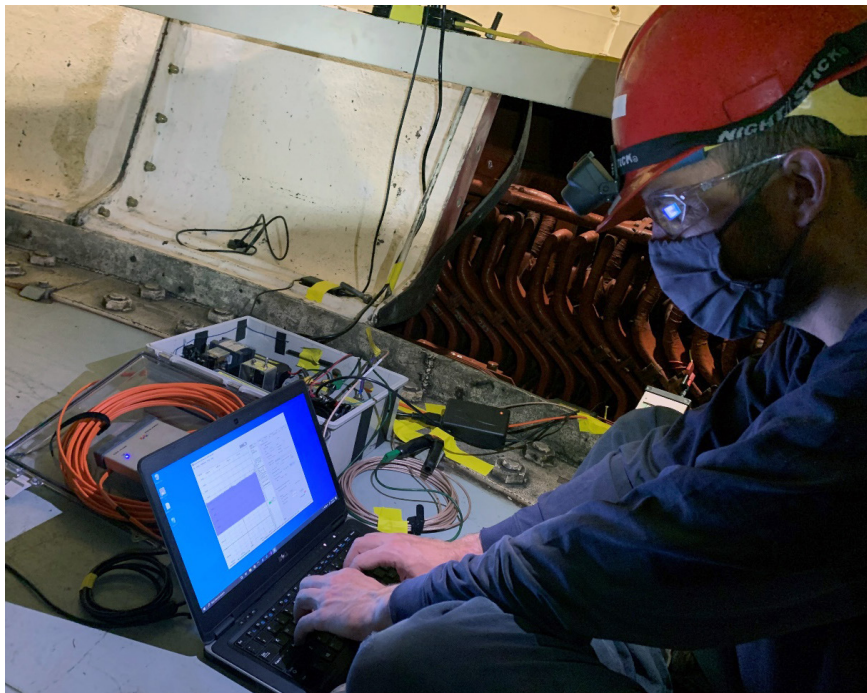
Researcher demonstrating the prototype system on the rotor of a hydro generator.
