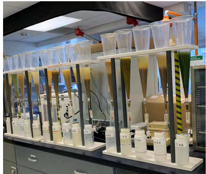
Water samples spiked with mussel veligers and settled in Imhoff cones to observe settlement efficiency.
