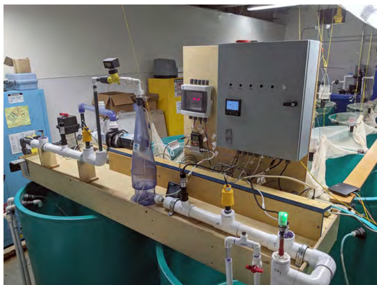
Speece Cone apparatus for the carbonation of raw water.
