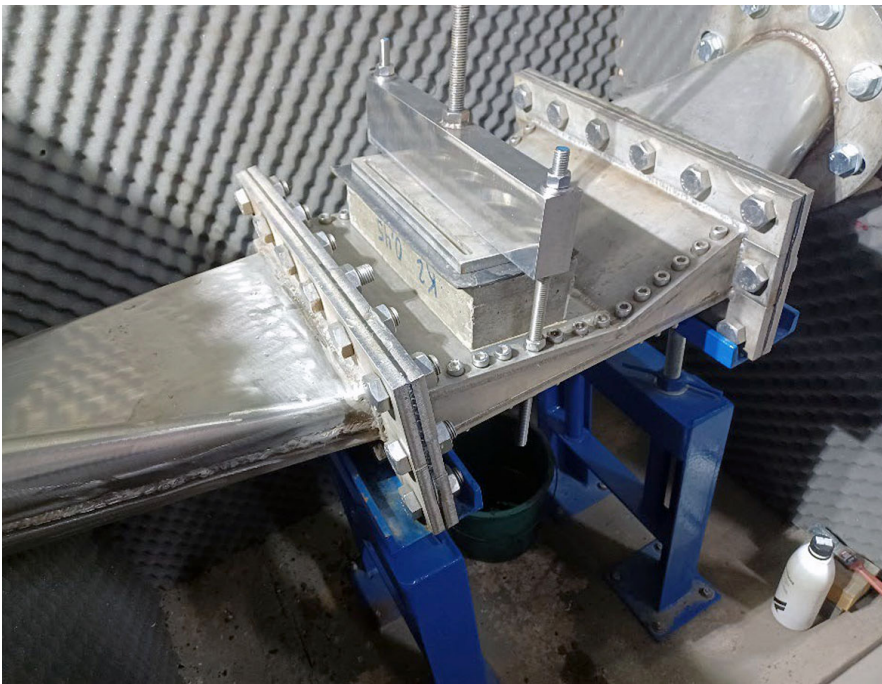
Cavitation machine at Federal University of Rio Grande do Sul (similar to Reclamation's) used to test durability of concrete to cavitation.
