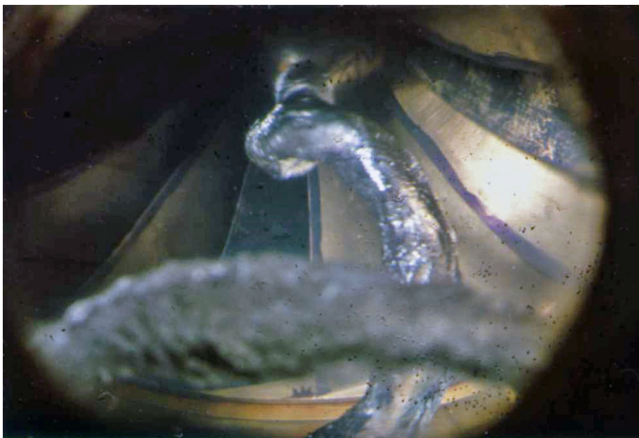
A cavitation vortex in a draft tube.
