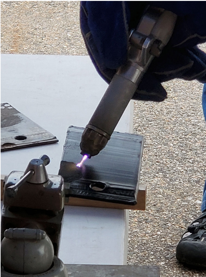
View of atmospheric plasma removing coal tar enamel from a test panel.
