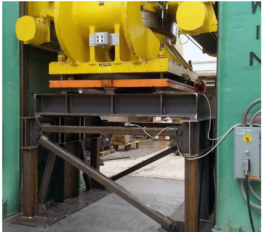
Experimental setup for the steel bulkhead gate.
