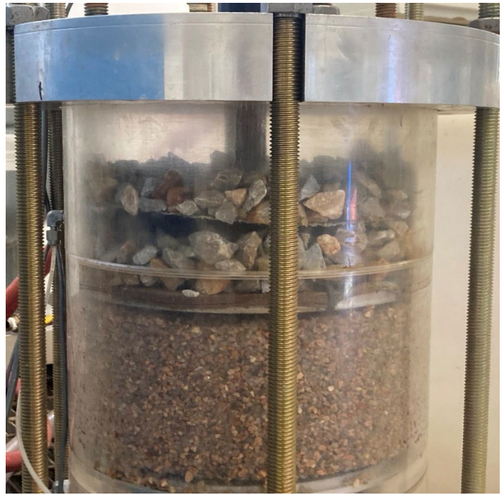
Soil specimen and setup for internal erosion analyses in a rigid cell permeameter.
