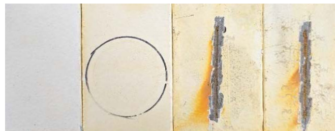
New polysiloxane coating system evaluated during laboratory corrosion testing.
