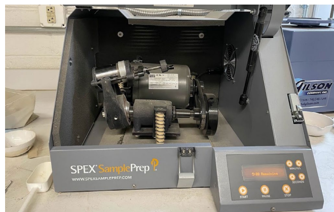
Ball mill device used to prepare samples for disaggregation analysis.
