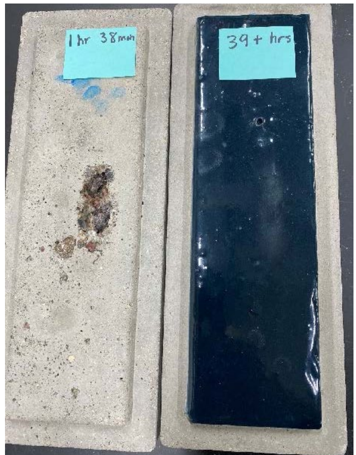
Bare concrete and a cavitation resistant coating after cavitation testing.
