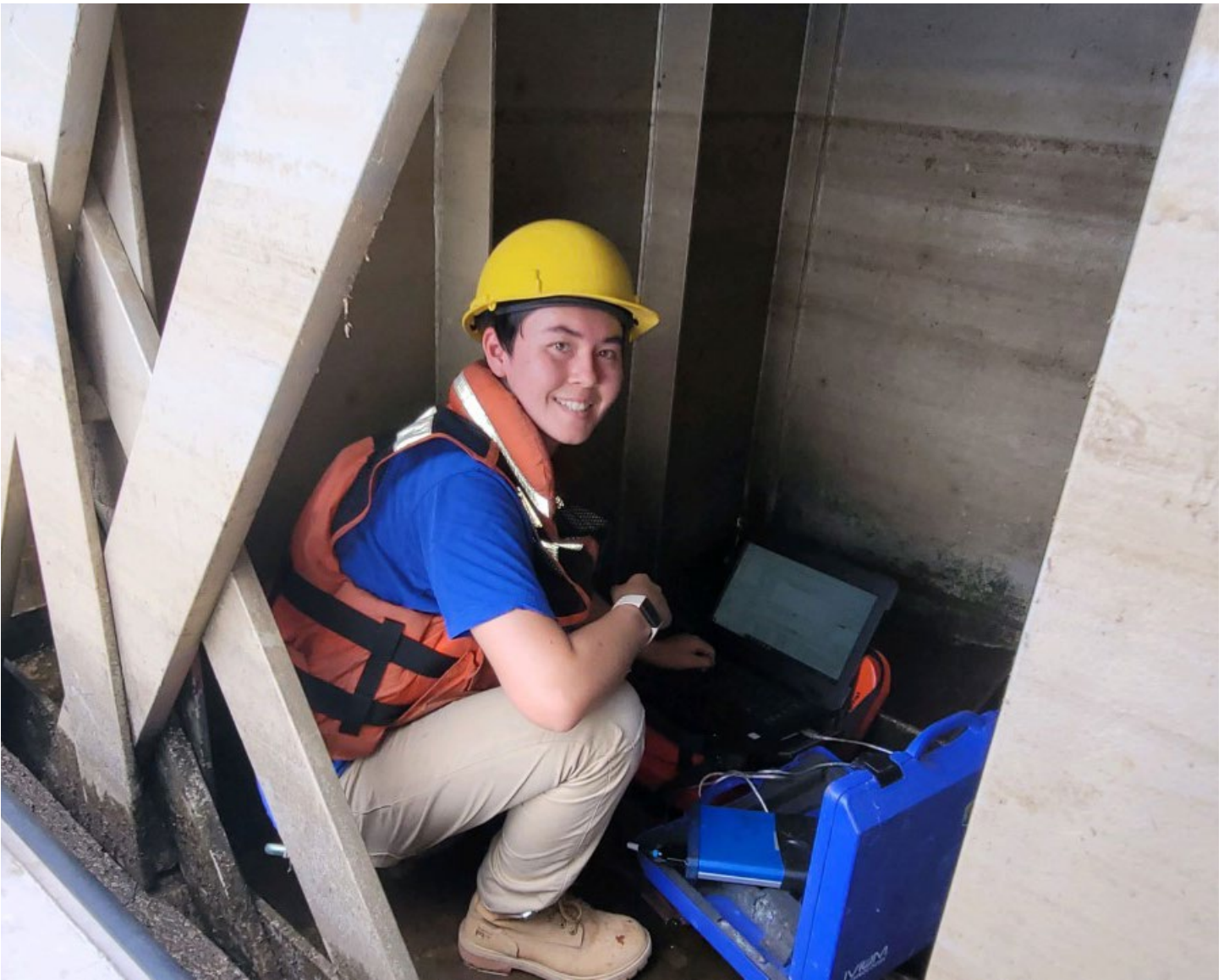
Researcher performing field electrochemical impedance spectroscopy testing on a vinyl-coated miter gate compartment at a U.S. Army Corps of Engineers facility.
