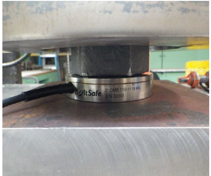
Laboratory testing of load-sensing washer in Denver, Colorado.
