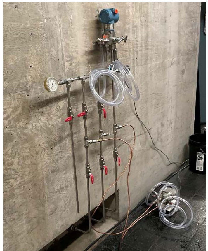
Winter-Kennedy flow meter during field testing.
