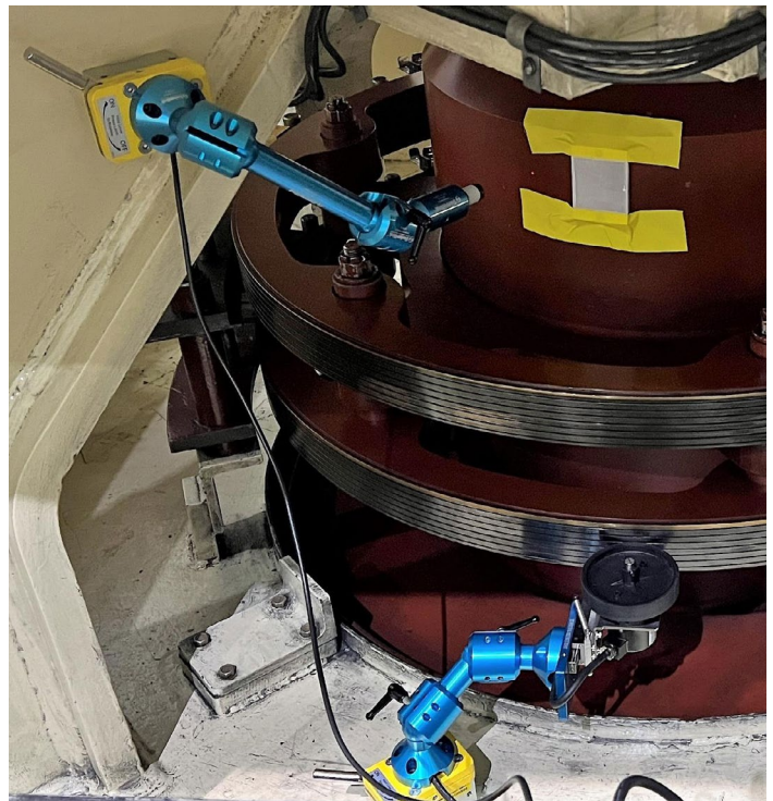
Encoder driven by rotor slip ring at bottom and revolution sensor and target at top.
