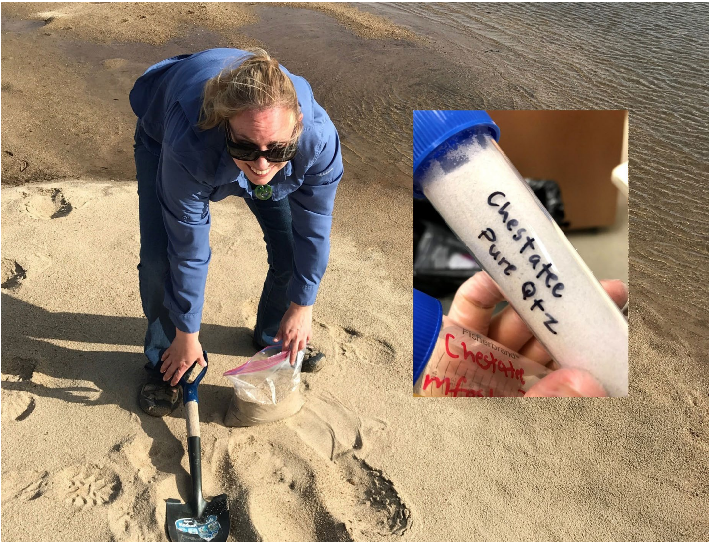
Sampling fresh sands on a river sand bar for Beryllium-10 testing to constrain millennial-scale basin erosion rates. Inset photo: Pure quartz obtained from river sands. Beryllium is isolated by further processing pure quartz.
