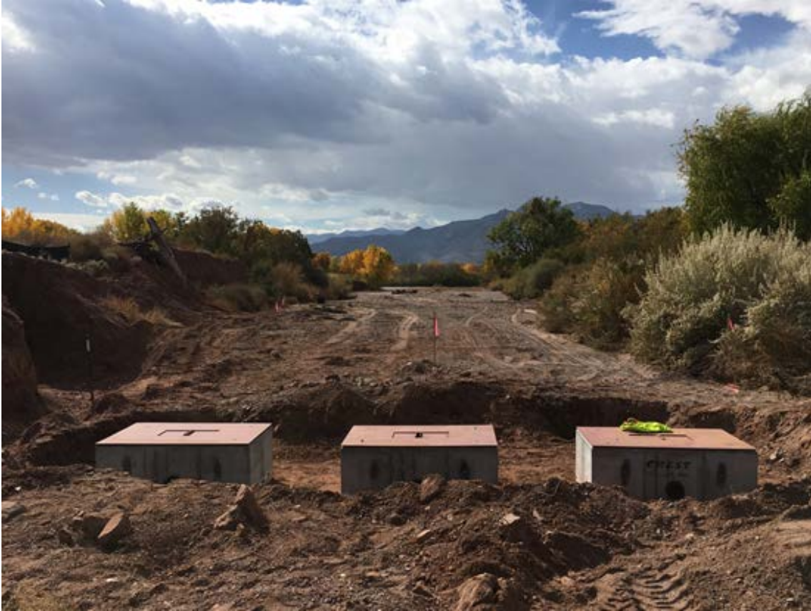
Figure 15. Research using Reid-type slot samplers to improve understanding of bed load transport rates on the ephemeral Arroyo de los Piños near Socorro, NM. Photograph courtesy of Kyle Stark, New Mexico Institute of Mining and Technology (Socorro, NM).
