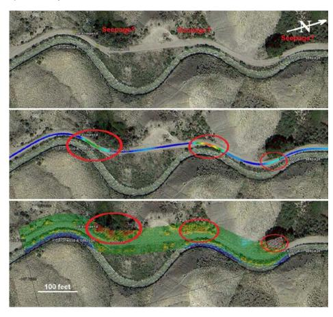
An example showing known and suspected canal seepage locations, and typical geophysical profiling anomalies and elevated NDVI values associated with these water losses that can be utilized to detect, map, and better characterize seepage.
