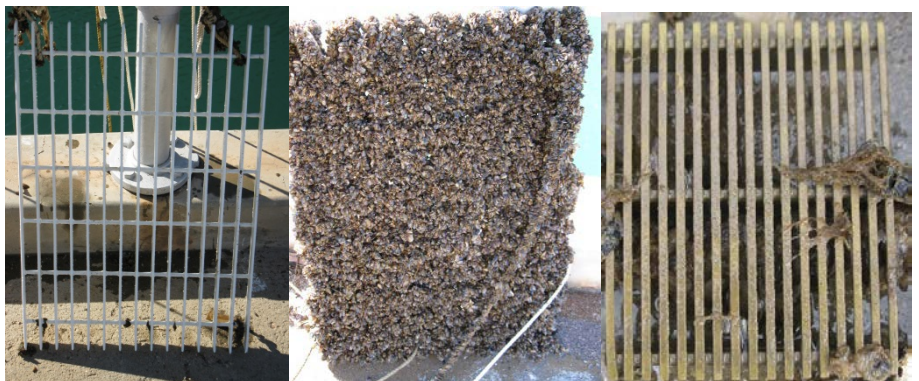
Left to right: Silicone foul release coating, steel, Z-alloy after 24 months of exposure.
