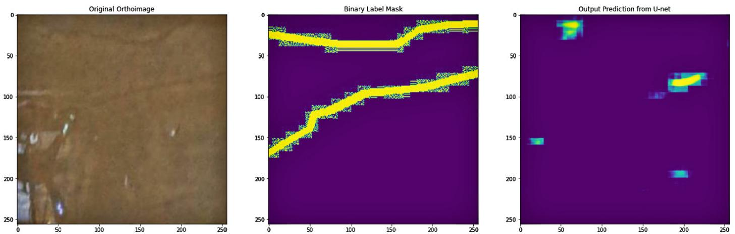
Example automatic crack mapping data set: input (left), label mask (center), and output prediction (right).
