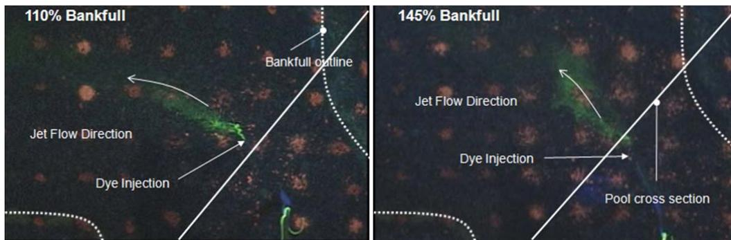
Figure 7. Dye tracer visualization of flow direction at 1.1 times and 1.45 times bankfull conditions, respectively.
