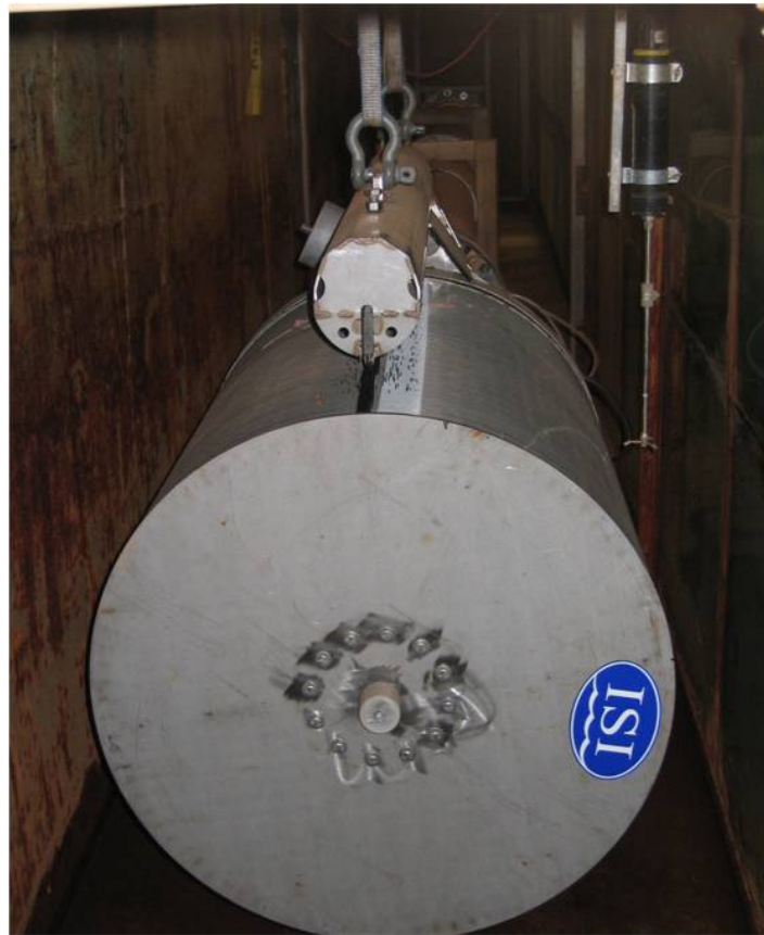
Figure 1. ISI hydraulically operated cylindrical screen inside test flume.
