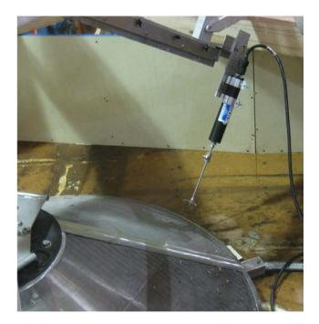
Figure 2. Sontek ADV probe test apparatus
