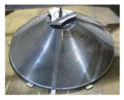
Figure 1. ISI Cone screen inside test flume. Note the 3 screen brushes have been removed.
