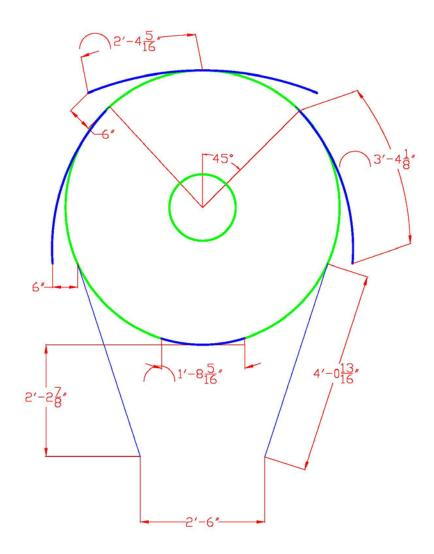
Figure 16. Details for final external bullnose Concept 2.
