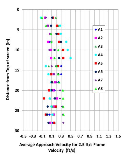
Figure 11. Bullnose Concept 2 - Cone Screen approach velocity profiles measured at locations A1 through A8.
