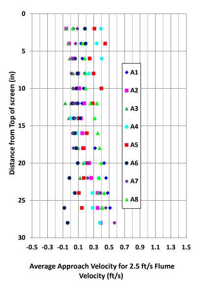
Figure 8. Bullnose Concept 1 - Cone screen approach velocity profiles measured at locations A1 through A8.
