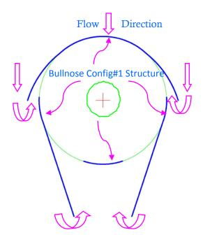
Figure 5. Illustration of Bullnose Concept 1. Blue lines indicate bullnose structure.
