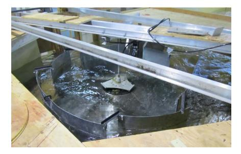
Figure 10. Photo of cone screen operating with Bullnose Concept 2.
