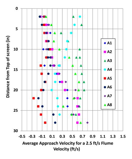
Figure 13. Bullnose Concept 3 - Cone Screen approach velocity profiles measured at locations A1 through A8.
