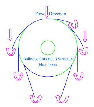
Figure 12. Illustration of Bullnose Concept 3. Blue lines indicate bullnose structure.
