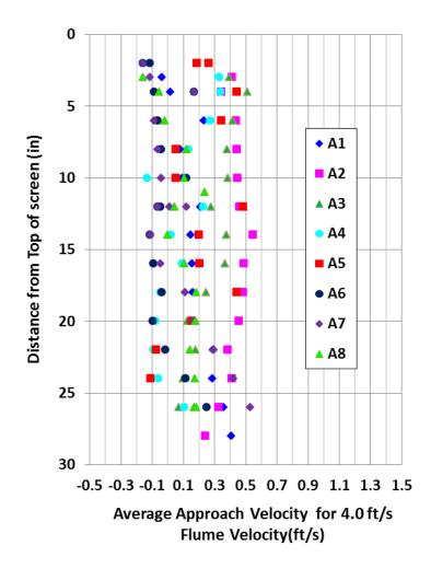
Figure 14. Bullnose Concept 2 and 4 ft/s flume velocity - Cone Screen approach velocity profiles measured at locations A1 through A8.
