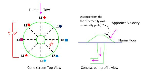
Figure 3. Velocity measurement locations for baseline condition and profile view of the screen setup.
