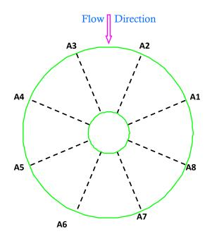
Figure 7. Velocity measurement locations for baffled (external and internal) cone screen.
