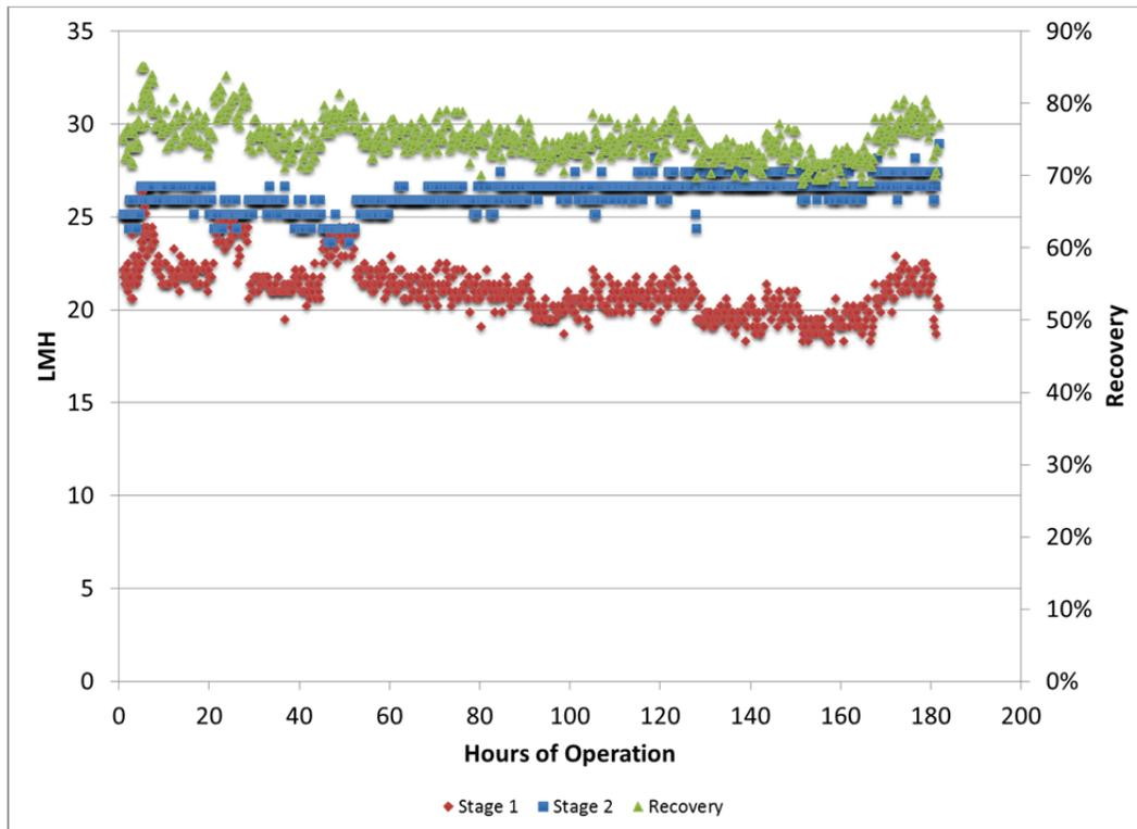
Figure 7-5. – Temperature normalized flux and recovery.
