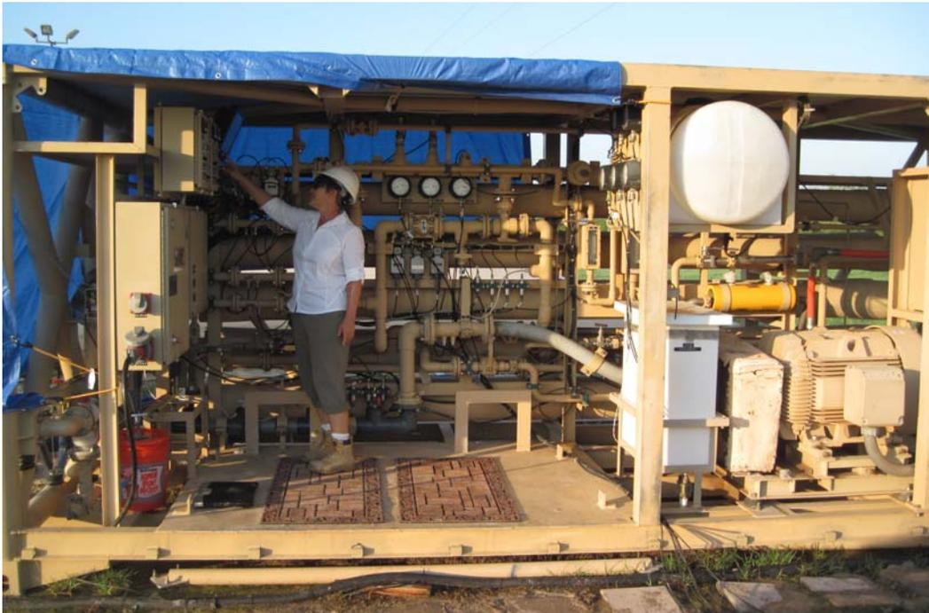
Figure 5-5. – RO skid and control center.
