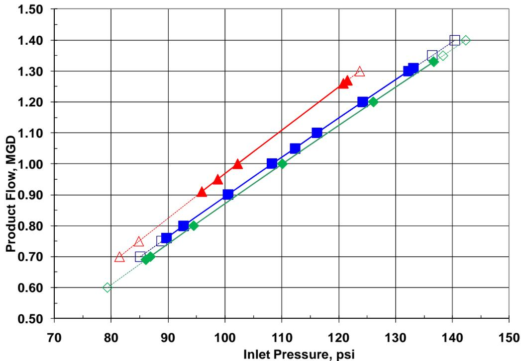
**Figure 2-1. – Relationship between product flow and inlet pressure.**
