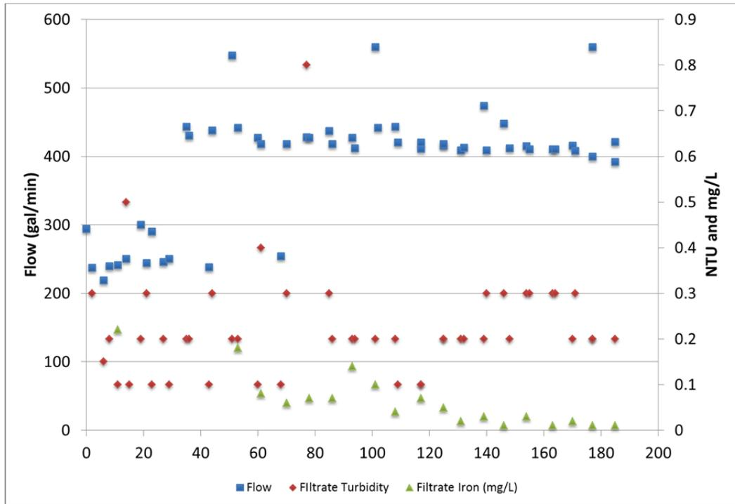
Figure 7-1. – UF system flow and filtrate quality.
