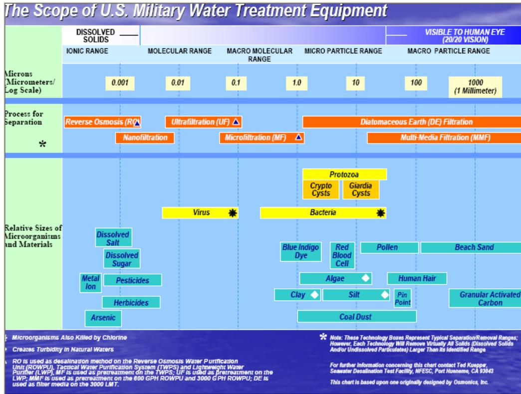
Figure 5-1. – Filtration spectrum. Pretreatment/Suspended Solids Filtration
