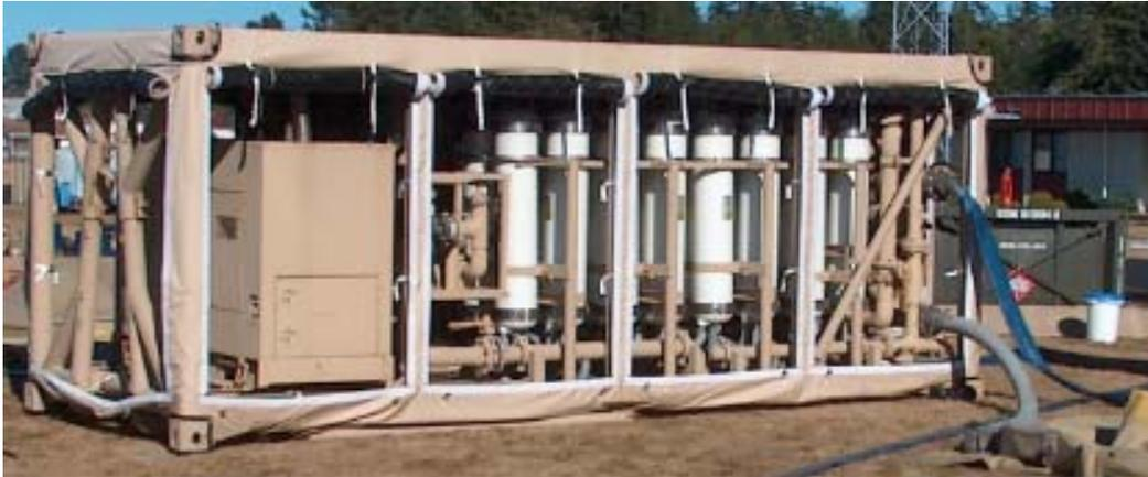
Figure 5-4. – Photo of the UF skid.
