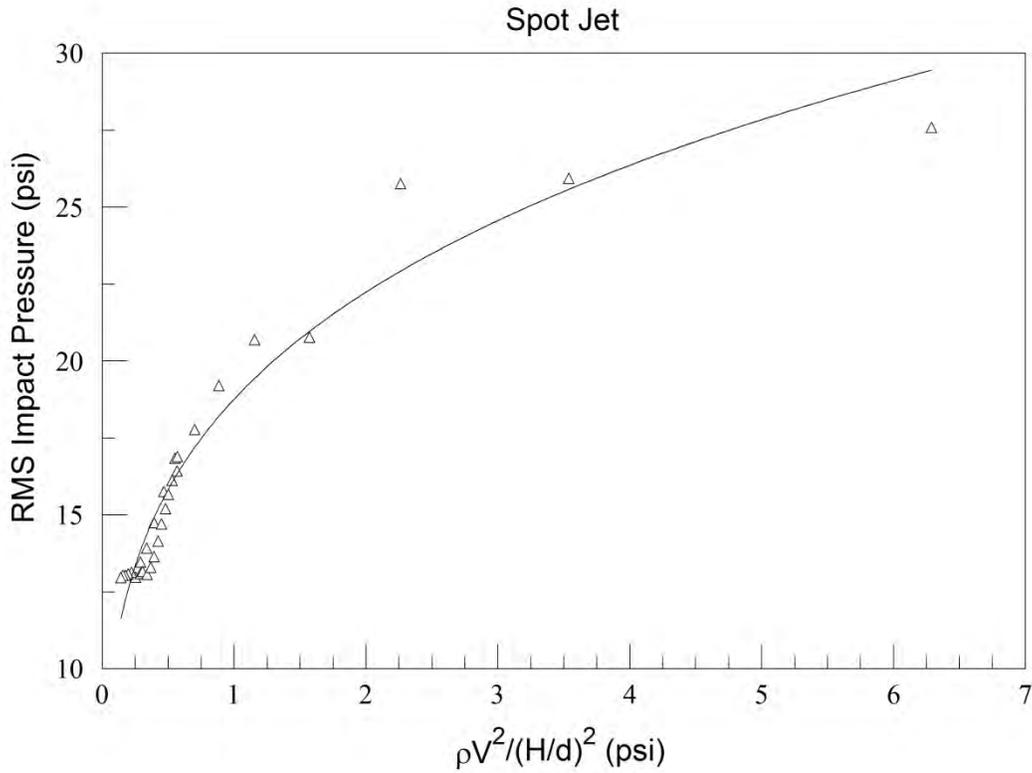
Figure 9 Impact pressure results for a spot jet set perpendicular to the surface for durability testing. For this data set  $R^2 = 0.943$ .
