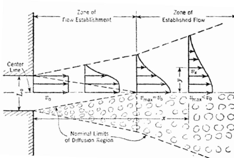
Figure 1 Schematic showing zones of submerged jet flow, from Albertson *et al* (1948)
