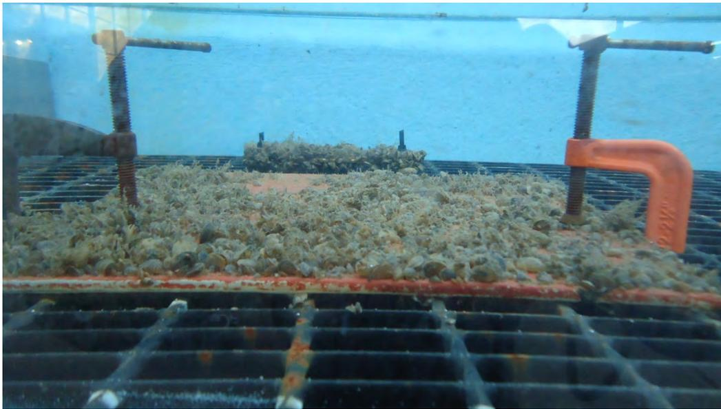
Figure 16 Seaspeed sample with live quagga mussels attached prior to testing for release pressures.
