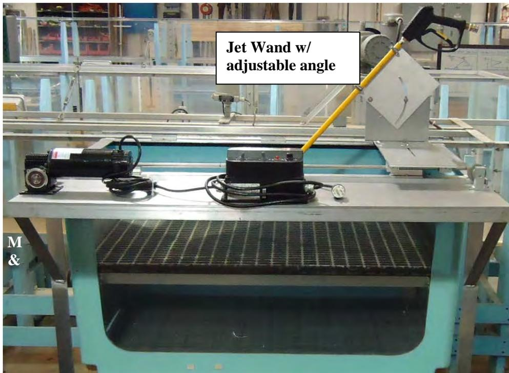
Figure 2 Test apparatus used for coating durability and mussel release testing in both the laboratory and the field.
