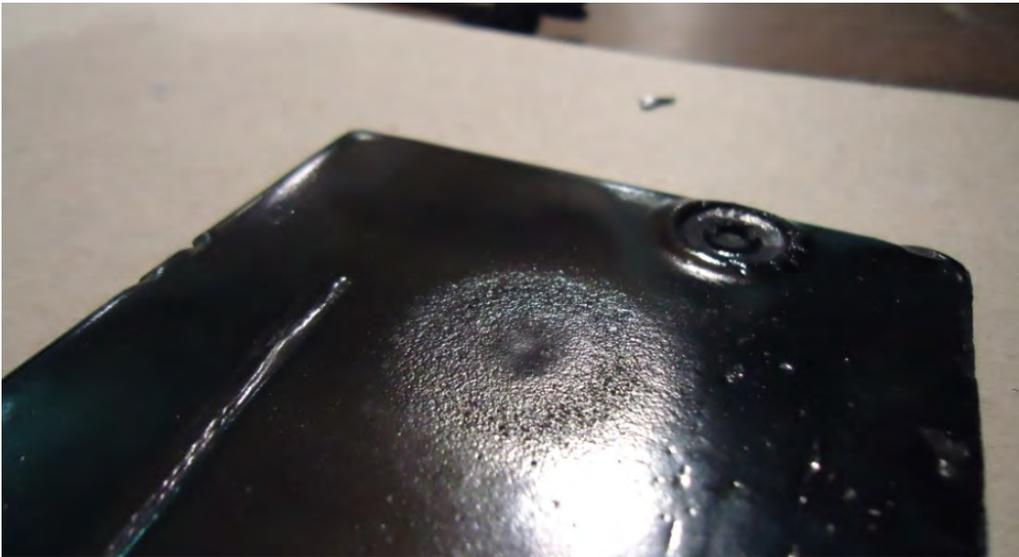
Figure 11 Photo of Coal Tar Enamel sample after durability testing. The center of the jet caused a small hole to form surrounded by cavitation pitting.
