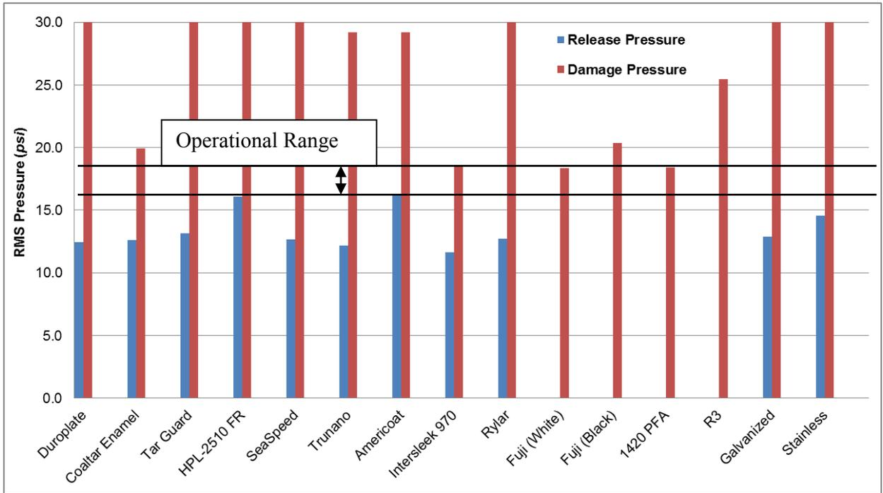
Figure 19 Average RMS impact pressure results for both mussel removal and coating damage.
