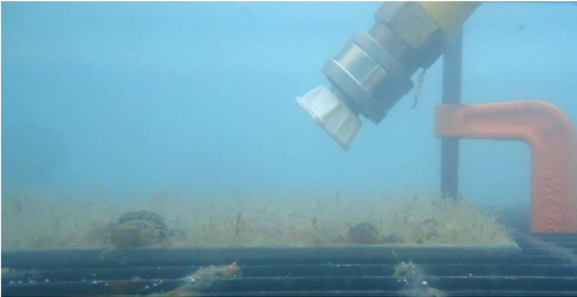
Figure 8 40° fan jet at a 45° angle used for release pressure testing in field tests with live quagga mussels.
