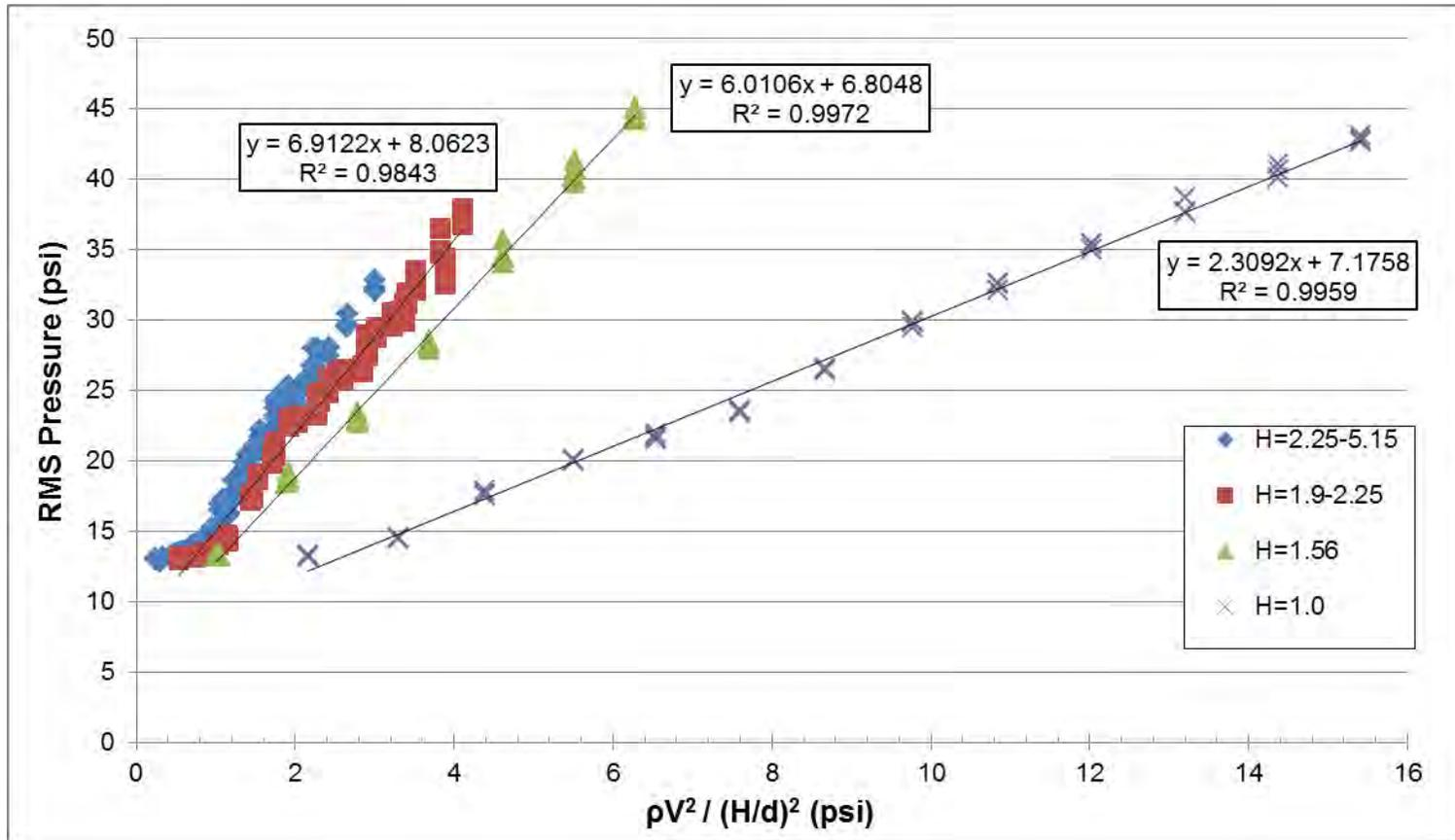
Figure 20 Fan Jet data sets for nozzle distances less than 2.25 inches. Equations on plot were used for pressure predictions for mussel removal data for close nozzle distances. Additional testing may be necessary for gaps in data (ex.  $H < 1.0$  inch or  $1.0 < H < 1.56$  inches).
