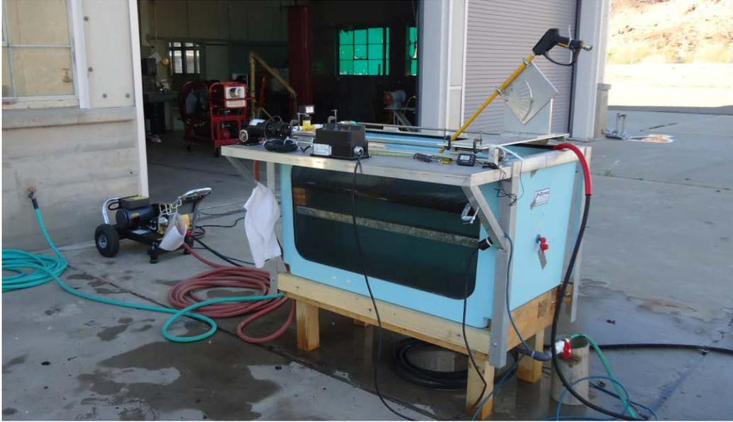
Figure 7 Test apparatus used for initial mussel removal testing at Parker Dam December 2011.
