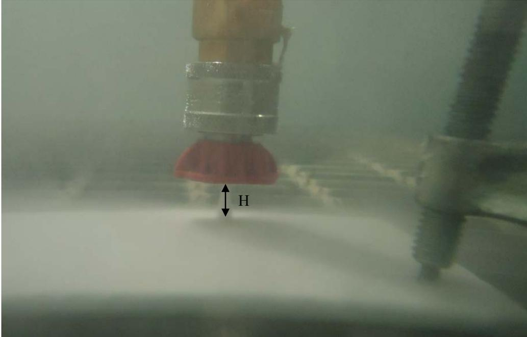
Figure 6 Spot jet used for durability pressure testing.
