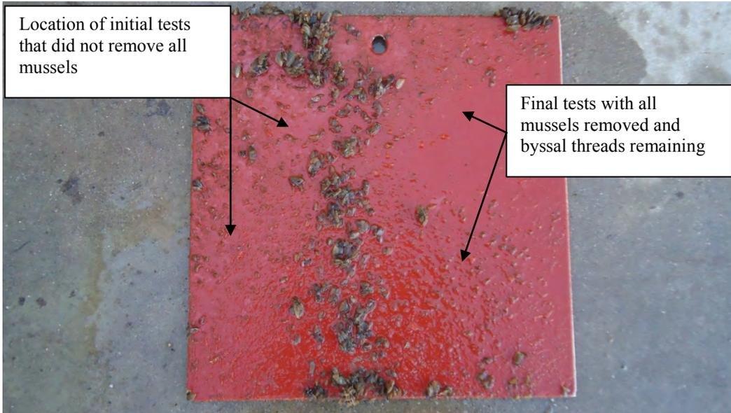
Figure 17 Seaspeed sample after release pressure testing. Mussels are removed where the proper jet distance and velocity were found (right side) but byssal threads remain on the plate.
