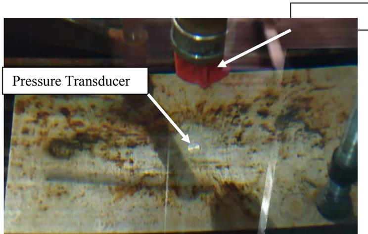
Figure 5 Piezometric pressure transducer set flush with the surface boundary used for impact pressure testing.
