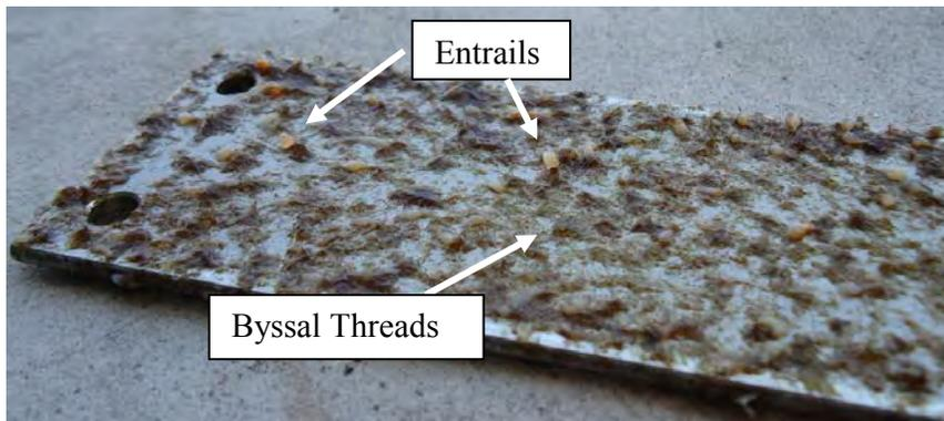
Figure 15 Byssal threads and entrails of mussels that were removed from a stainless steel plate during water jetting.
