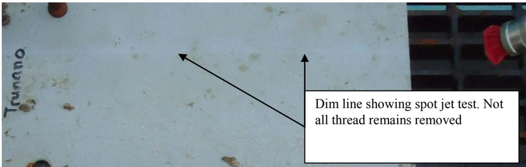
Figure 18 Attempt to remove byssal thread remains using a spot jet ½ inch from surface.
