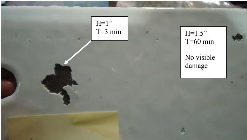
Figure 14 R3 sample; visible damage of coating peeled of test plate after 3 minute test. No damage was observed from 60 minute test with distance of 1.5 inches.
