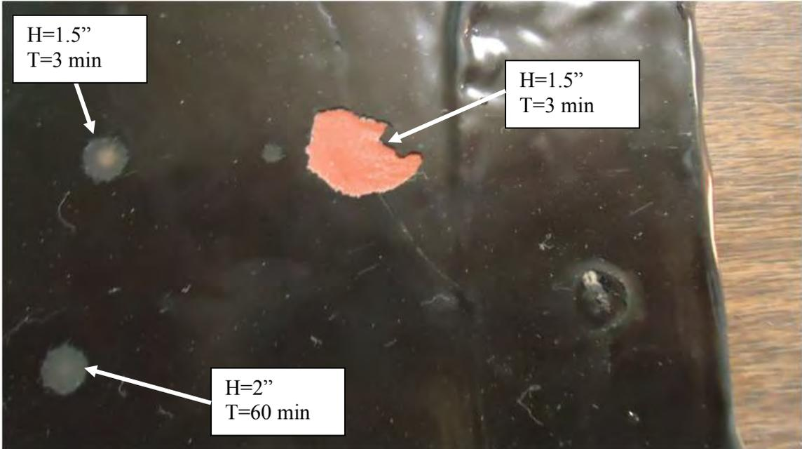
Figure 12 Fuji test sample; visible damage from 3 minute and 60 minute tests.
