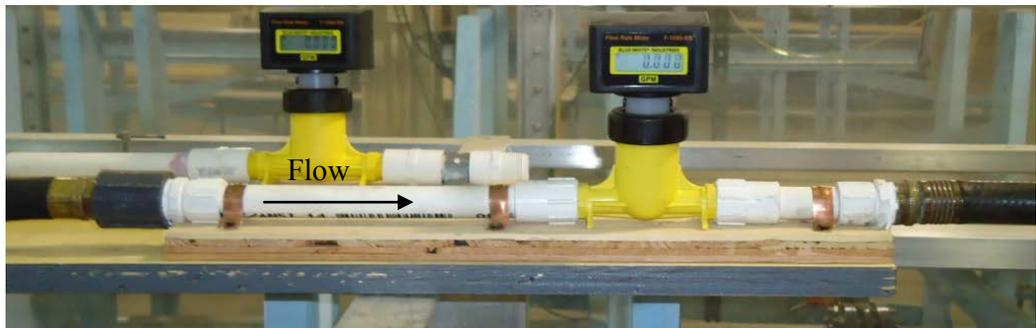
Figure 4 Inline propeller flow meter used to measure flow and estimate nozzle jet velocity.
