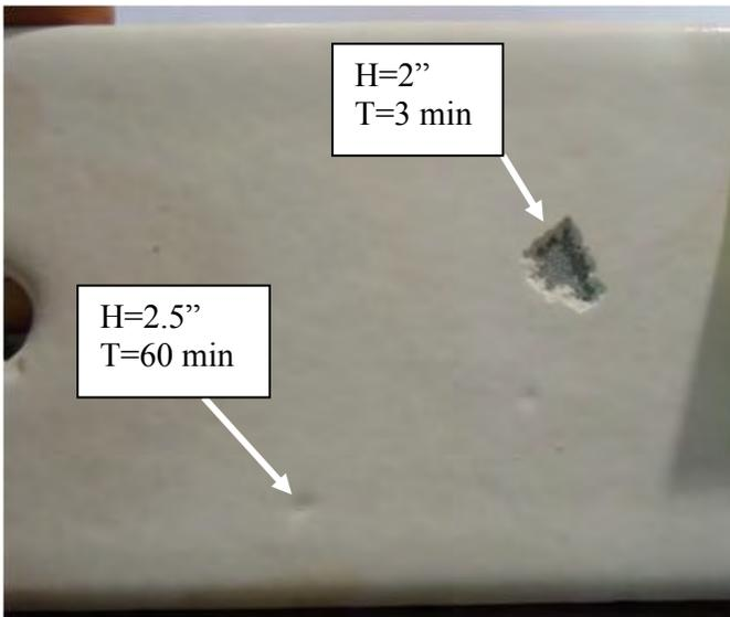
Figure 13 1420 PFA test sample; chunk removed from 3 minute test and slight dent (no damage) from 60 minute test.
