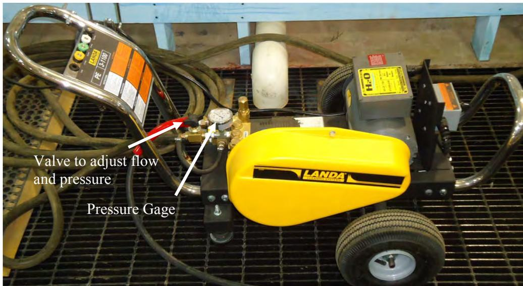
Figure 3 Landa pressure pump used to create water jets for coatings testing.
