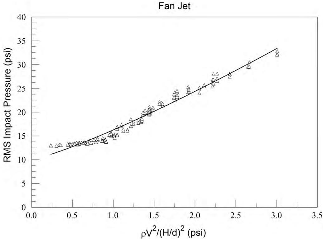
Figure 10 Impact pressure results for a 40 degree fan jet set at 45 degrees to the surface for release pressure testing. For this data set  $R^2 = 0.972$ .
