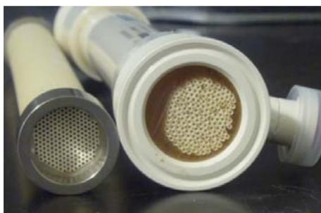
**Figure 4.1 End view of alumina (left) and PES (right) modules.**
