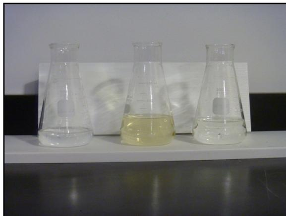
**Figure 7.1 Color of the filtrate during caustic cleaning (pH 11, 400 ppm NaOCl); initial (left); after 4 minutes (middle); after 5 minutes (right).**
