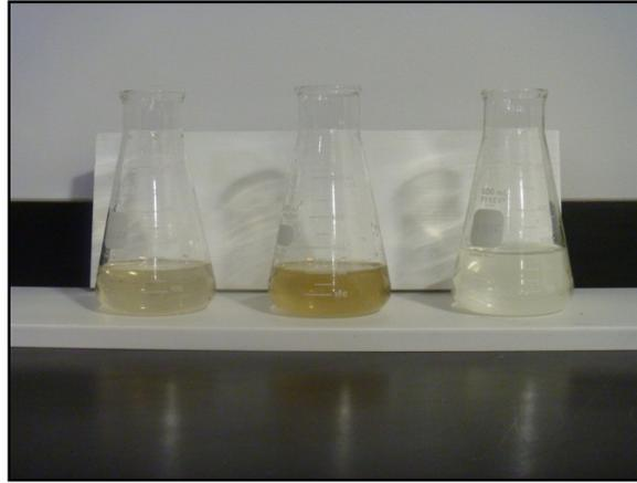
**Figure 7.2 Backwash effluent after 1 minute (left), 4 minutes (middle), and 5 minutes (right); color evolution indicates complete cleaning has been accomplished.**
