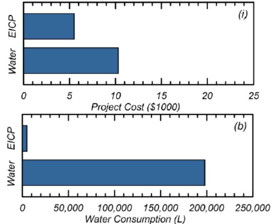
Pictured above: Results from a life cycle analysis in 2019 that compared EICP to water application for dust control for a 1-acre treatment area over a 2-week period.
