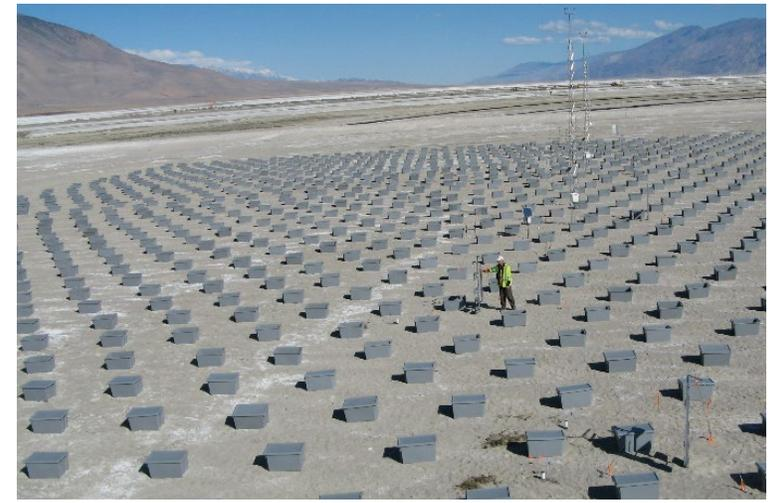
Engineered solid roughness elements test at Owens Lake
