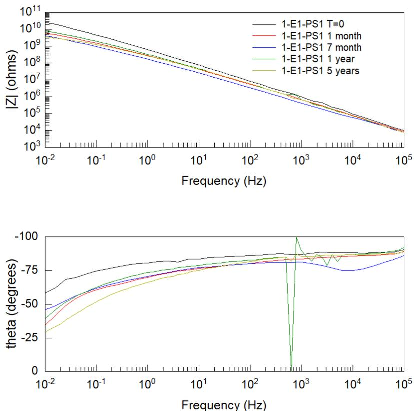
Figure 3. Bode plot for polysiloxane system 1-E1-PS1, exposure time is 5 years.
