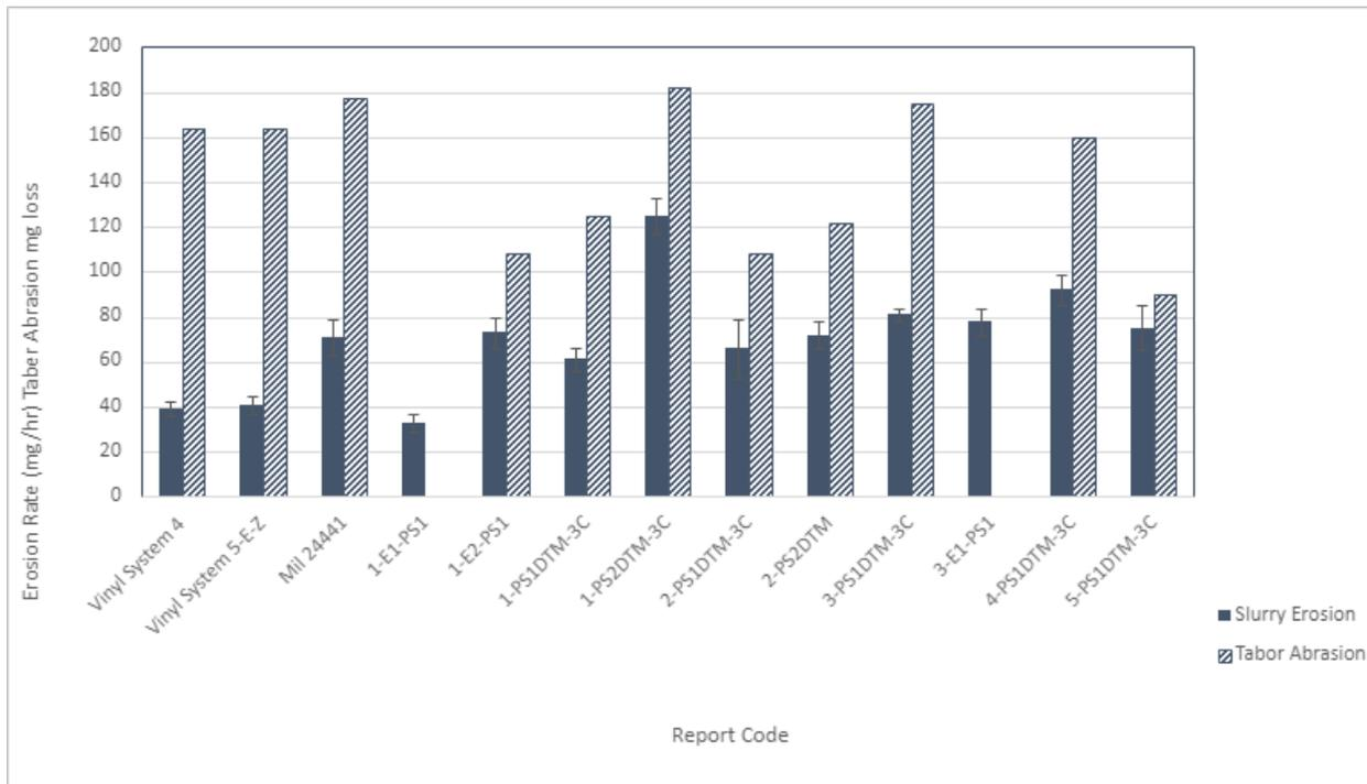
Figure 17. Erosion and abrasion test results. Error bars are included for the slurry erosion results.
