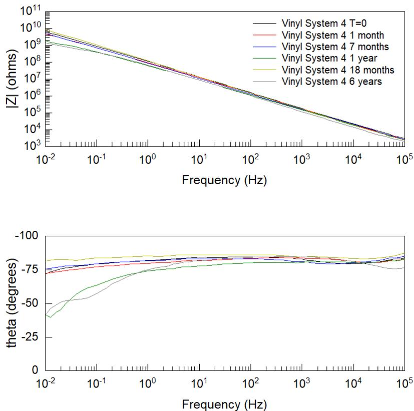
Figure 1. EIS data presented as Bode plot for vinyl system 4, exposure time is 6 years. The impedance magnitude is stable and stays above  $1 \times 10^9$  ohms, and phase angle stays below -45 degrees.
