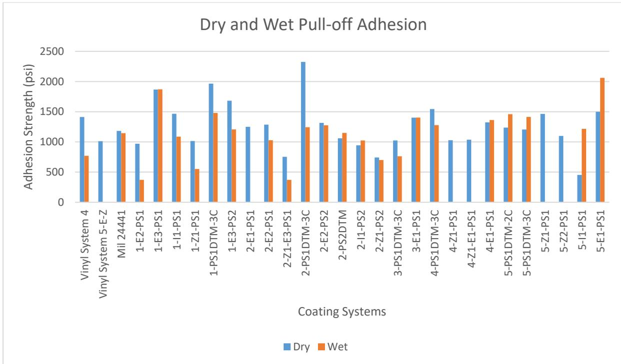
Figure 19. Average pull-off strength (psi) for dry and wet adhesion test results.
