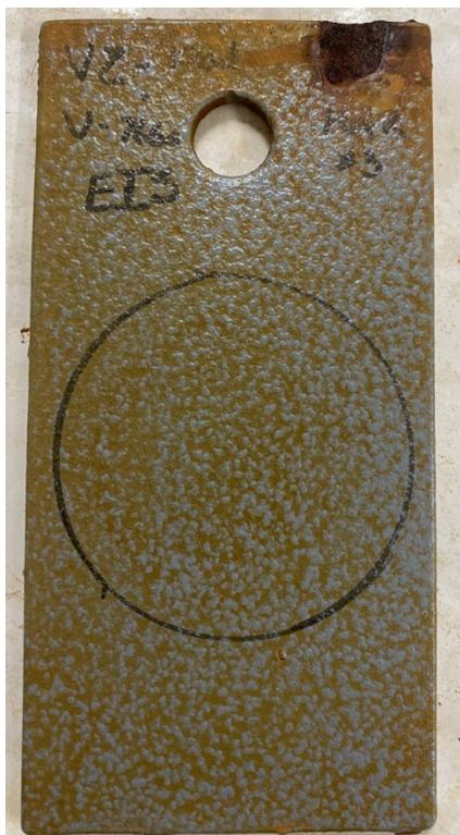
Figure 7: Vinyl System 5-E-Z after six years of immersion testing. Textured surface is possibly due to zinc pigments reacting to form zinc oxide and zinc hydroxide.
