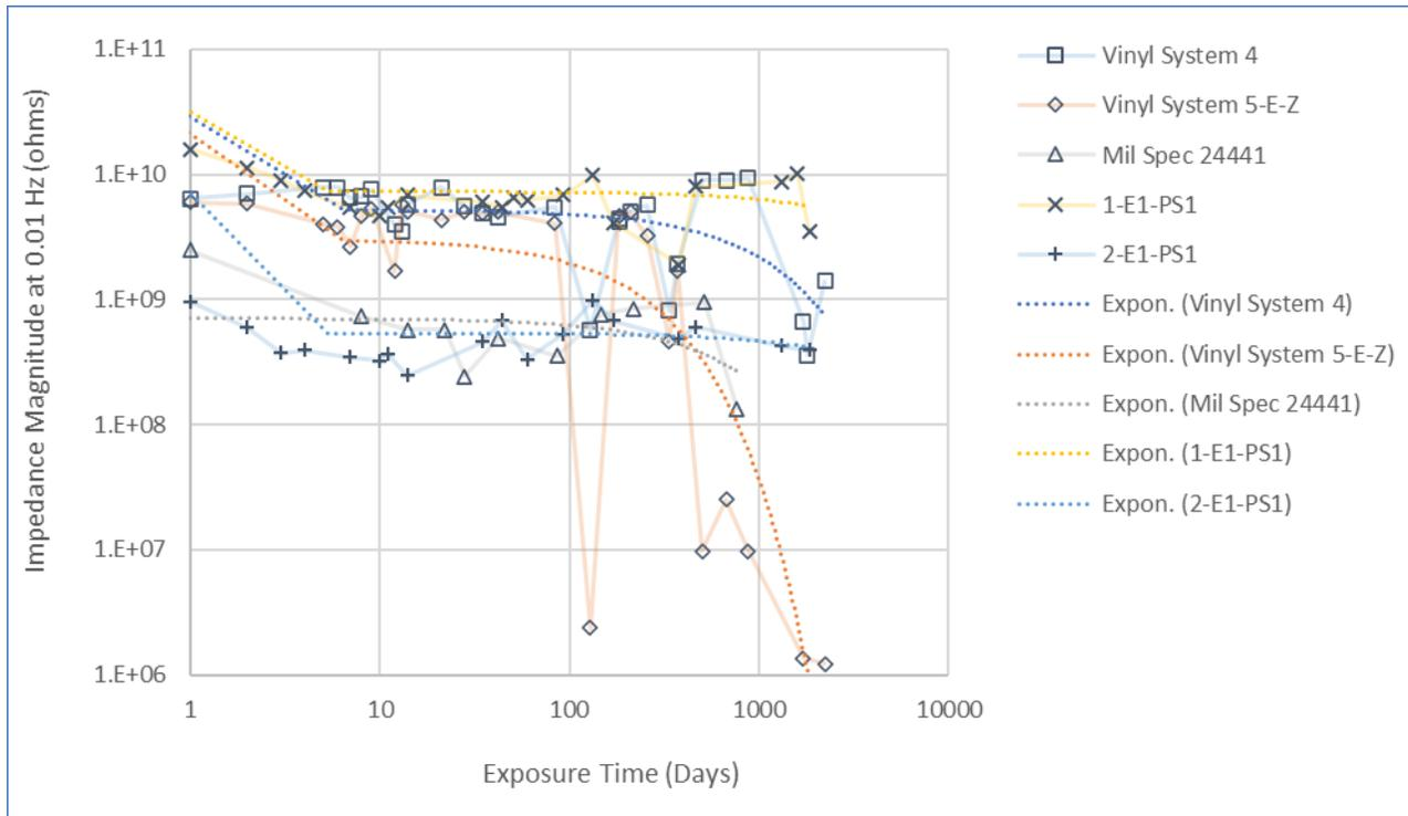
Figure 6. EIS plot of low frequency impedance at 0.01Hz vs. exposure time. An exponential trend line was fitted for each coating system. Notice Vinyl System 5-E-Z significantly drops in EIS magnitude after 1.5 years (about 500 days) in immersion.
