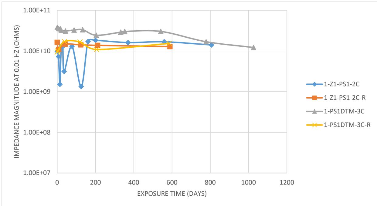
Figure 20: EIS impedance at 0.01 Hz over time for reproducibility study.
