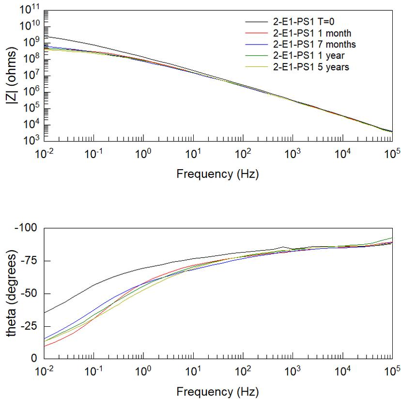
Figure 5. Bode plot for polysiloxane system 2-E1-PS1, exposure time is 5 years.
