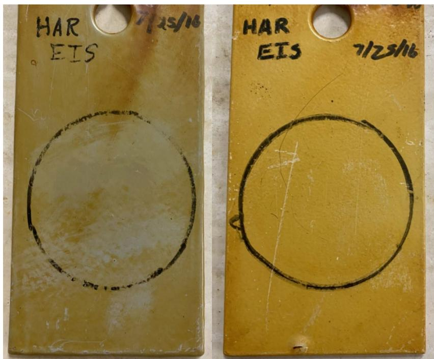
Figure 9. System 1-E1-PS1 (Left) and system 2-E1-PS1 (Right) after five years immersion testing. Notice one small blister on the bottom of the panel of system 2-E1-PS1.
