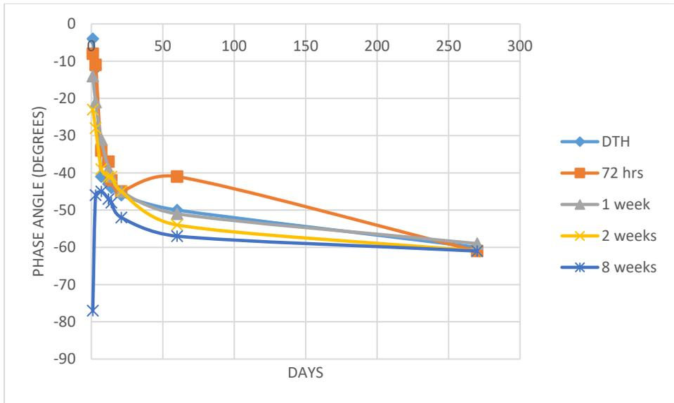
Figure 30: Phase angle of all cure durations during the evaluation period. The initial phase angles are different for all cure durations, but all converge to approximately -60 degrees after 250 days showing pseudo capacitive behavior.
