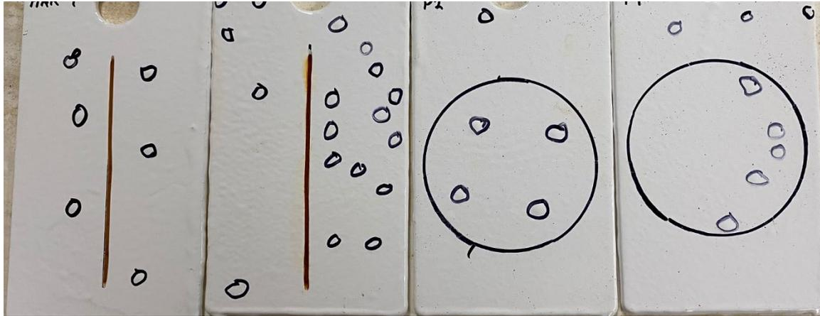
Figure 10. Polysiloxane system 5-Z1-PS1 after 1 month in HAR water immersion. The black circles show the blister locations.
