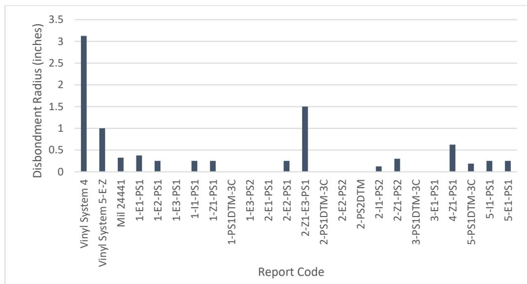
Figure 16. Cathodic disbondment result showing that most polysiloxanes perform similar to the Mil 24441 control and better than the vinyl systems. Three systems were not tested due to blistering in water immersion prior to the cathodic disbondment test and were withdrawn, and four systems had blisters or cracking.
