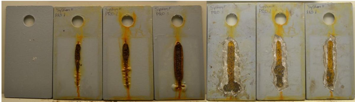
Figure 12. PRO cyclic test of vinyl system 5-E-Z; (left) before scraping (right) after scraping away coating.
