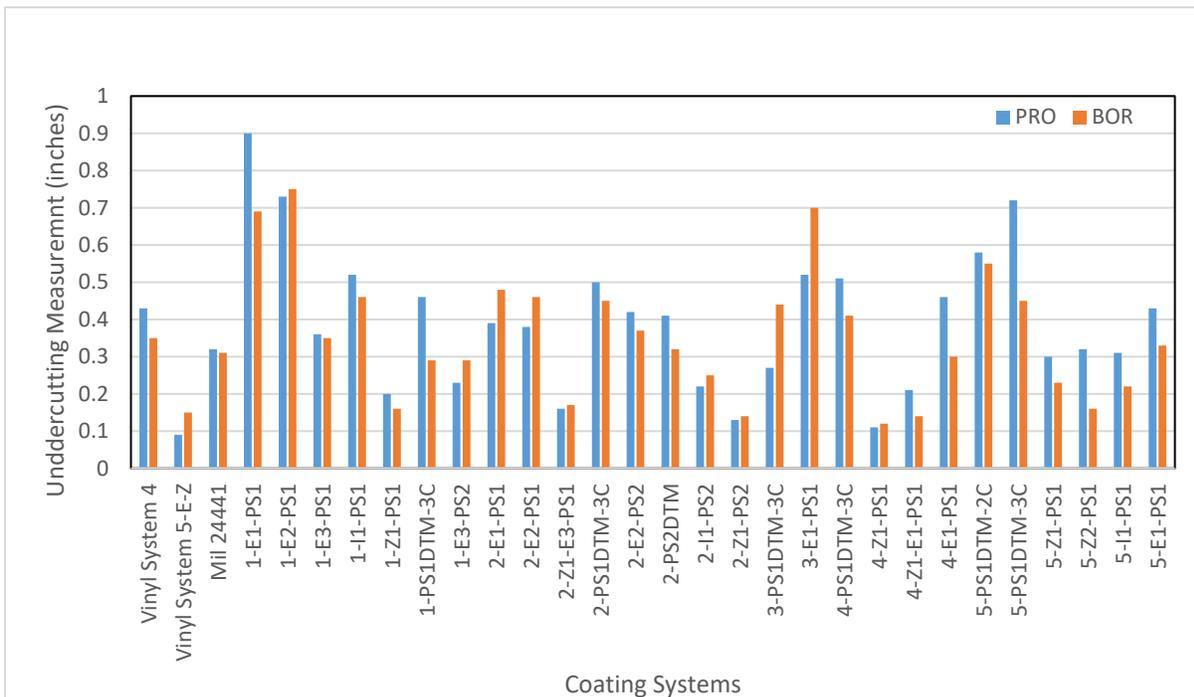
Figure 11: Undercutting results for all polysiloxanes and controls in cyclic testing.
