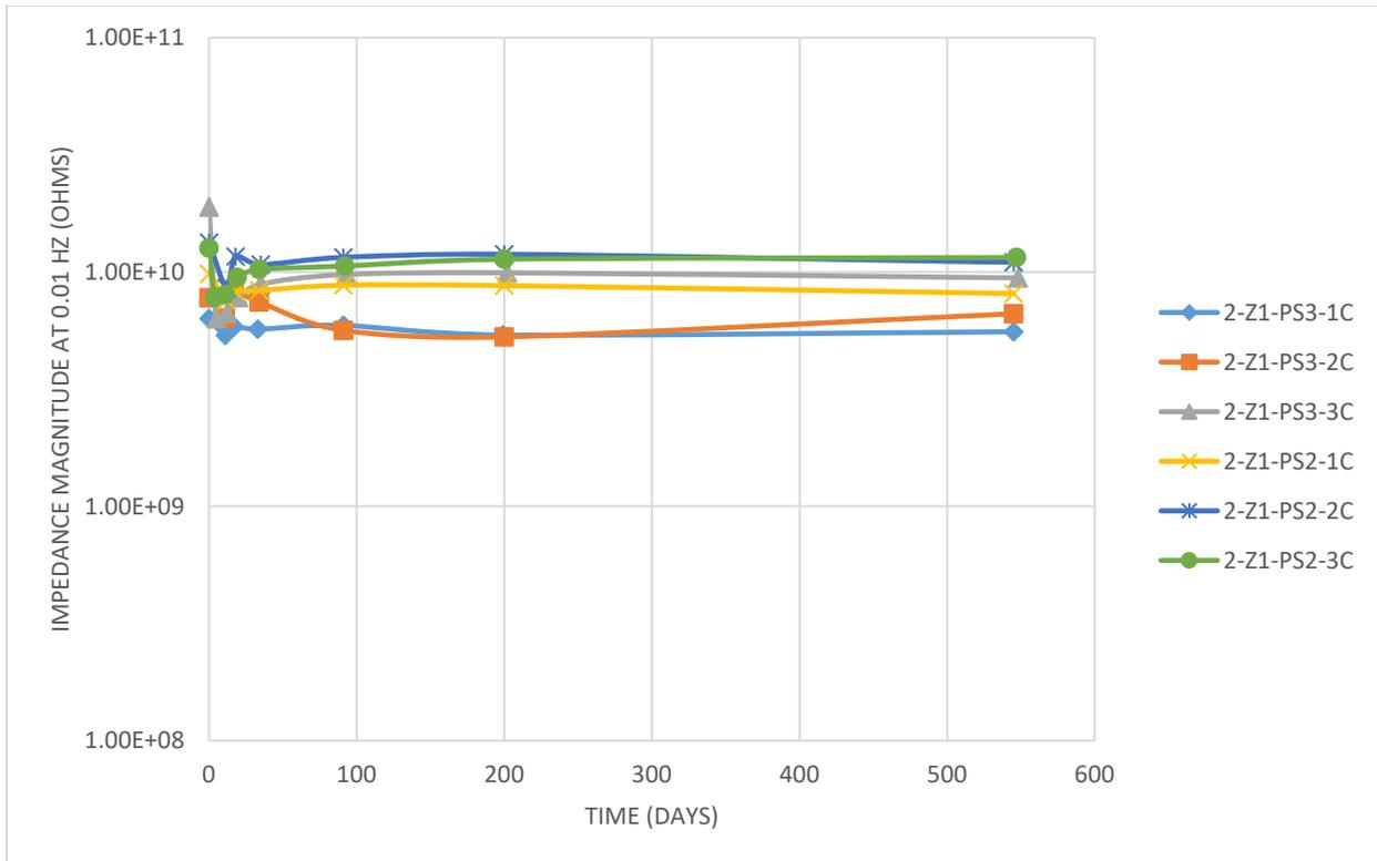
Figure 25: EIS results at 0.01 Hz for 2-Z1-PS2 coating systems. As the number of coats increases the overall impedance of the system increases.
