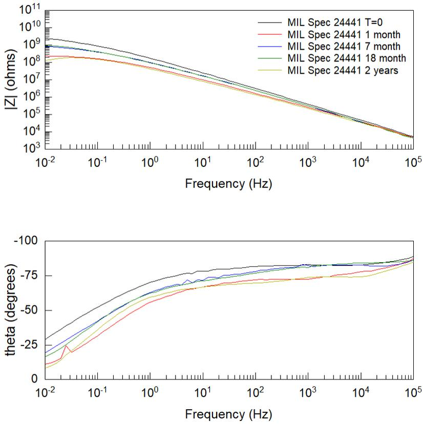
Figure 4. Bode plot for Mil Spec 24441 epoxy, exposure time is 2 years.
