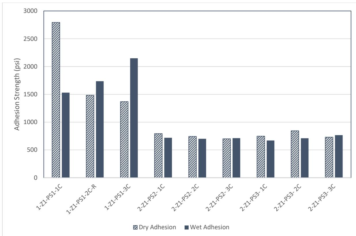
Figure 28: Average dry and wet pull-off adhesion results for two, three, and four coat system study.
