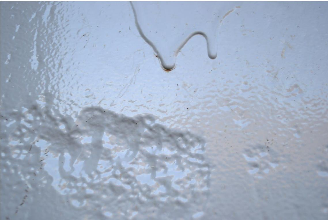
Figure 32: Large drip from application. Pitted area of steel with no defects to the coating or corrosion observed.
