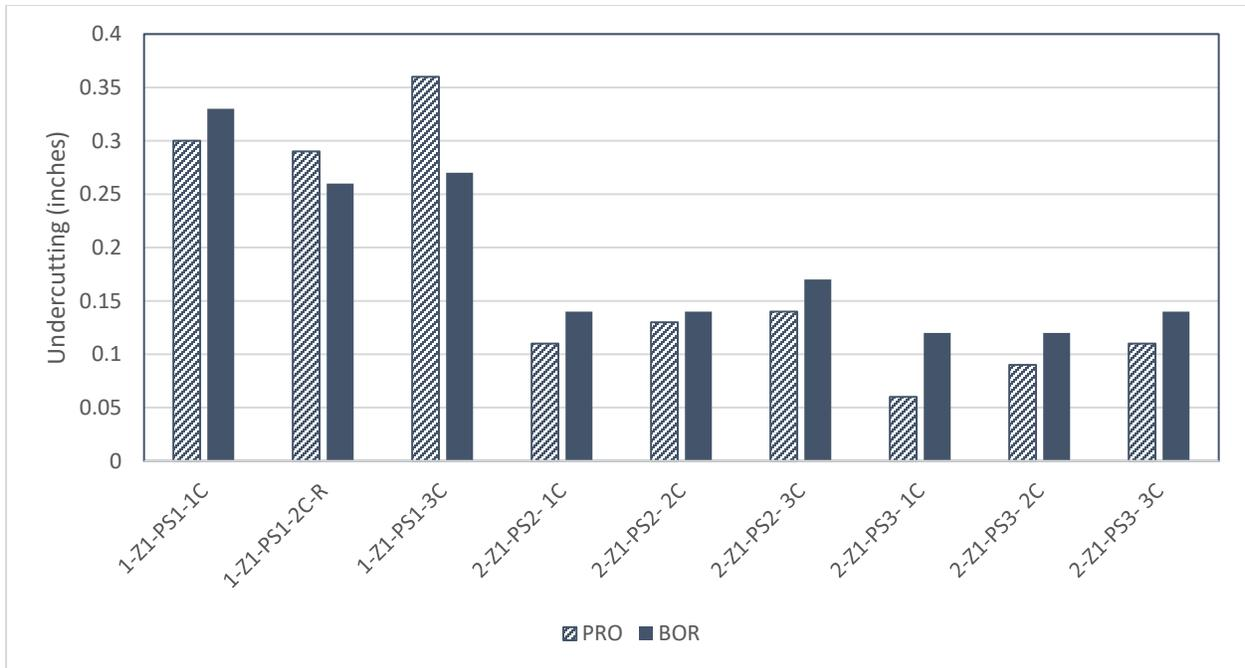
Figure 26: Cyclic test results showing the PRO and BOR undercutting resistance for two, three, and four coat systems.
