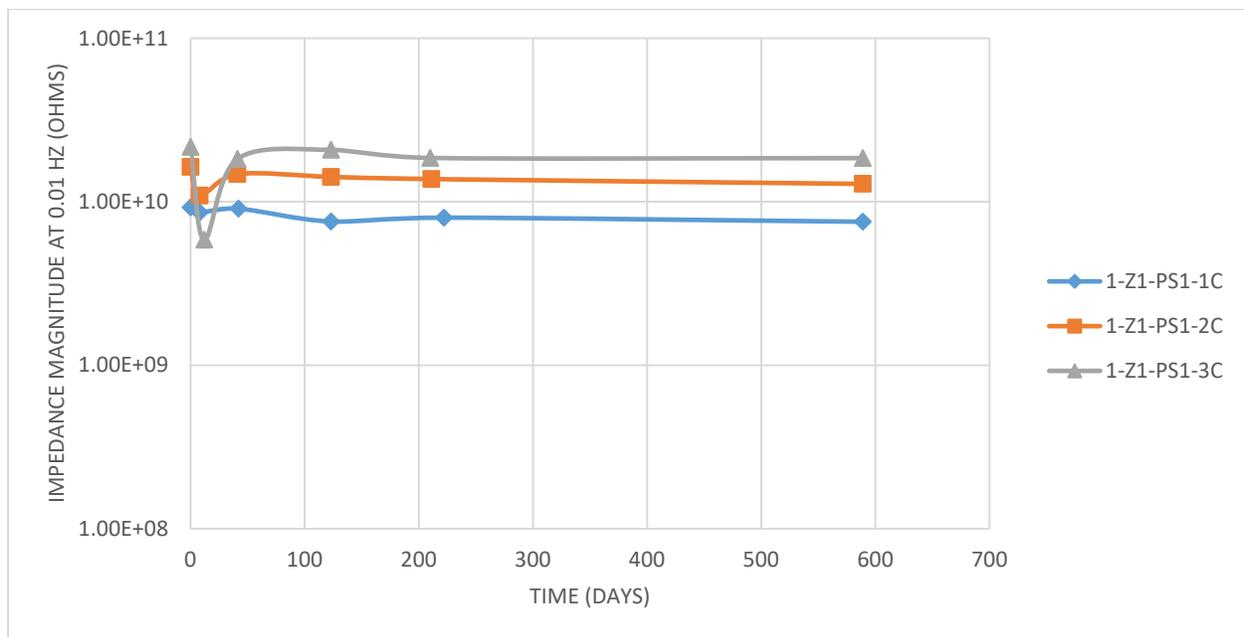
Figure 24: EIS results at 0.01 Hz for 1-Z1-PS1 coating systems. As the number of coats increases so does the impedance.
