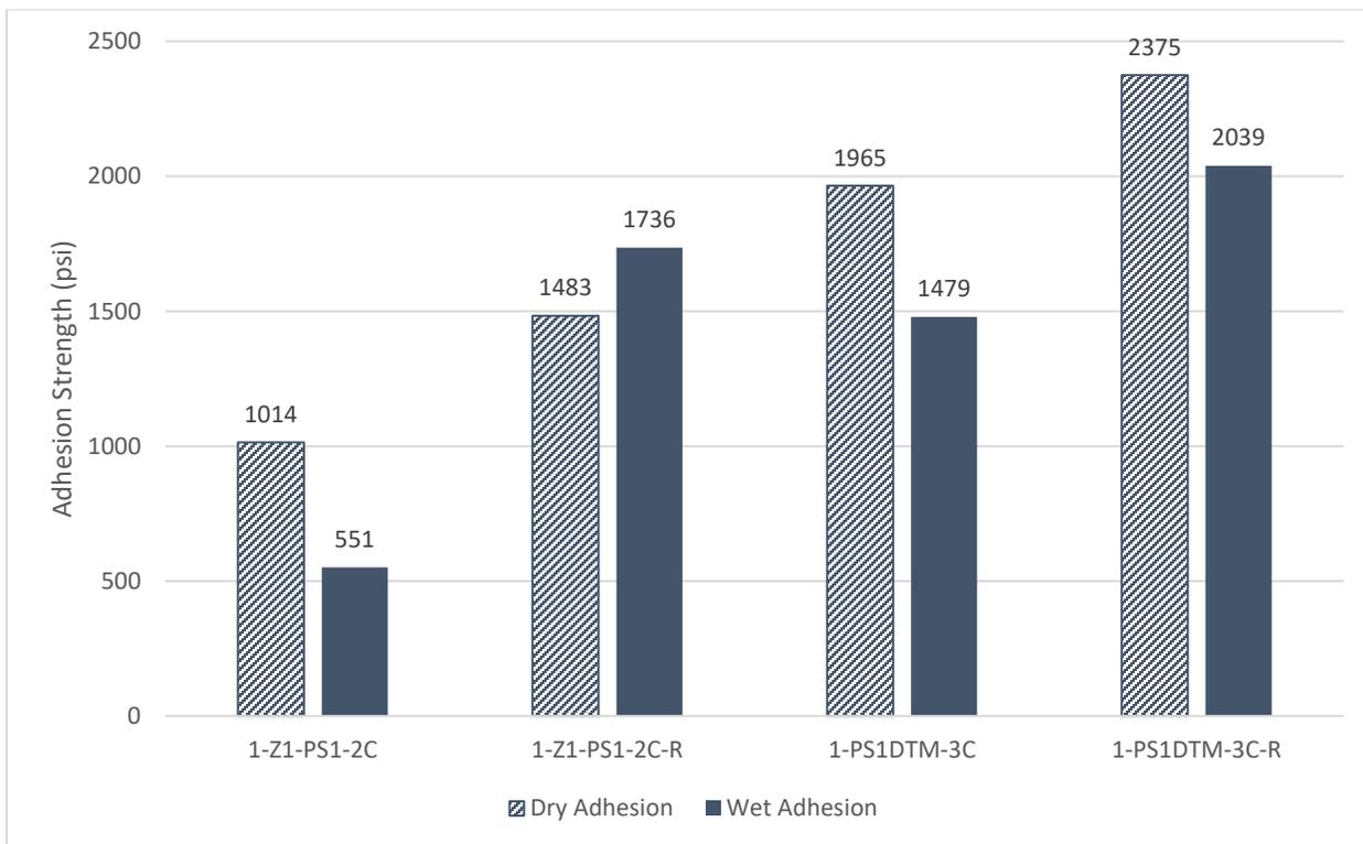
Figure 23: Dry and wet pull-off adhesion results for reproducibility study. Adhesion pull-off values increased for both systems.
