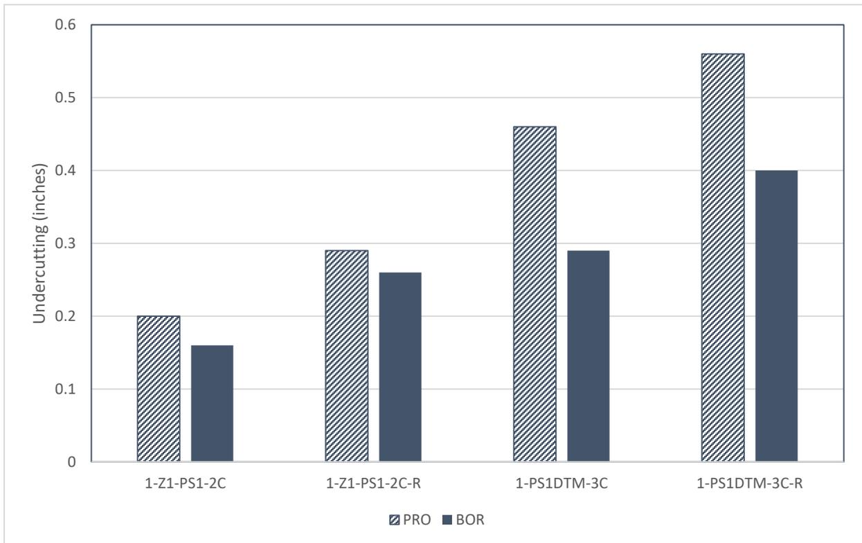
Figure 21: Cyclic test results for PRO and BOR test reproducibility study. Undercutting resistance decreased for both coating systems and both tests.
