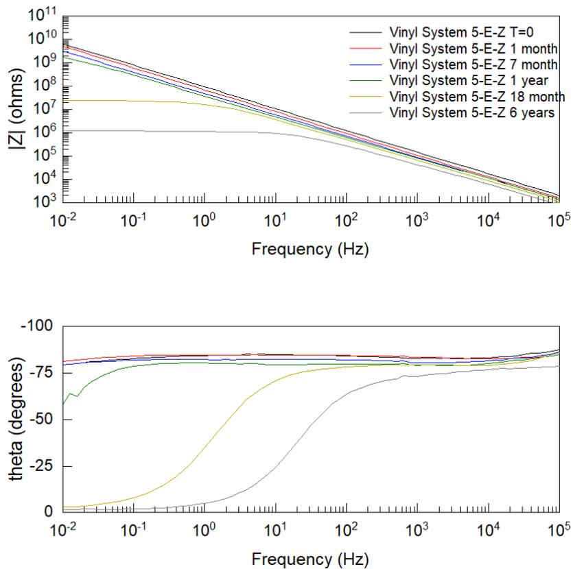
Figure 2. EIS data presented as Bode plot for vinyl system 5-E-Z, exposure time is 6 years. The impedance magnitude and phase angle decreased during immersion testing.
