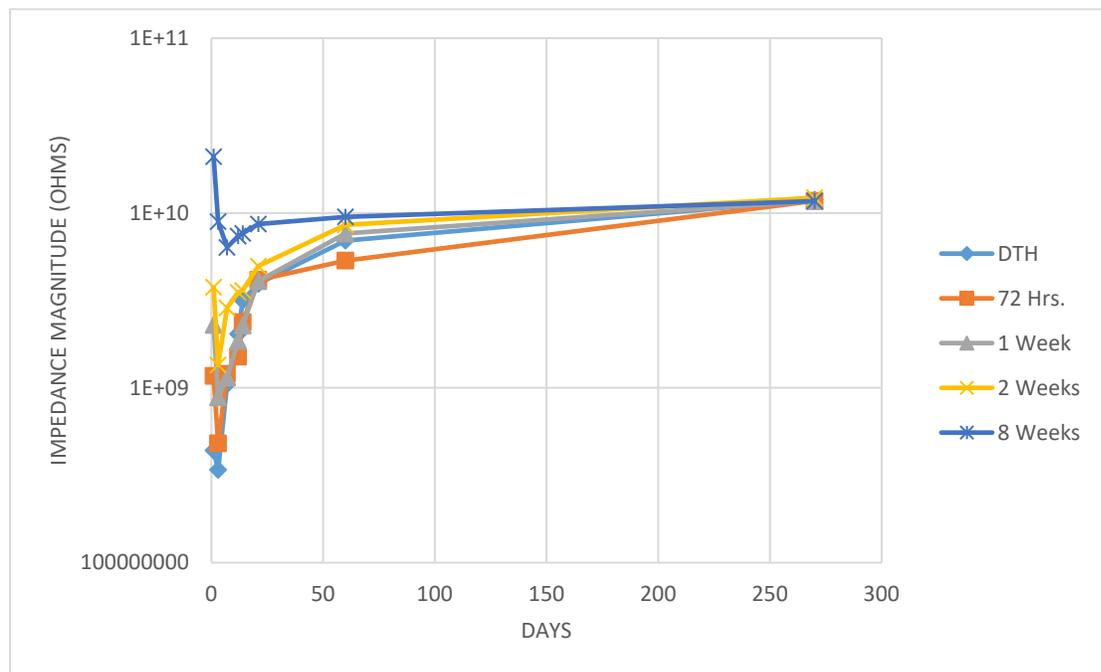
Figure 29: Impedance magnitude at low frequency over the duration of testing. The cure durations have different starting impedance values but all level out to the same impedance value at approximately 250 days.
