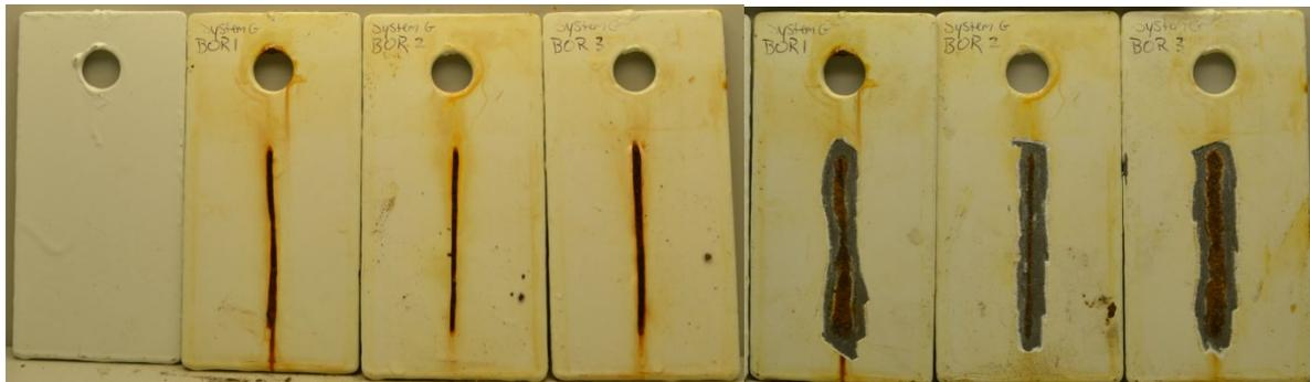
Figure 14. BOR cyclic test of 2-Z1-PS2; (left) before scraping (right) after scraping away coating.
