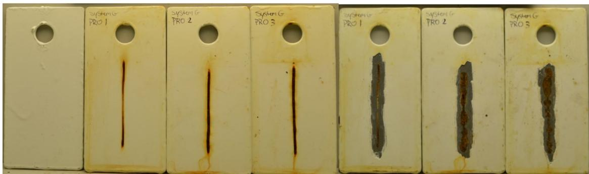
Figure 15. PRO cyclic test of 2-Z1-PS2; (left) before scraping (right) after scraping away coating.
