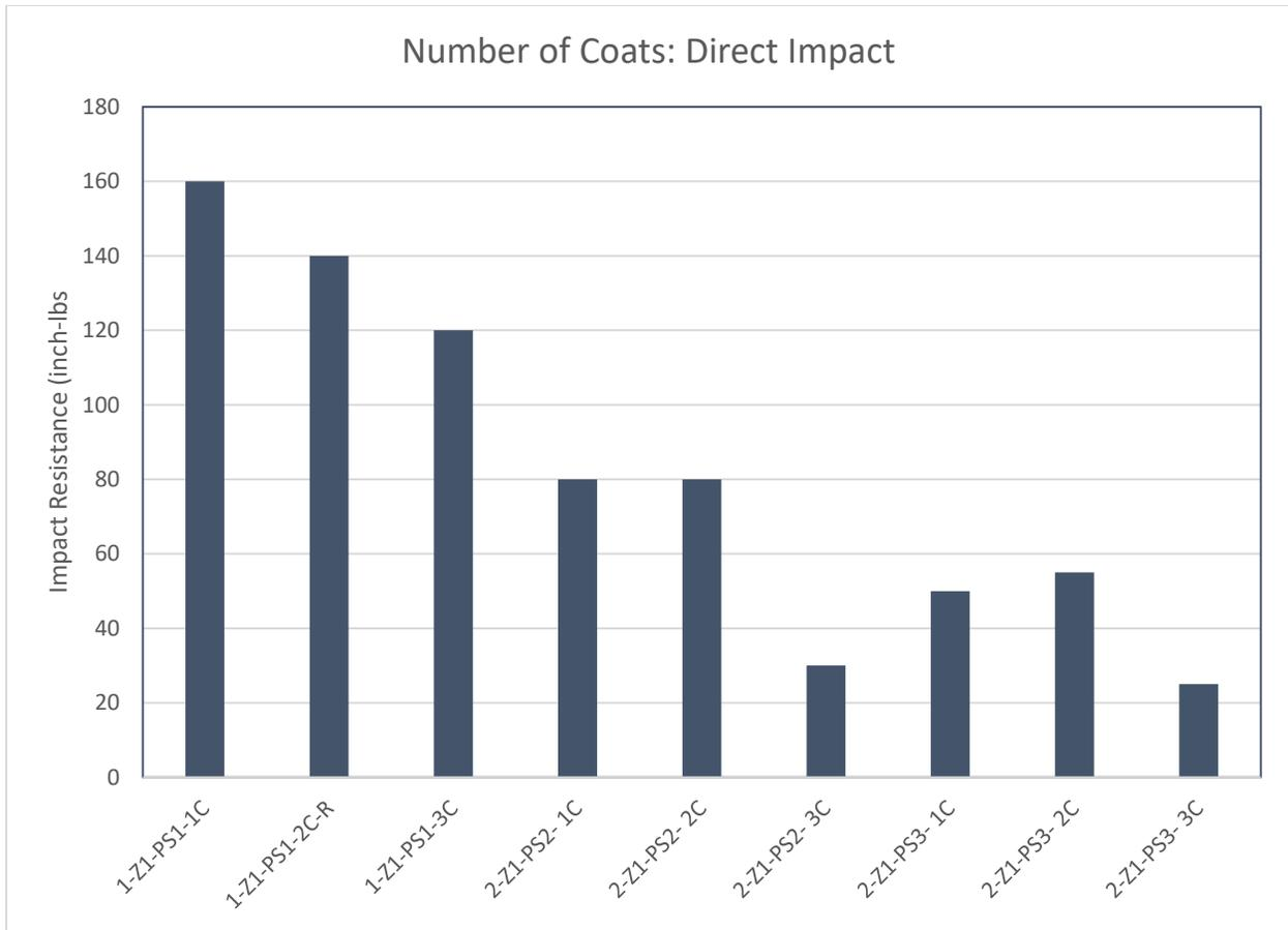
Figure 27: Direct impact results. Manufacturer 1 had higher impact resistance than Manufacturer 2. As the number of coats increased the impact resistance decreased.
