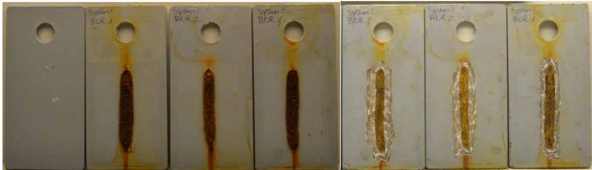
Figure 13. BOR cyclic test of vinyl system 5-E-Z; (left) before scraping (right) after scraping away coating.
