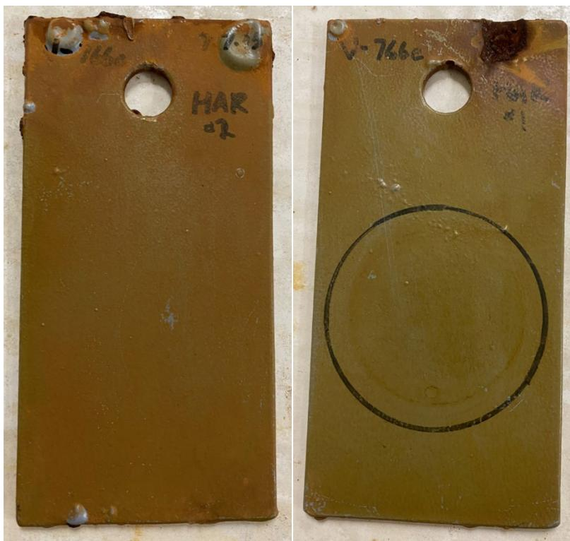
Figure 8. Vinyl System 4 after six years on immersion testing. Large blisters have formed around edges and small blisters formed near EIS test cell.
