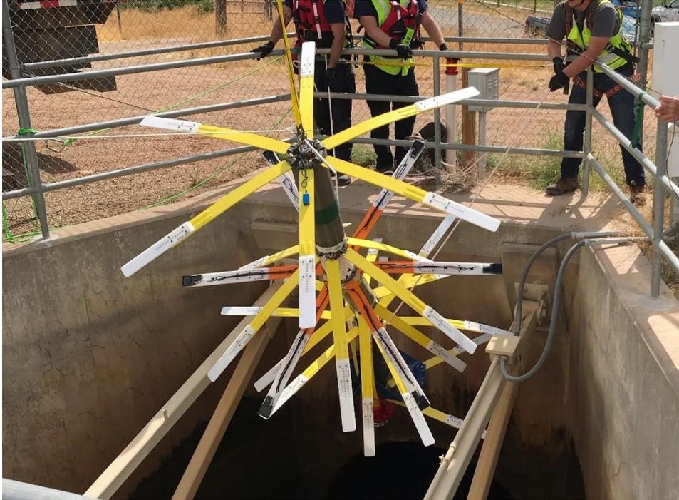
Figure 2-2. EM inspection tool being lowered into Dolores siphon for unmanned EM inspection
