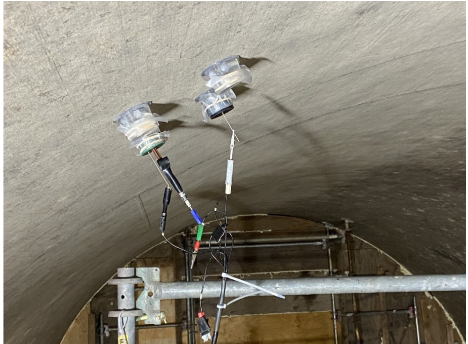
Figure 1. Electrochemical impedance spectroscopy test cell set-up for coating evaluation near pipe crown in a large diameter pipe.
