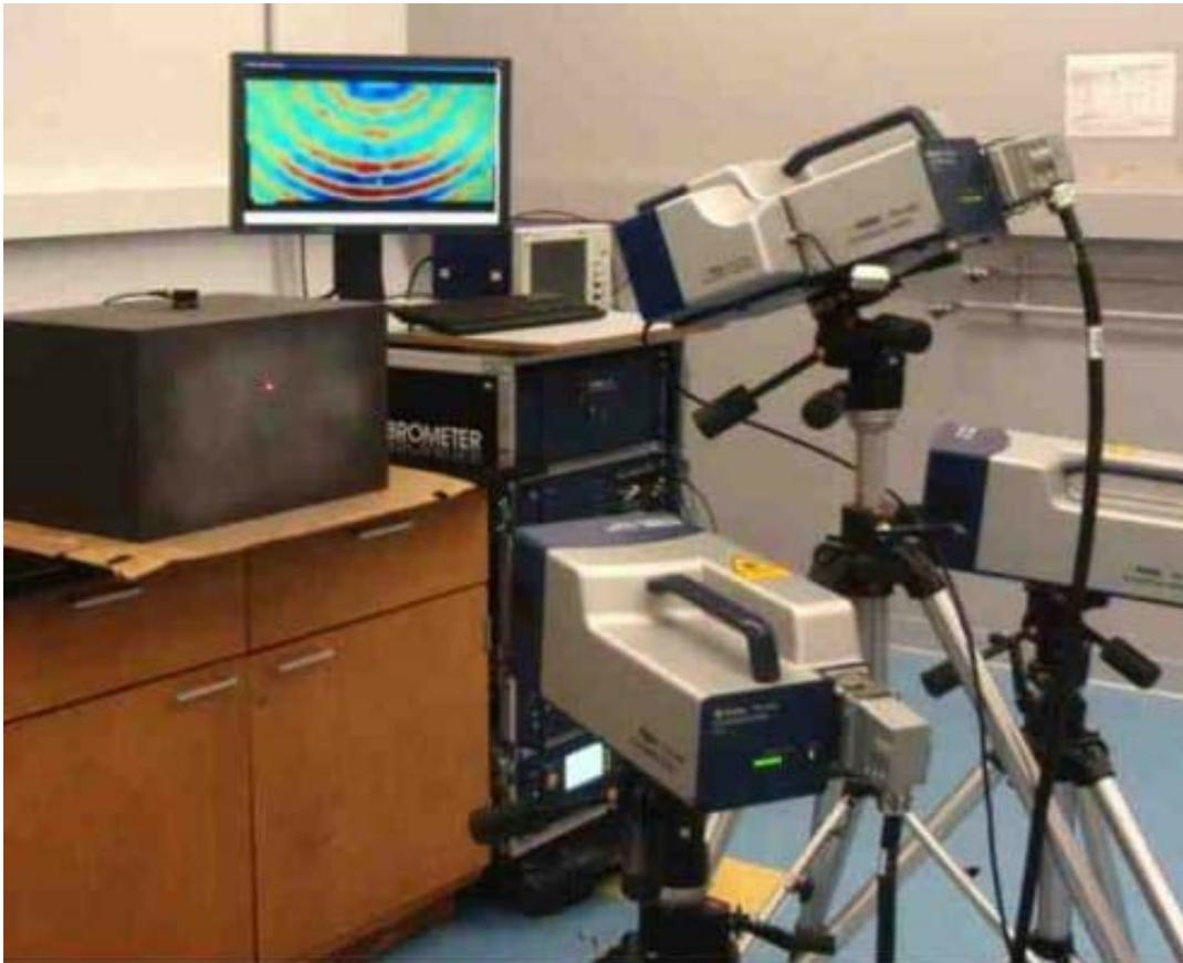
**Figure 2.** Image of an LDV lab experimental setup: Scan of a nuclear graphite block experiencing bulk and surface wave propagation. The wavefield simultaneously captured from the block surface by three LDV units placed at different angles is subsequently fed to an inverse-elasticity algorithm to reconstruct the position, size, and shape of defects (e.g. internal damage due to thermal gradients) that may have developed in the interior of the block, from (Pourahmadian & Guzina, 2018).
