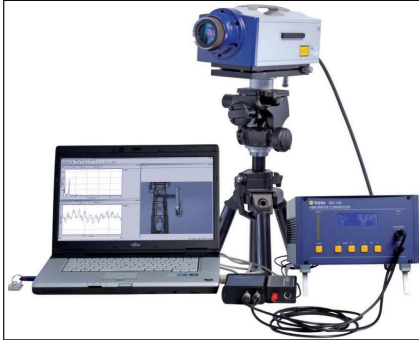
**Figure 11. Image of the PolyTec Inc. RSV-150M system with compact data acquisition system and simple USB computer interface. The image shows waveforms and spectral content of vibrations of a remote cell tower antenna several hundred feet away from the tripod-mounted sensor head, taken from (PolyTec, 2019).**
