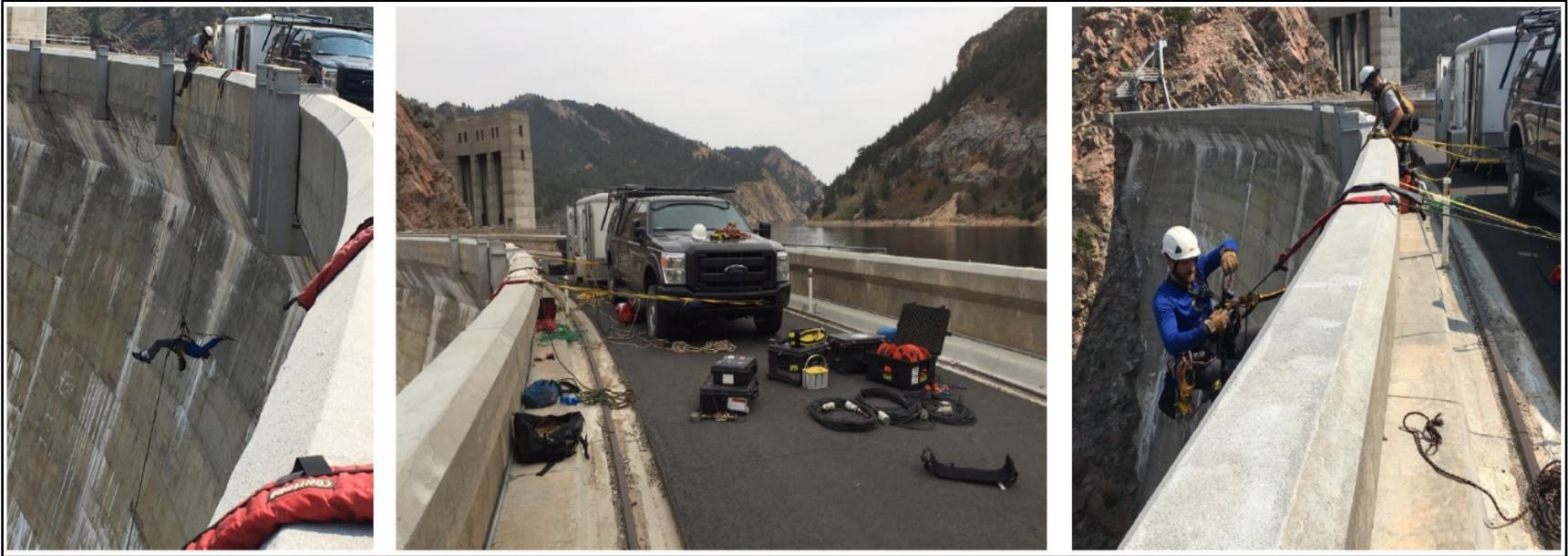
**Figure 3. Photos showing complex ropes access team preparations for seismic data collection along vertical transects on the downstream face of Seminoe Dam in Wyoming.**
