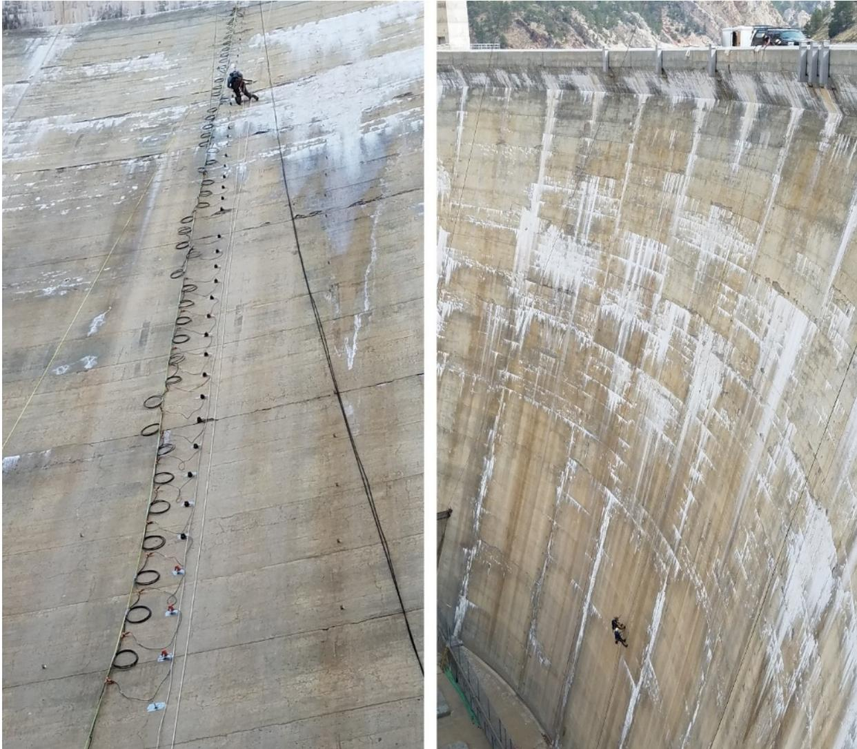
**Figure 15. Photos showing ropes access supported geophysical data collection along a vertical seismic survey transect mounted down the face of Seminole Dam in Wyoming. These data were collected as part of a research project related to ASR detection with the use of various geophysical techniques.**
