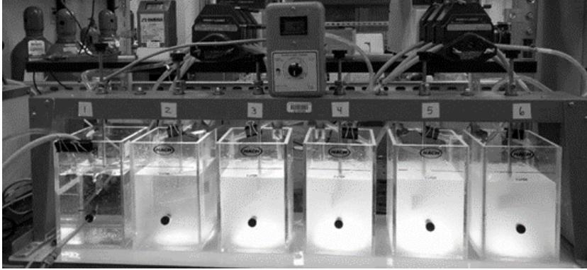
Figure 2. Six CSTRs-in-series running at steady state ( $\tau \sim 11$  min). Observe the increase in turbidity from left to right.
