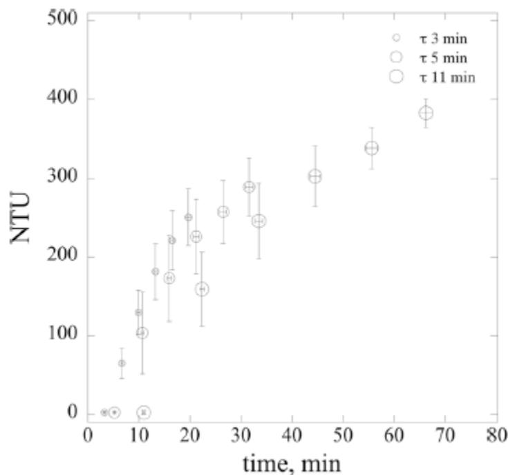
Figure 5. Turbidity (NTU) vs. reaction time (min). Each data point is a CSTR (nos. 1-6 left to right) for the particular residence time,  $\tau$ . The uncertainties are 1 standard deviation.
