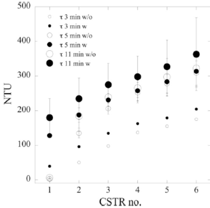
Figure 7. Turbidity vs CSTR no. without (w/o) and with (w) recirculation mixing (380 mL/min) in the 1<sup>st</sup> CSTR at three residence times ( $\tau$ ). The uncertainties are 1 standard deviation (only one experiment was performed at  $\tau \sim 3$  min).
