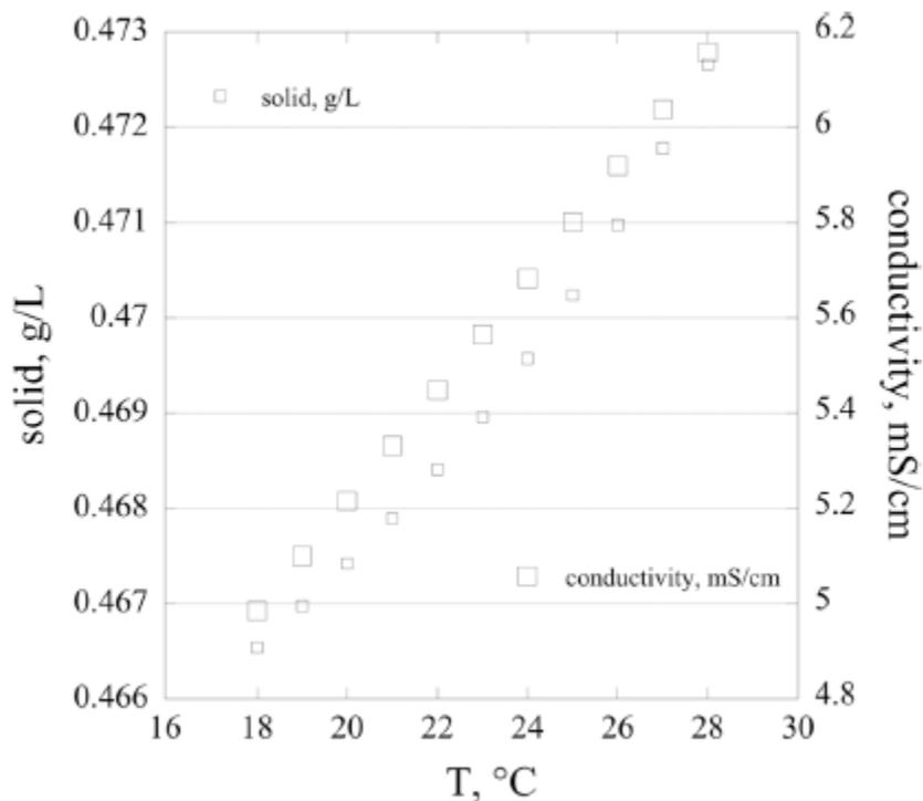
Figure 3. Estimated calcite precipitated and solution specific conductivity at equilibrium for the mixed composition from Table 4.
