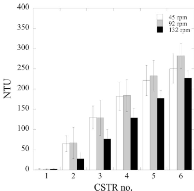
Figure 6. Effect of impeller speeds on turbidity evolution ( $\tau \sim 3$  min).
