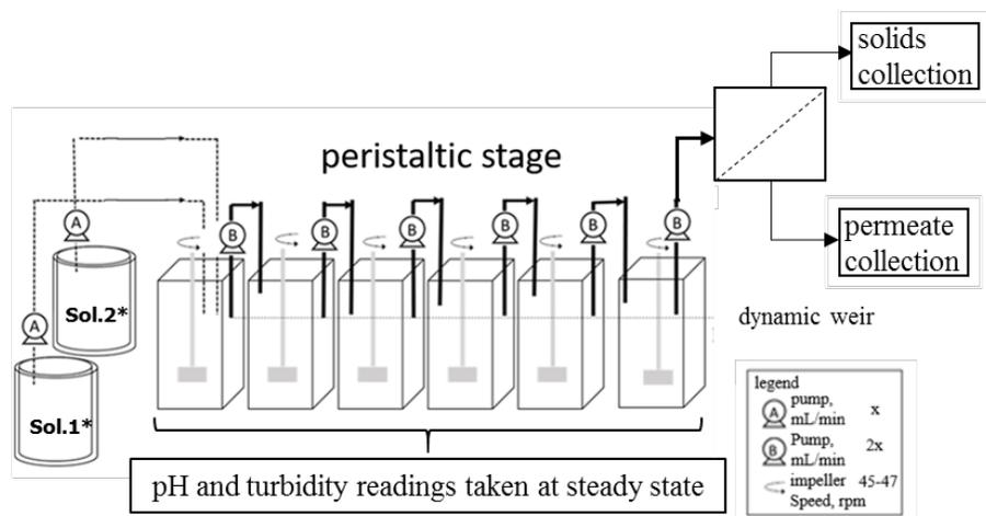
Figure 1. Schematic representation of CSTRs-in-series setup.
