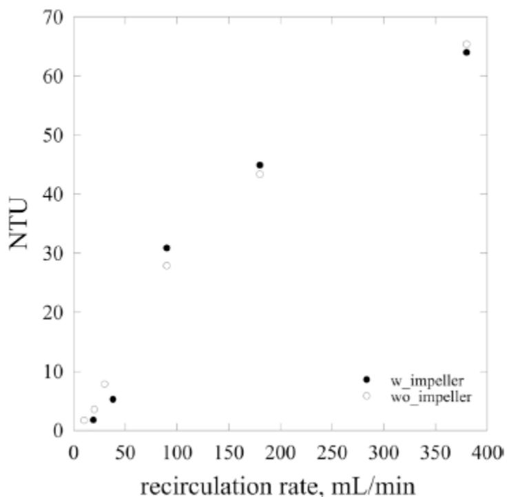
Figure 9. Turbidity in one CSTR using peristaltic-pump-based recirculation mixing with and without additional impeller mixing (@  $\sim 45$  rpm) with  $\tau \sim 3$  min.
