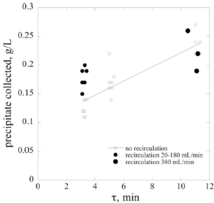
Figure 8.  $\text{CaCO}_3$  precipitate collected from 6<sup>th</sup> CSTR vs. residence time with and without recirculation mixing in the 1<sup>st</sup> CSTR. Trendline presented for the impeller mixing-only data.
