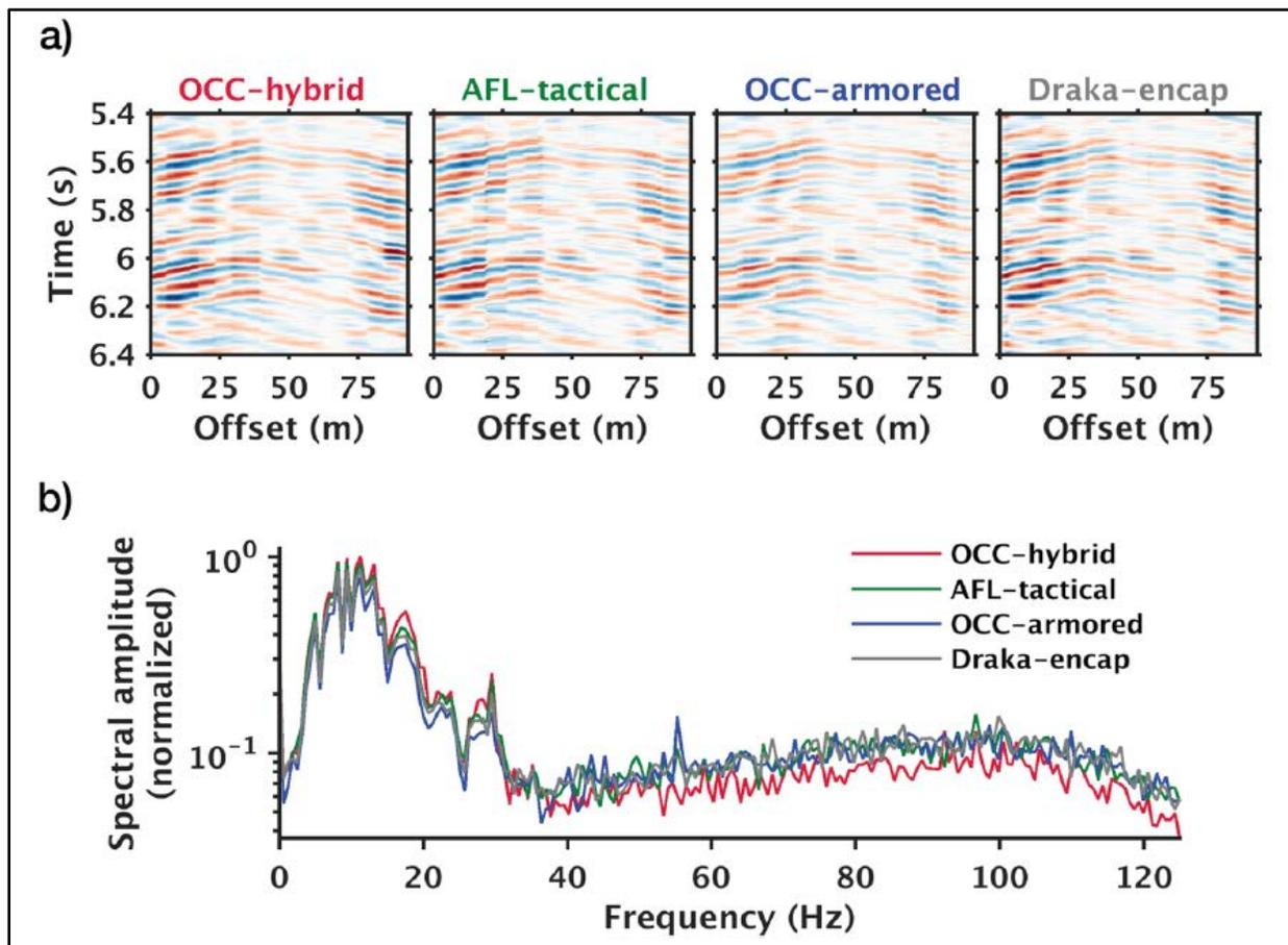
Figure 6 – Comparisons of identical traffic noise recorded by fiber-optic cables of different packaging. (a) Zoom-in view of 1-second noise records. (b) Mean spectral amplitudes computed using identical spatial and temporal windows (spatial window = offset range as in (a); temporal window = 1 minute). From Dou et al. (2017).
