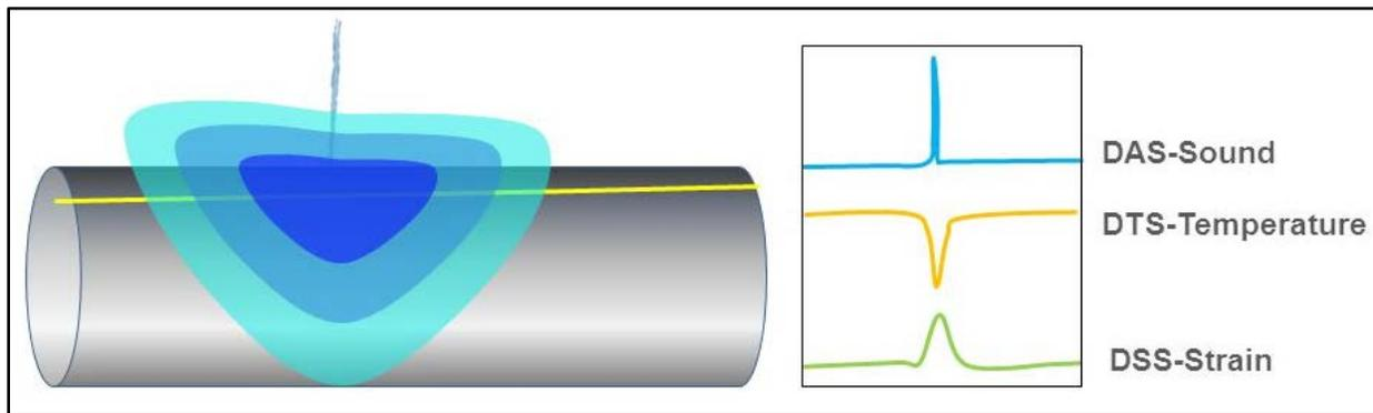
Figure 17 – Schematic of pipeline leak detection using DAS, DTS, and DSS technology. Modified from Hawk Measurement Systems (2020).
