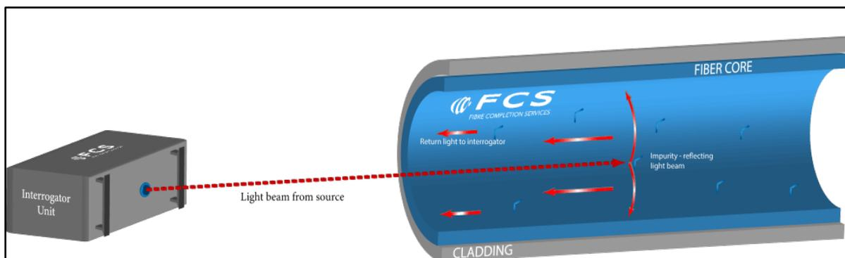
Figure 1 – Schematic of a DAS system’s main components: an interrogator unit and a fiber optic cable. Modified from FCS (2020).
