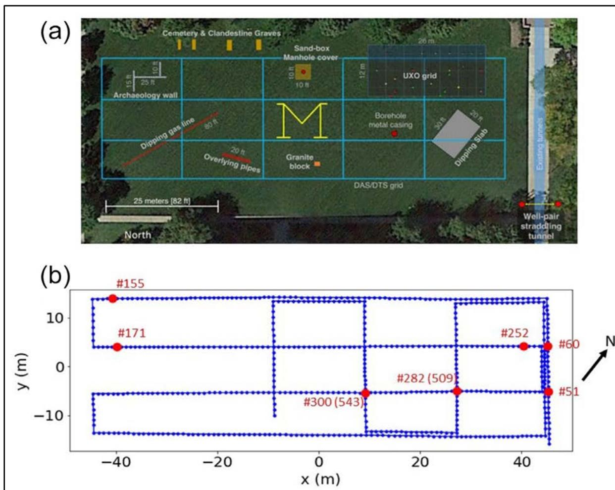
Figure 23 - Map of Kafadar Geophysical Laboratory buried anomalies, including the 27 m by 90 m DAS (blue) grid. (b) DAS fiber-optic cable (blue curve) geometry and calibrated channel locations (blue dots). Red dots mark the channels mentioned in this paper. Modified from Luo, B., et al., (2020).
