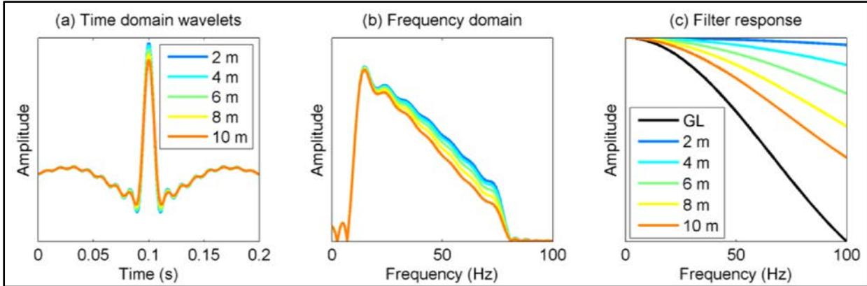
Figure 8 - Examples of Klauder wavelets (8 to 80 Hz) travelling at 2,000 m/s for a gauge length of 20 m. Modified from Dean and Hartog (2016).
