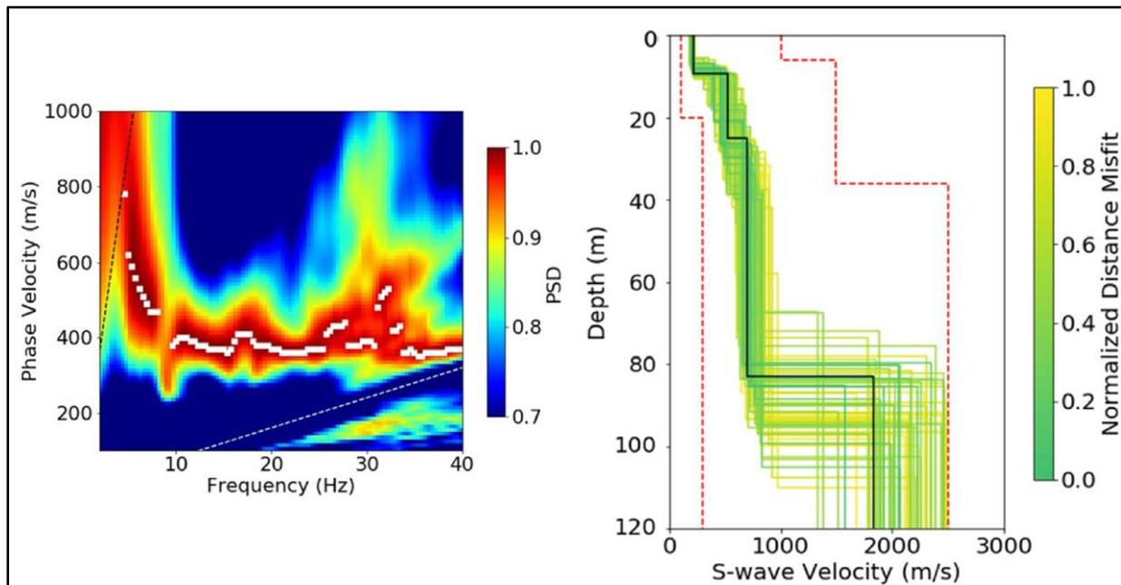
Figure 21 – Dispersion image of a 5-min chunk of passive seismic data and the picks of dispersion data points depicted with white squares (left). The accepted final MASW modeled S-wave velocity profiles color-coded by normalized distance misfit (right). Black solid curves denote the best-fitting model with least distance misfit. Red dashed curves mark the model parameter boundaries for inversion. Modified from Luo et al., (2020).
