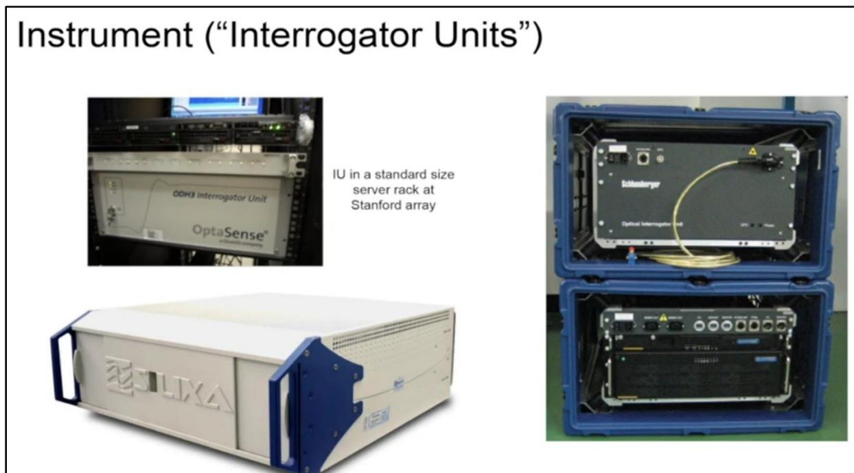
Figure 2 – Example photos of DAS Interrogator units, generally described as small semi-portable or rack-mounted electronic systems that are connected at one end of a fiber optic cable. Modified from Dou et al., (2017).
