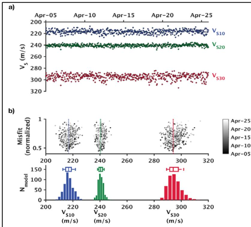
Figure 20 - Average shear-wave velocities ( $V_{s10}$ ,  $V_{s20}$ , and  $V_{s30}$ ) estimated from best-fit models of all 502 epochs. (a) Average  $V_s$  displayed as functions of calendar time. (b) Distributions of  $V_{s10}$ ,  $V_{s20}$ , and  $V_{s30}$  (lower) and corresponding misfits (upper) ( Dou et al., 2017).
