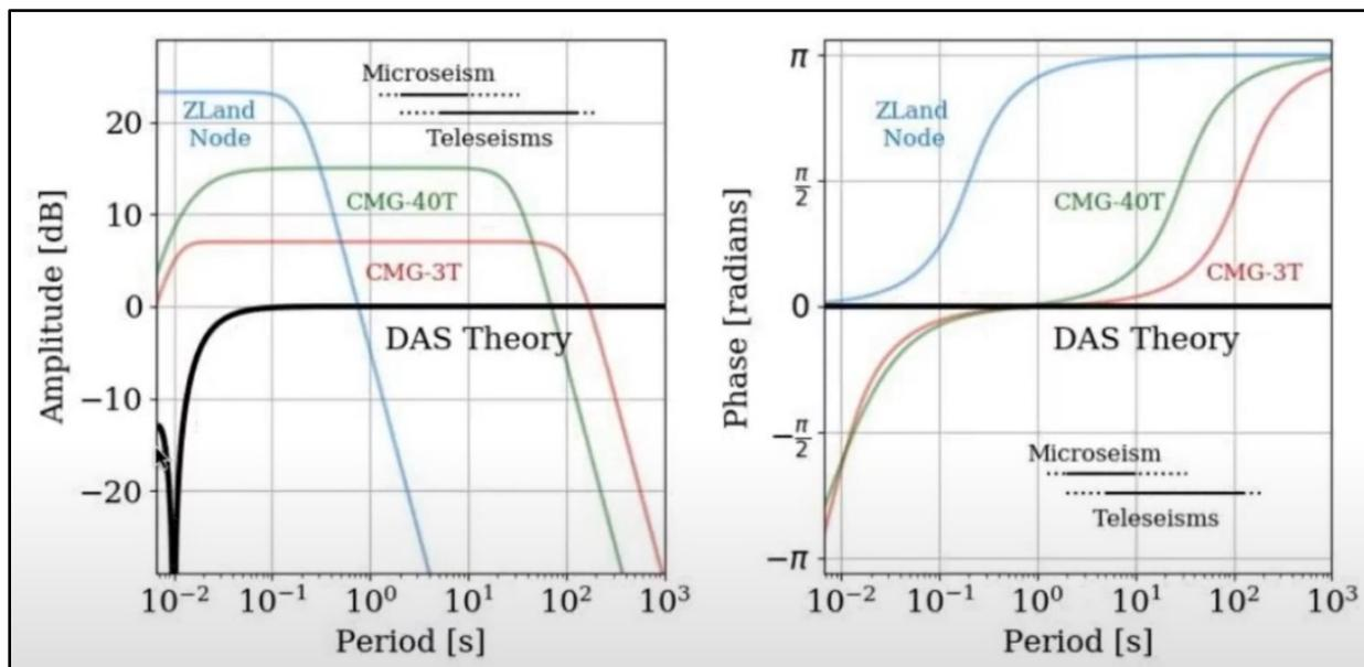
Figure 10 - Graphic depicting the instrument responses of various broadband seismometer instruments (labeled colored lines) and typical DAS systems (bold black line) with amplitude and phase spectra presented in left and right plots, respectively. Modified from Lindsey, N., (2020).
