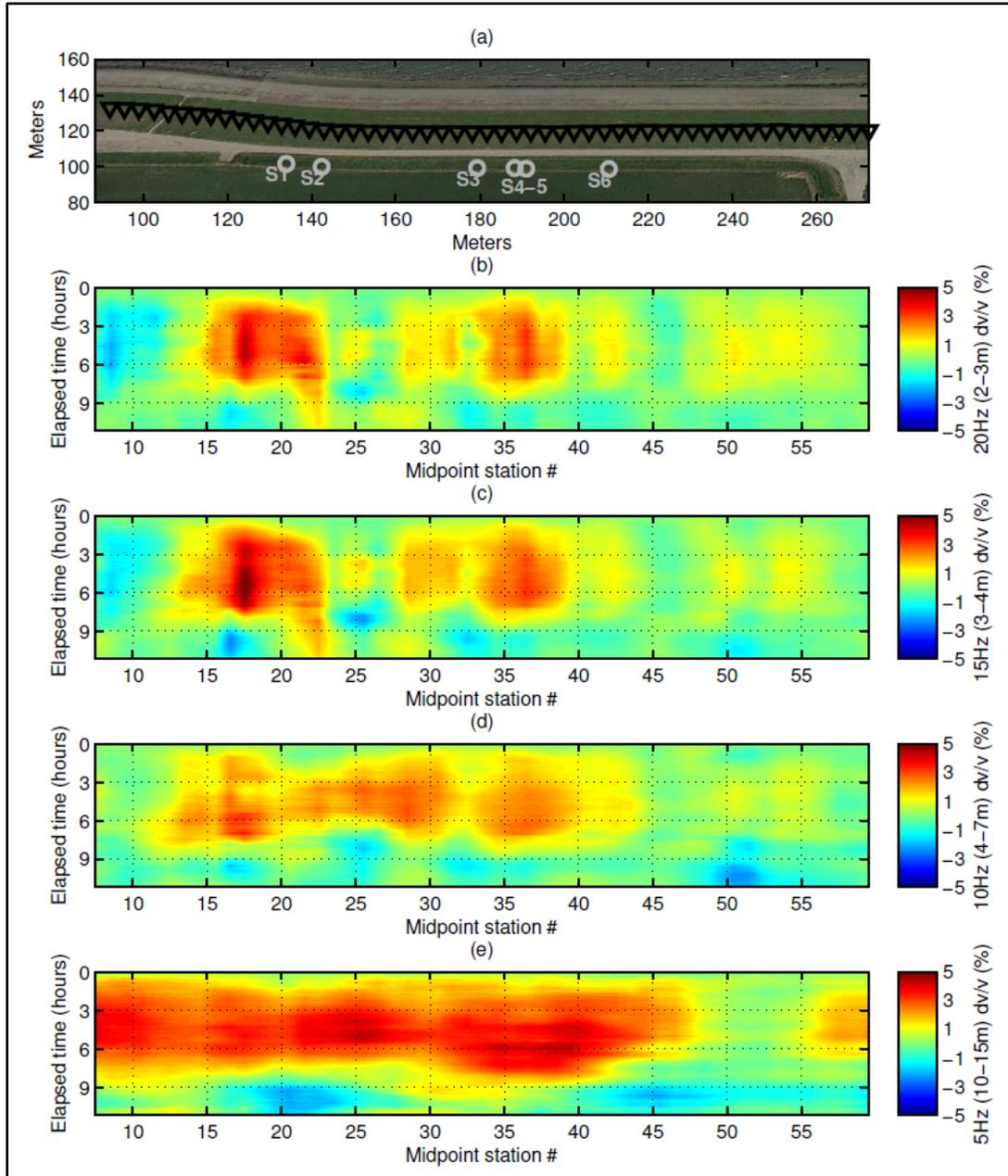
Figure 22 - Maps of relative velocity changes during the 12h tide cycle, along a 180m-long section of the levee. Different frequencies - i.e. depths - are investigated: 20Hz/2-3m (b), 15Hz/3-4m (c), 10Hz/4-7m (d), 5Hz/10-15m (e). A plan view of the monitored section aligned with the velocity variation maps is shown in (a). Note the spatial correlation between lateral locations of sand-boils and peak  $dV/V$  changes shown in red (Planès et al., 2017).
