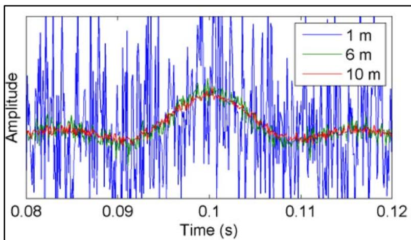
Figure 7 - Three synthetic Klauder wavelets (8 to 80 Hz) calculated using a gauge length of 20 m, a velocity of 2,000 m/s, and pulse widths of 1, 6, and 10 m. Modified from Dean and Hartog (2016).
