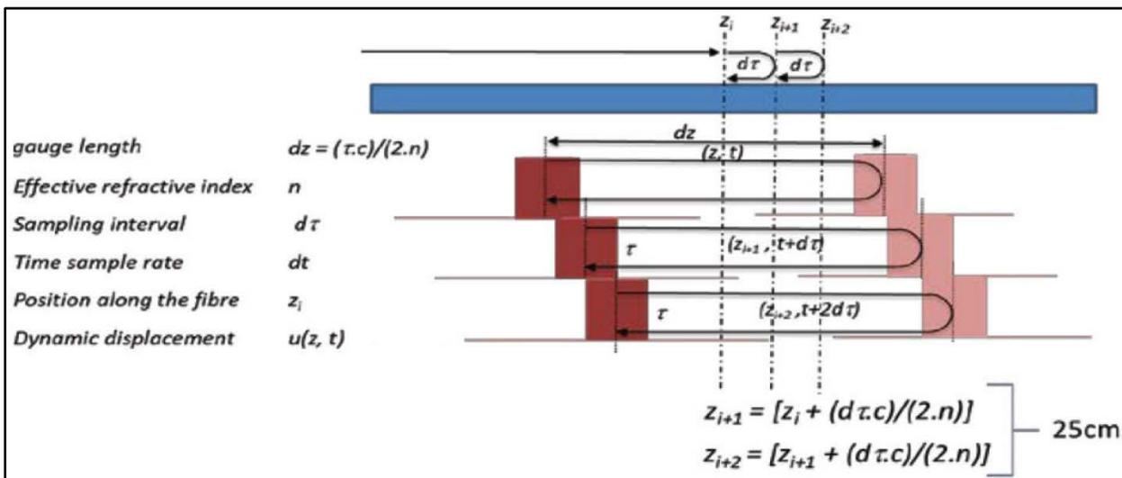
Figure 9 - Illustration of the measurement principles as well as the gauge length along a fiber. Modified from Naldrett et al., (2018).
