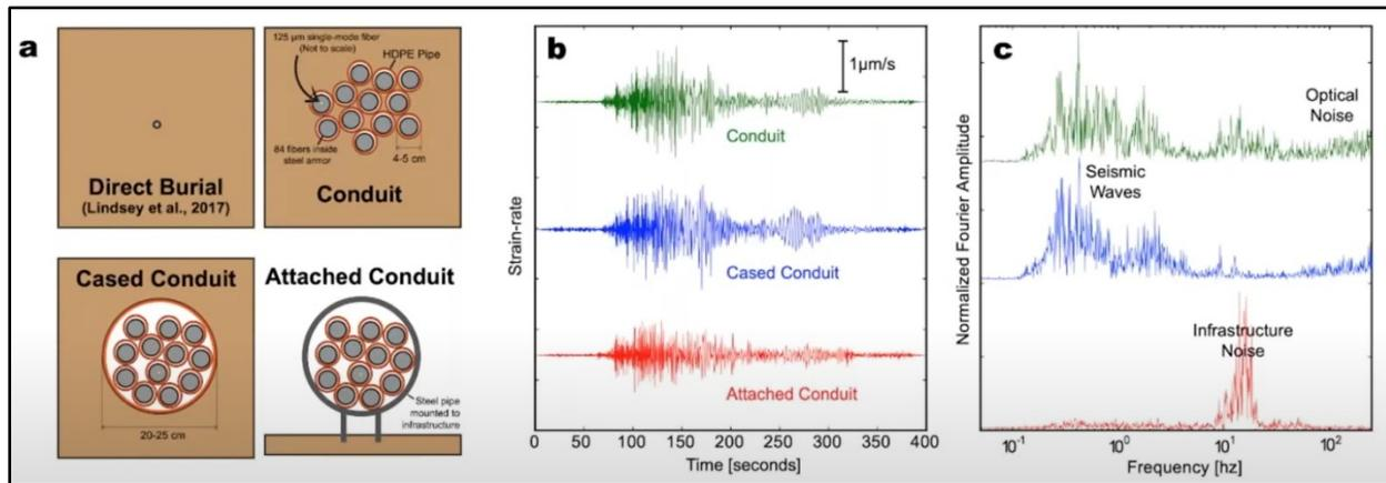
Figure 5 – Graphic depicting various options for installation and mounting (e.g., coupling) of DAS system fiber cables (a), and comparisons of the resulting data in the time-domain (b), and related amplitude spectra (c). As seen, each approach to mounting or installing DAS fiber affects the resulting recorded data characteristics, where the amplitudes of low-frequency modes are mostly affected. (Modified from Lindsey, N., 2020)
