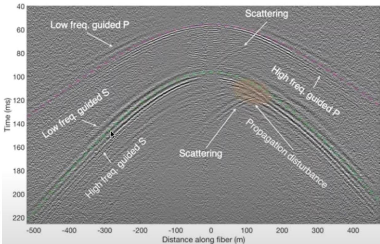
Figure 14 – Example of real seismic data collected along a single DAS fiber with sensing intervals of approximately 1m (3.28ft) along a 1000m long fiber (Lellouch et al., 2019).
