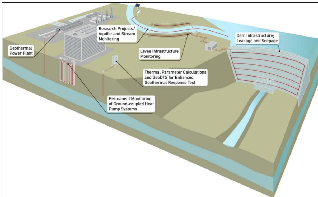
Figure 16 – Schematic of various applications of DAS (and DTS and DSS) already being implemented in industry. Modified from AP Sensing (2020).
