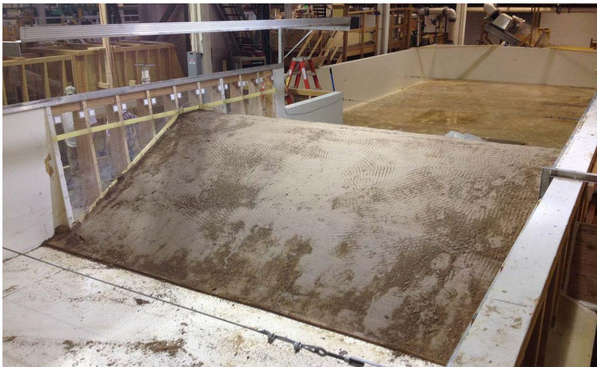
Figure 24 - Embankment breach test facility viewed from the upstream end of the headbox, overlooking the completed test embankment.
