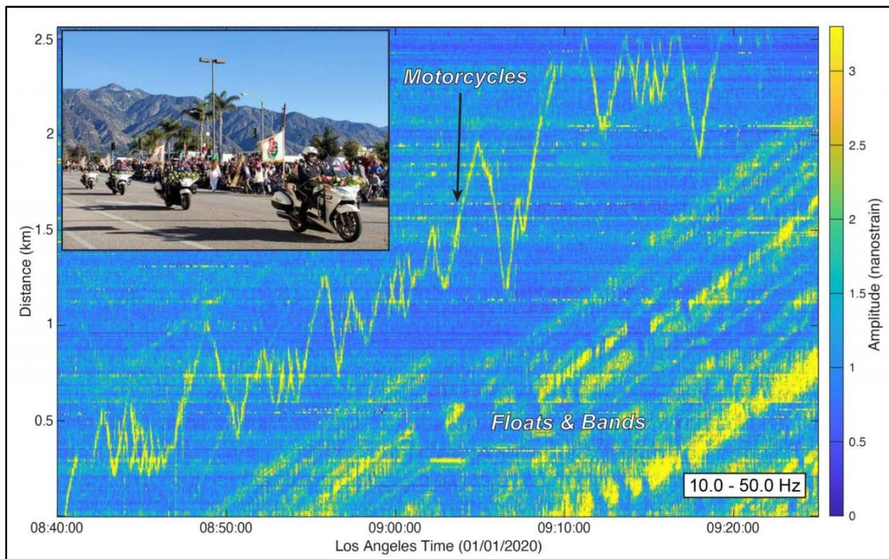
Figure 18 – DAS records showing seismic vibrations caused by motorcycles, marching bands, and floats during 2020 Rose Parade. Modified from SRL (2020).
