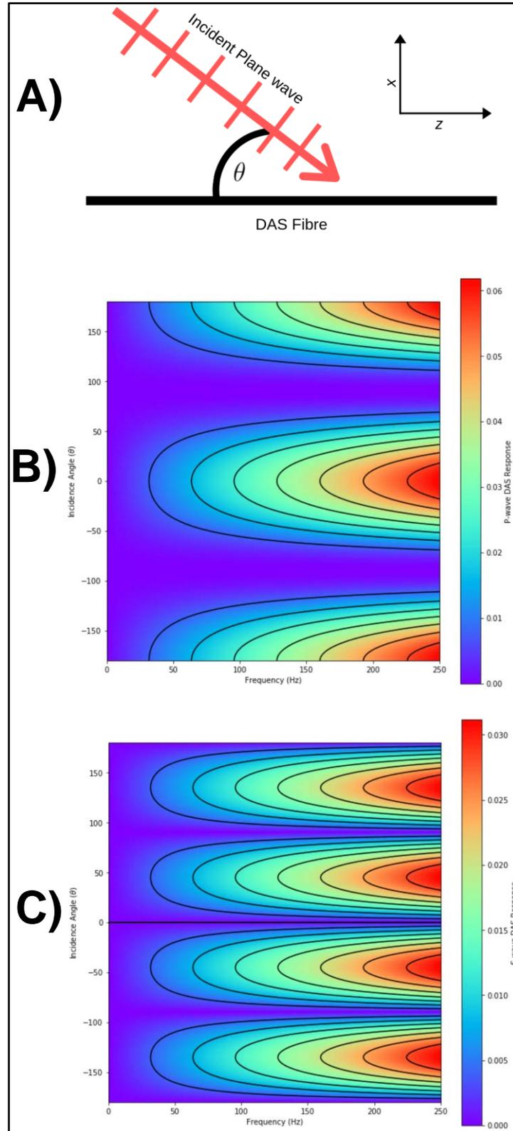
Figure 11 – Schematic of the angle of an incident plane-wave relative to a DAS fiber's normal vector (A), the amplitude response spectrum of DAS as a function of frequency and incidence angle for p-waves (B), and for s-waves (C). Modified from Chambers, K. (2020).
