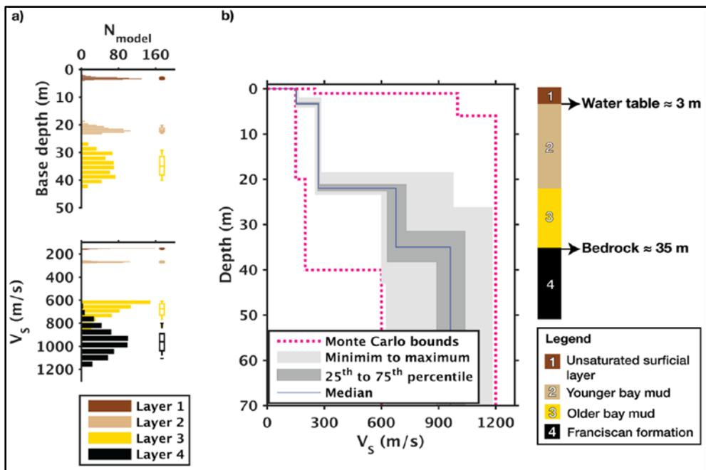
Figure 19 - Error analysis and geologic interpretation of the best-fit  $V_s$  profiles. (a) Histogram and box plots illustrating distributions of base depth and  $V_s$  in each layer. (b) Error bounds, median  $V_s$  profile, and corresponding geologic features ( Dou et al., 2017).
