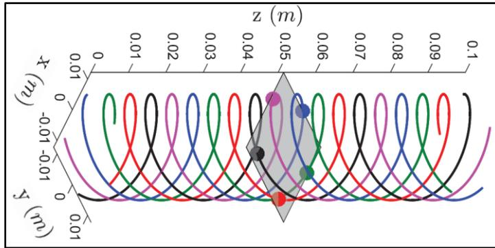
Figure 15 - Example of five equally spaced helical optical fibers with a diameter of 2.44 cm and a pitch angle of  $20^\circ$ . The dots represent measurement at the same length along respective fibers, which refer to the same portion of the cable indicated by the horizontal plane. Modified from Ning and Sava (2018).
