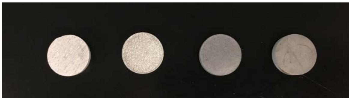
Figure 1: 316L stainless steel specimens. From left: cold rolled steel, as-printed PBF printed steel, heat treated PBF printed steel, and PBF printed steel after sensitization and etching.
