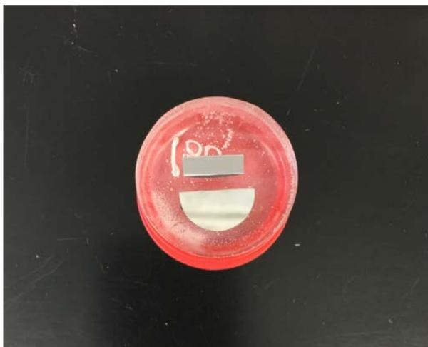
Figure 3: Metallography specimen (as-printed) mounted in epoxy and polished to one micron.
