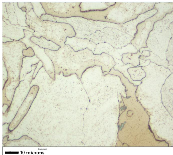
Figure 12: Microstructure of the heat-treated specimen at a magnification of 63X.
